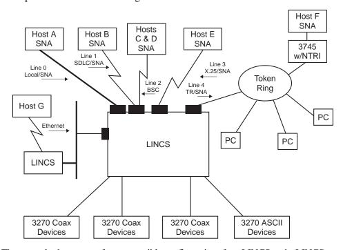
The example shows one of many possible configurations for a LINCS node. LINCS can support up to 16 hosts (Hosts A through P) on eight lines (Lines 0 through 7). Figure 2-3 shows the following support:
