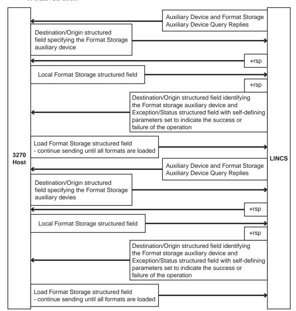
The following diagram shows the typical sequence of events when a host is distributing formats to a LINCS node.
