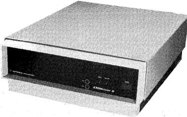
The EXORciser is an expandable development system that allows development of any 8-bit Motorola microprocessor or microcomputer configuration, from the simplest to the most elaborate. It comes with an MPU Module that provides system timing and a DEbug Module that contains system firmware. Both MC68B00 or MC68B09 MPU versions are offered in the EXORciser Development System.
