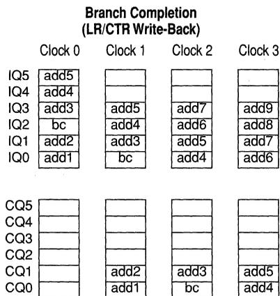
**Figure 6-9. Branch Completion**
