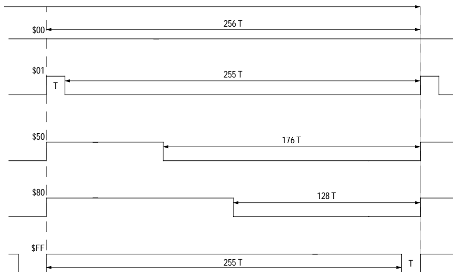
Figure 12-2 PWM output waveforms (POL = 1, active high)
