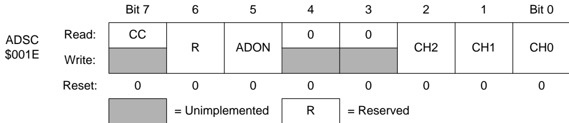
Figure 9-1. A/D Status and Control Register
