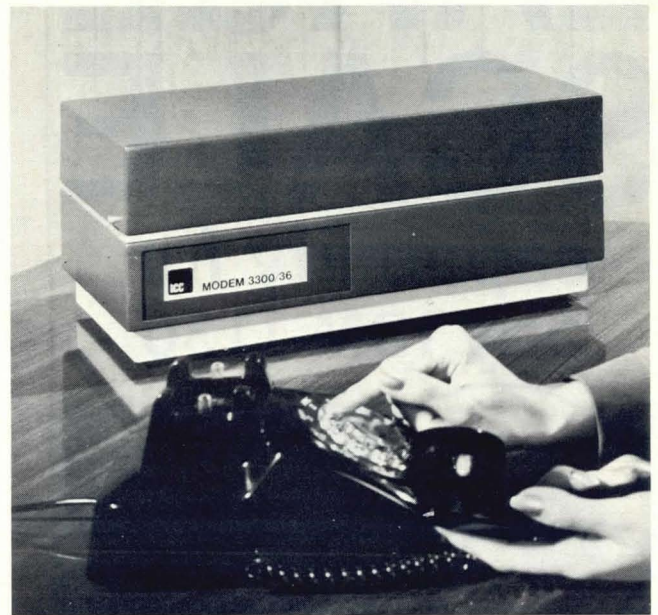
Fig. 4 Typical hardwired modem. (International Communications Corp.'s Model 3300/36)
