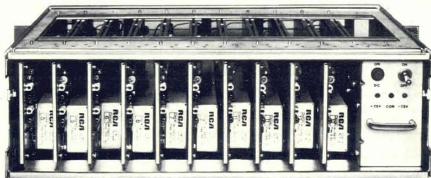
Fig. 5 Typical multiplexer for point-to-point lines. (RCA's Model CDM)
