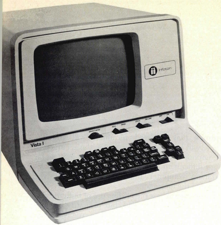
Fig. 1 Typical CRT display terminal. (Infoton VISTA 1)
