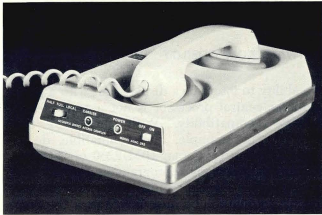
Fig. 3 Typical acoustic coupler. (Anderson Jacobson ADAC 242)
