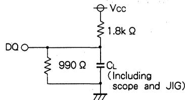
Fig.1 Output load
