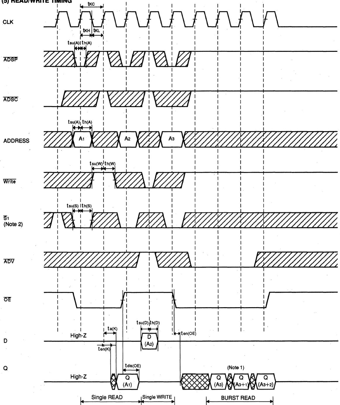
Note 1. Q(A3) refers to output from address A3. Q(A3+1) refers to output from the next internal burst address following A3.
