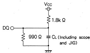
Fig. 1 Output load
