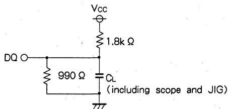
Fig.1 Output load
