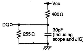
Fig.1 Output load
