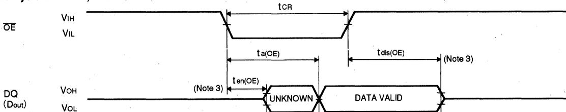
Note 4. Address and  $\bar{S}$  valid prior to  $\overline{OE}$  transition low by  $(t_{a(A)} - t_{a(OE)})$ ,  $(t_{a(S)} - t_{a(OE)})$ .
