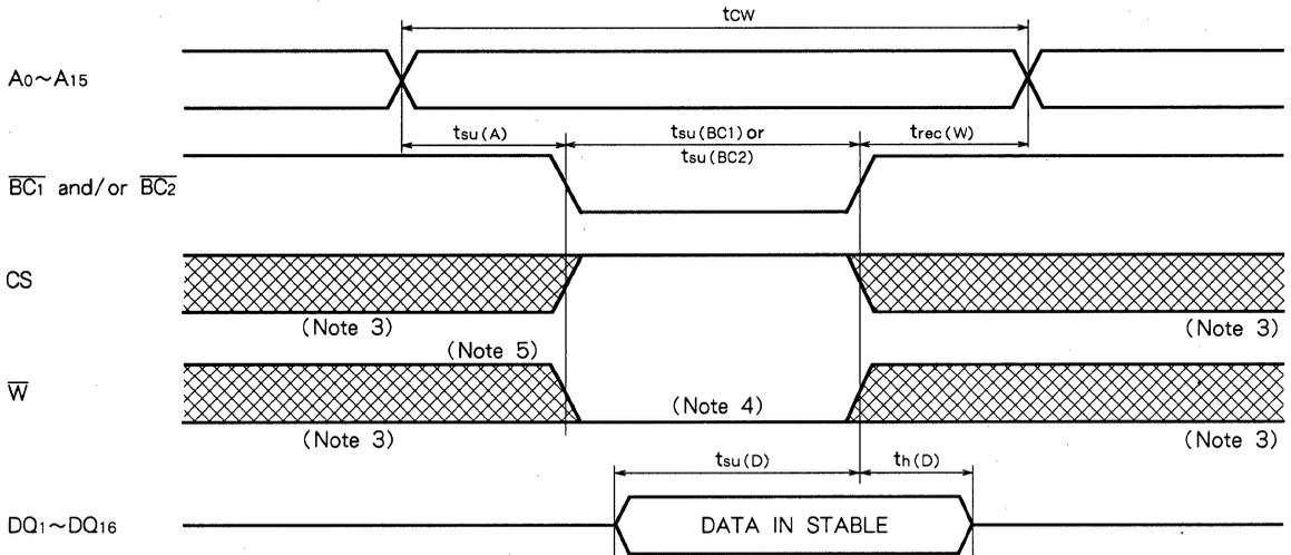
Write cycle ( $\overline{CS}$  control mode)
