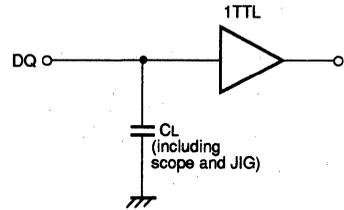
Fig.1 Output load
