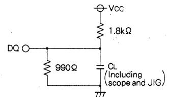
Fig. 1 Output load
