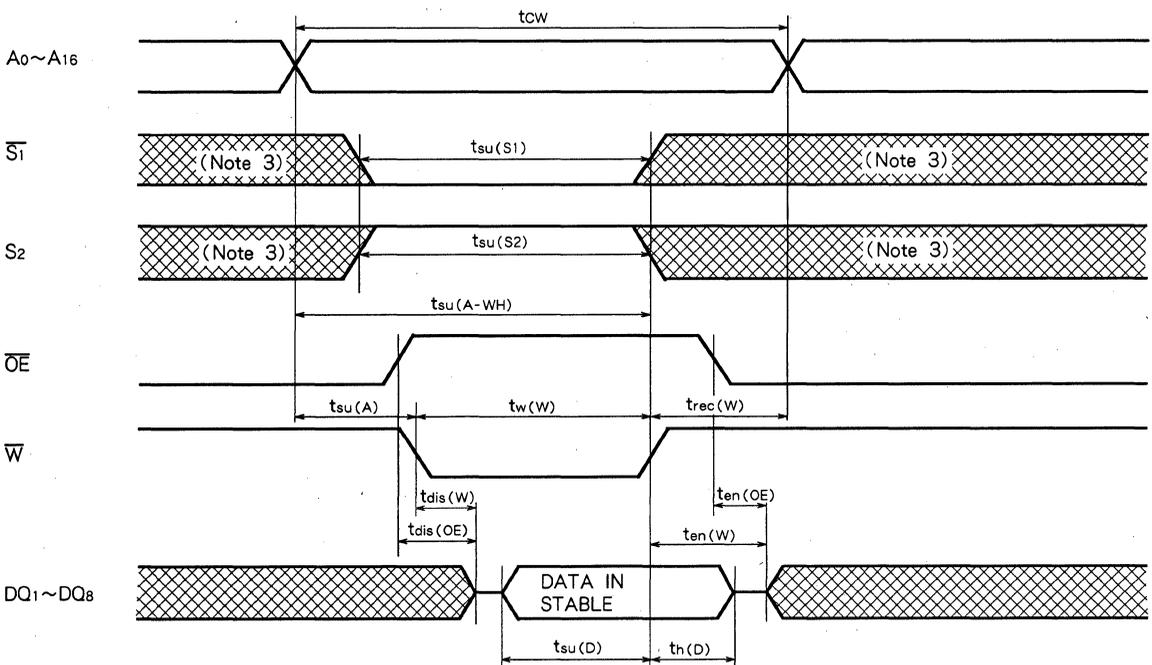
Write cycle ( $\overline{S1}$  control mode)
