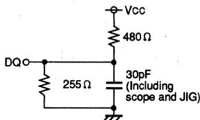
Fig.1 Output load
