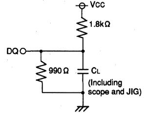
Fig.1 Output load
