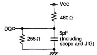
Fig.2 Output load for t<sub>en</sub>, t<sub>dis</sub>
