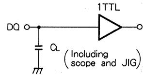
Fig.1 Output load
