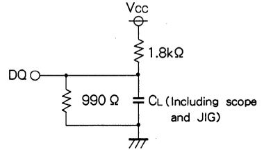
Fig. 1 Output load
