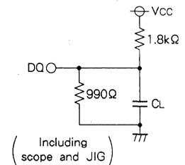
Fig. 1 Output load
