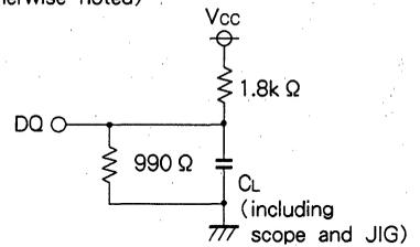
Fig.1 Output load
