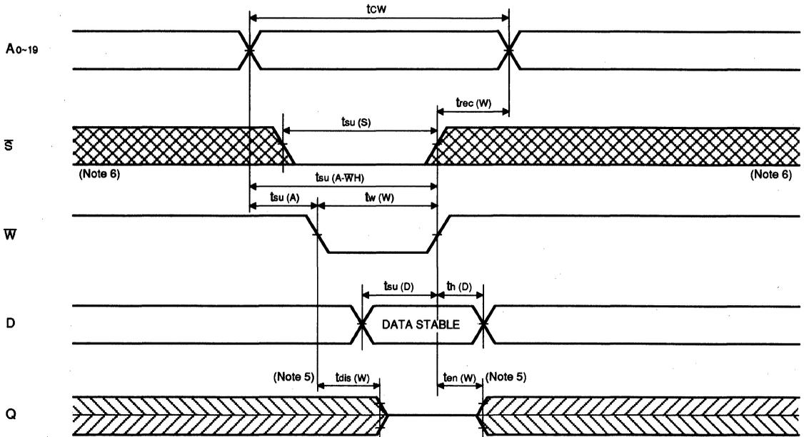
**Write cycle ( $\overline{S}$  control mode)**
