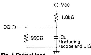
**Fig. 1 Output load**
