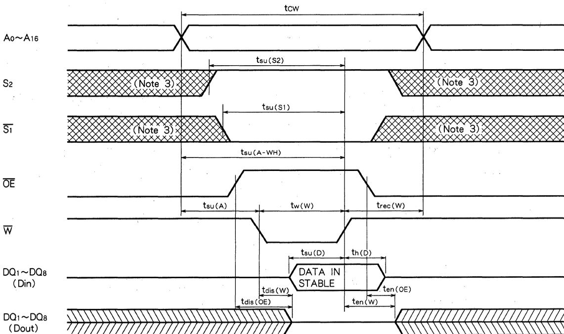
Write cycle ( $\overline{S1}$  control mode)
