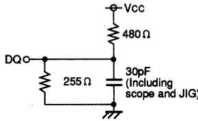
Fig.1 Output load
