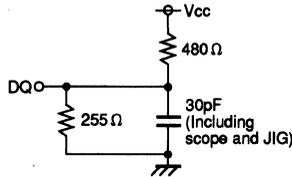
Fig.1 Output load
