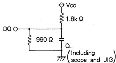
Fig. 1 Output load
