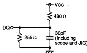
Fig.1 Output load
