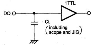
Fig.1 Output load
