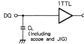
Fig.1 Output load
