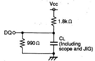
Fig.1 Output load
