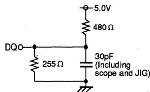
Fig.1 Output load
