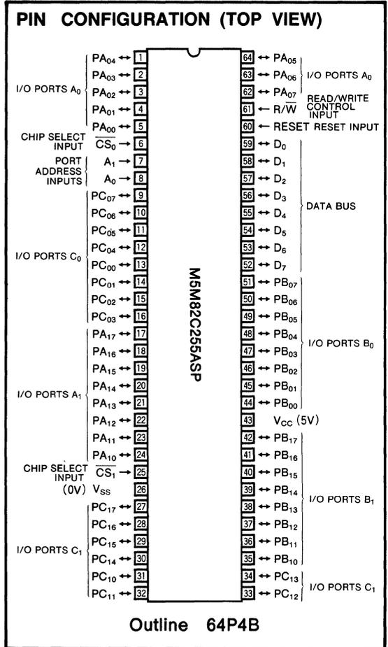
**CMOS PROGRAMMABLE PERIPHERAL INTERFACE**
