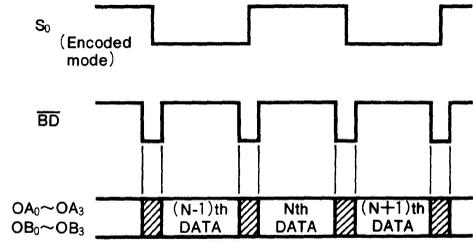
Note 5 : Values of the output data shown in the slanted line areas are decided upon the clear command executed last to become the value of the display RAM after the reset. The values in the slanted areas after reset will go low-level. In the same manner, the values  $OA_0 \sim OA_3, OB_0 \sim OB_3$  are dependent on the clear command executed last. When the both A and B are blanked, the signal  $\overline{BD}$  will be in low-level.
