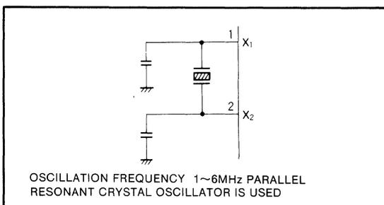
Fig. 7 Connections when crystal is used for X<sub>1</sub> and X<sub>2</sub> inputs
