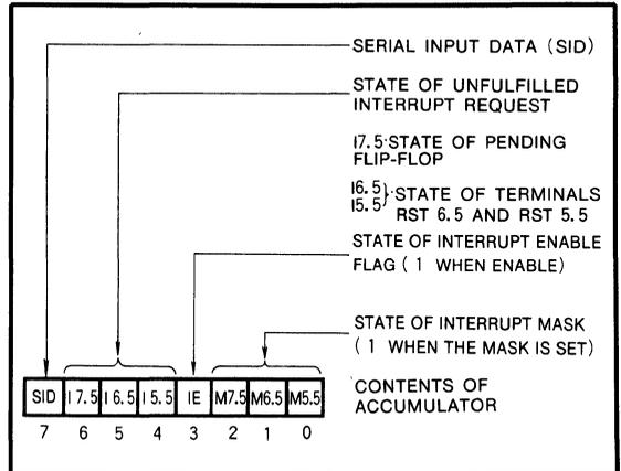
Fig.7 Relation of the SIM instruction RIM with the accumulator
