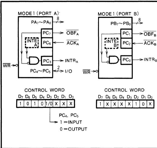
Fig. 5 An example of mode 1 output state
