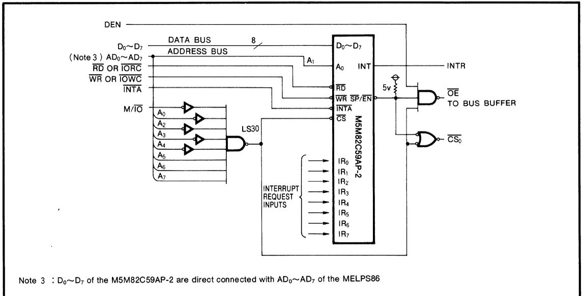
Note 3 : D<sub>0</sub>~D<sub>7</sub> of the M5M82C59AP-2 are direct connected with AD<sub>0</sub>~AD<sub>7</sub> of the MELPS86
