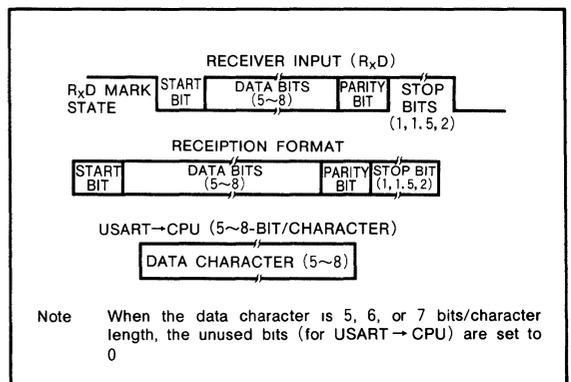
Note When the data character is 5, 6, or 7 bits/character length, the unused bits (for USART → CPU) are set to 0
