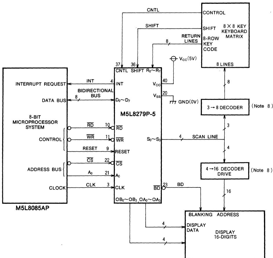
Note 8 : When using an 8-bit character display of more than 9 digits for the decoder display, it is necessary to provide two decoders for example 4 → 10 decoder, 4 → 16 decoder and key scan 3 → 8 decoder. Only S<sub>0</sub>, S<sub>1</sub> and S<sub>2</sub> may be used as inputs to the key scan 3 → 8 decoder. (Don't drive the keyboard decoder with the MSB of the scan line)
