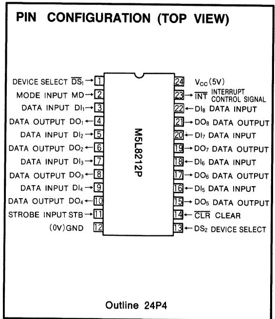
When MD is high, the data in the data latches is transferred to the data outputs. When  $\overline{DS}_1$  is low and  $DS_2$  is high, the data inputs are latched in the data latches. The low-level clear input  $\overline{CLR}$  resets the data latches and sets the service request flip-flop SR, but the state of the output buffers is not changed.
