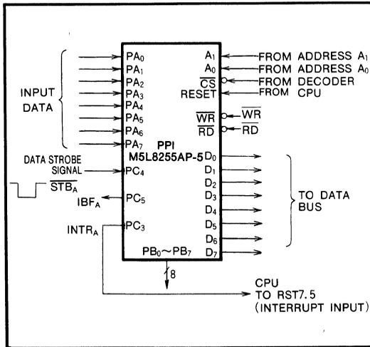
Fig. 12 A circuit for an application using mode 1
