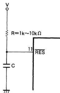
Since the MELPS 86, 88 require a reset pulse over 50 μs after V<sub>CC</sub> reaches 4.5V upon power on, the capacitor value should be determined by the graph shown below. Note that the time for V<sub>CC</sub> to reach 4.5V has not been considered, so that it is necessary to choose the characteristics value of capacitance under consideration of the power supply.
