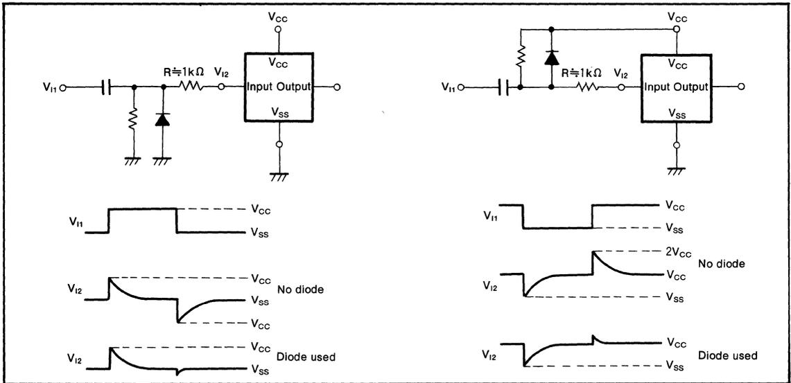
Fig. 13 Preventing latchup when using differential circuits
