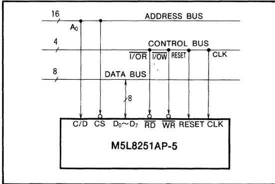
Fig. 1 M5L8251AP-5 interface to CPU system bus
