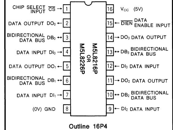
The terminal  $\overline{DIEN}$  controls the data flow. The data flow control is performed by placing one of a pair of buffers in high-impedance state and allowing the other to transfer the data.
