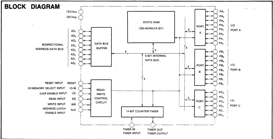
**CMOS 2048-BIT STATIC RAM WITH I/O PORTS AND TIMER**
