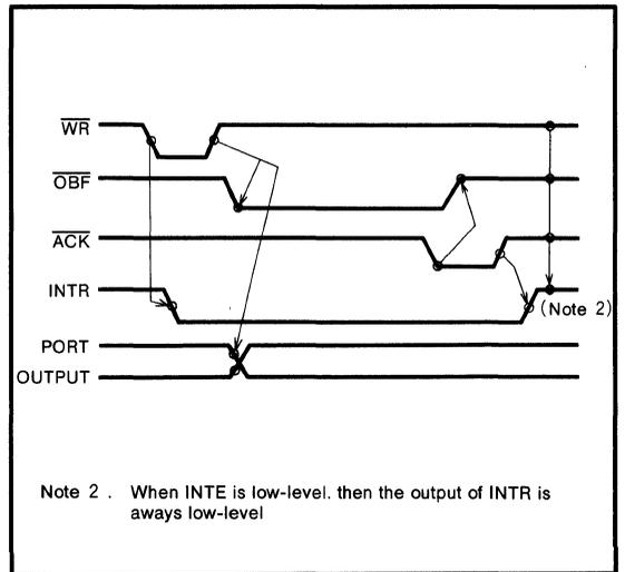
Fig. 6 Timing diagram
