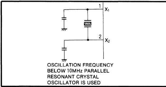
Fig. 5 Connections when crystal is used for X<sub>1</sub> and X<sub>2</sub> inputs
