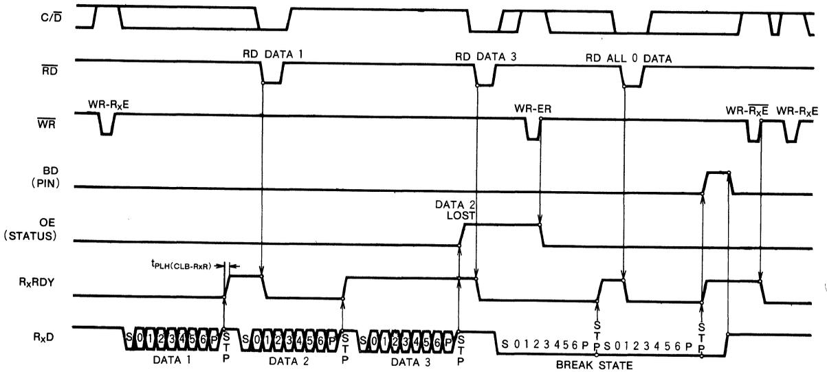
Note 14 : Example format = 7 bits/character with parity & 2 stop bits
