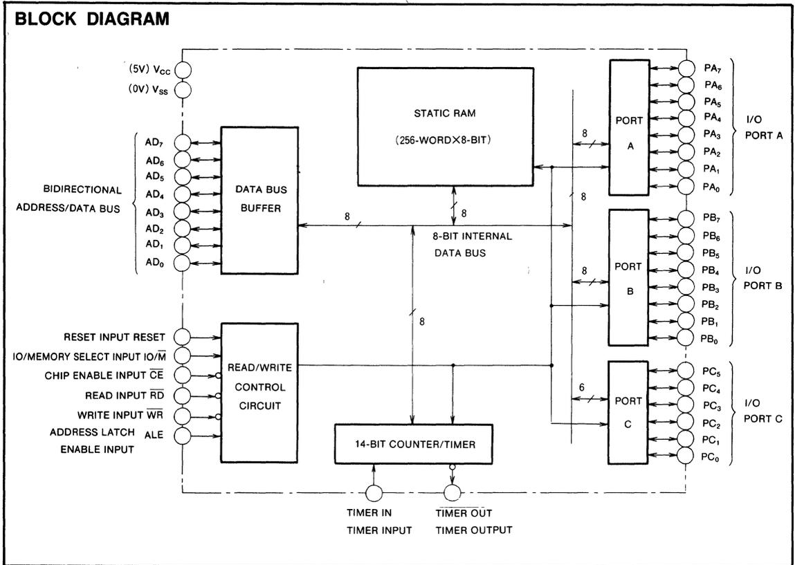
CMOS 2048-BIT STATIC RAM WITH I/O PORTS AND TIMER
