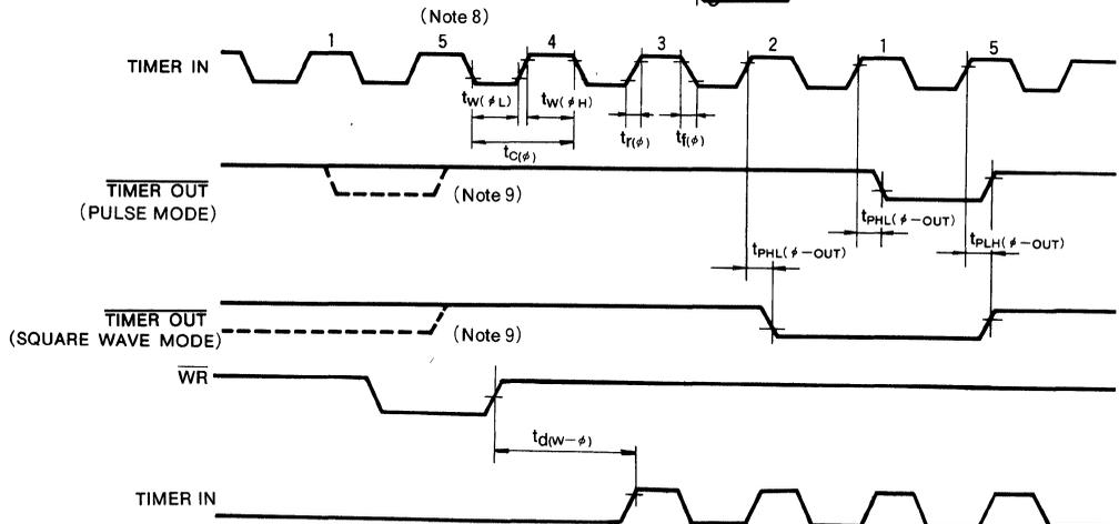
Note 8 : The wave form is shown for the case of counting down from 5 to 1.
