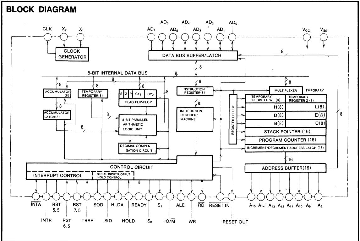
**CMOS 8-BIT PARALLEL MICROPROCESSOR**
