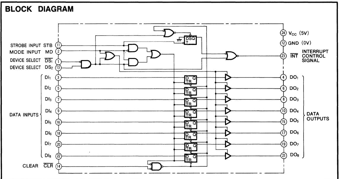
8-BIT INPUT/OUTPUT PORT WITH 3-STATE OUTPUT
