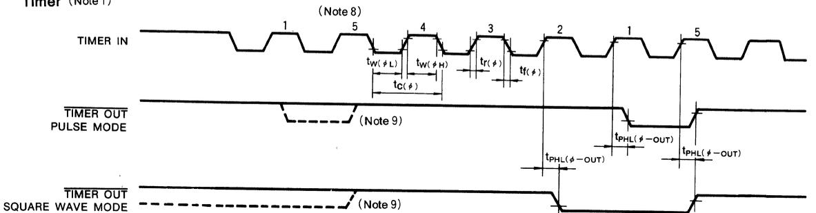
Note 8 : The wave form is shown for the case of counting down from 5 to 1
