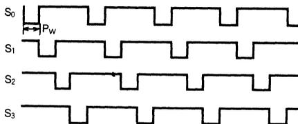
Note 4 : Here  $P_w$  is  $640\mu s$  if the internal clock frequency is set to 100kHz.
