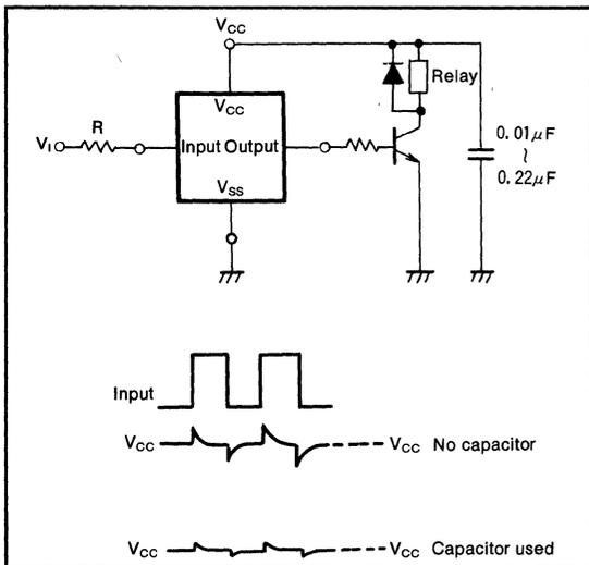
Fig. 14 Preventing latchup when driving large current circuits
