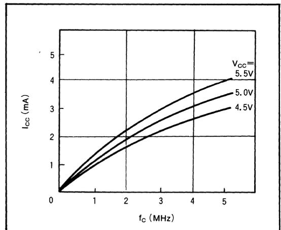
Fig. 6 Operating frequency vs. power dissipation
