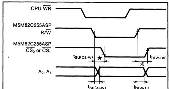
Fig. 4 Write operation of the M5M82C255ASP
