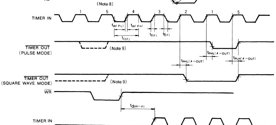
Note 8 : The wave form is shown for the case of counting down from 5 to 1
