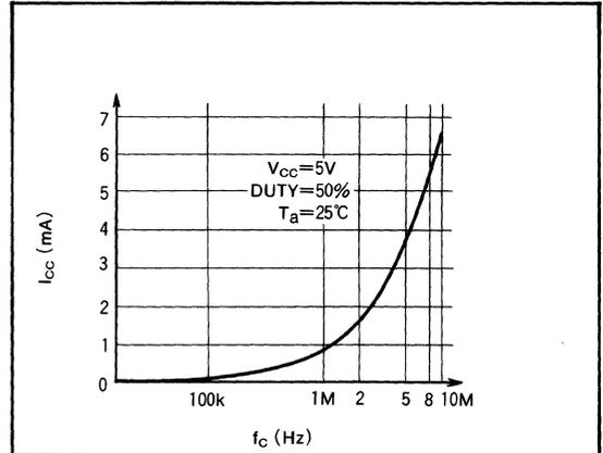
Fig. 5 Operating frequency vs. power dissipation
