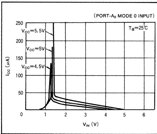
Fig. 4 Input voltage vs. dissipation current
