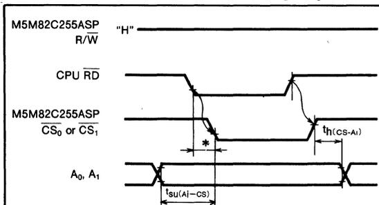
Fig. 3 Read operation of the M5M82C255ASP
