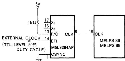
The frequency should be three times the CPU cycle frequency
