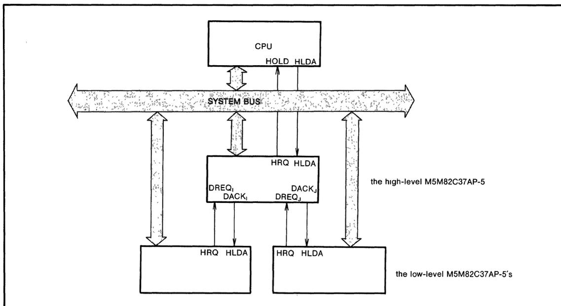
Fig.1 Example of a DMA system using a cascade connection
