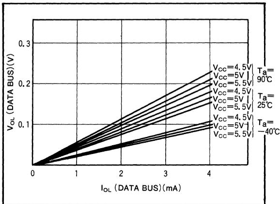
Fig. 9  $I_{OL}$ - $V_{OL}$  characteristics M5M82C55AP-2
