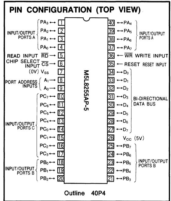
bit bidirectional bus port and one 5-bit control port. Bit set/reset is controlled by CPU. A high-level reset input (RESET) clears the control register, and all ports are set to the input mode (high-impedance state).
