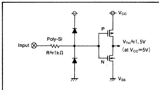
Fig. 10 CMOS peripheral device input circuit (equivalent diagram)
