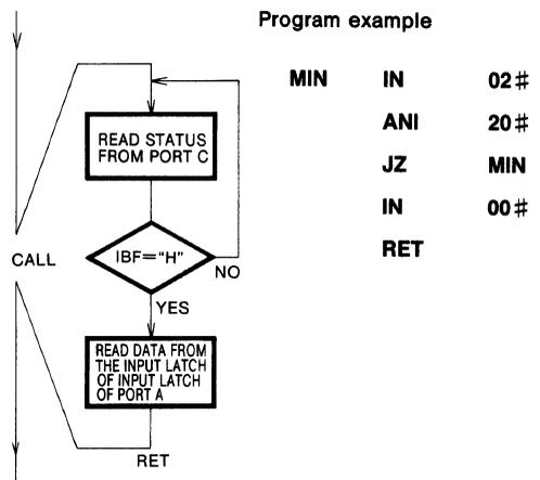
3. Slave CPU subroutine for transmitting data to the master CPU.
