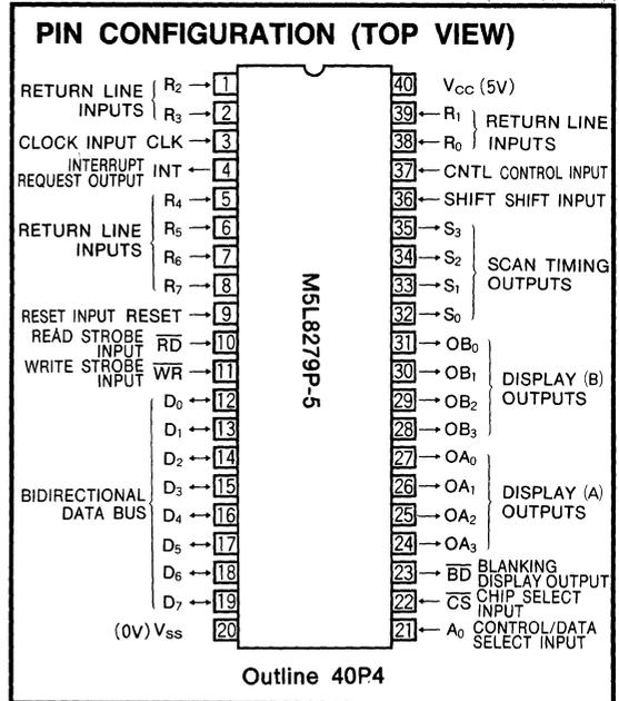
debounce buffer and an 8 X 8-bit FIFO/SENSOR RAM. It operates in any one of the scanned keyboard mode, scanned sensor matrix mode or strobed entry mode. The display portion is provided with a 16 X 8-bit display RAM that can be organized into a dual 16X 4 configuration. Also, an 8-digit display configuration is possible by means of programming.
