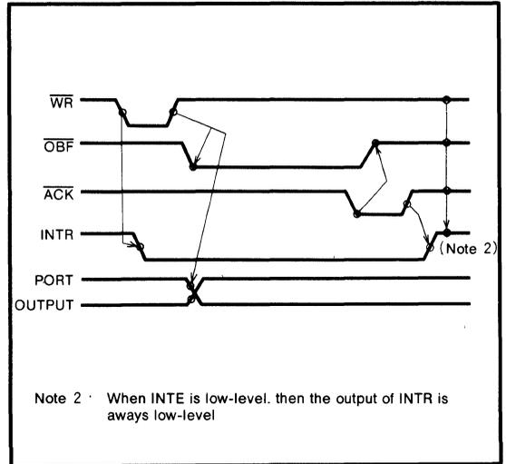
Fig. 6 Timing diagram
