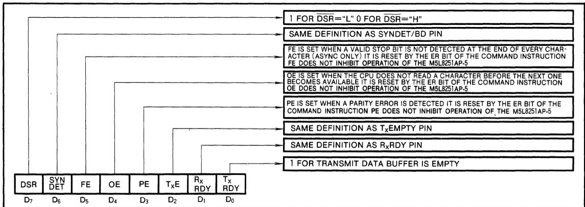
Fig. 10 Status information ( $\overline{C/D}="H"$ ,  $\overline{WR}="L"$ )
