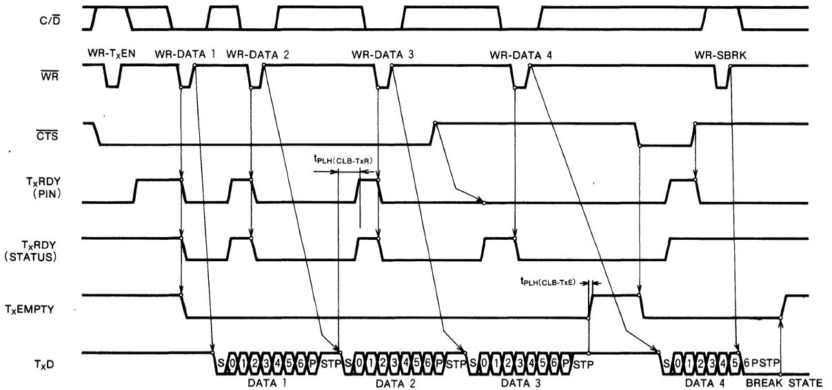
Note 11 : Example format = 7 bits/character with parity & 2 stop bits
