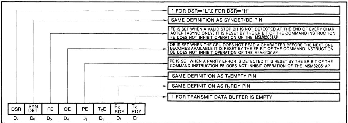
Fig. 10 Status information  $C/\overline{D}$ ="H",  $\overline{RD}$ ="L")
