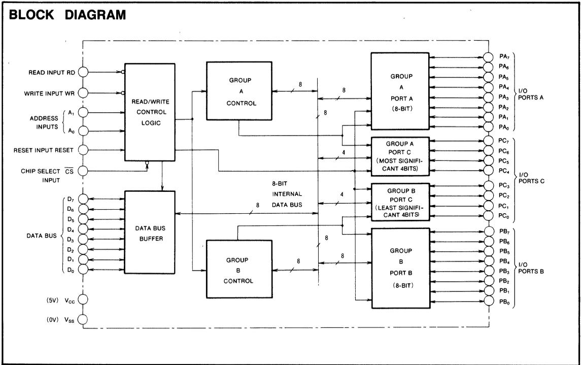
**CMOS PROGRAMMABLE PERIPHERAL INTERFACE**
