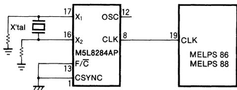
The crystal frequency should be three times the cycle time of the 8086, 8088 or 8089, and the crystal should be located as close to the M5L8284AP as possible.
