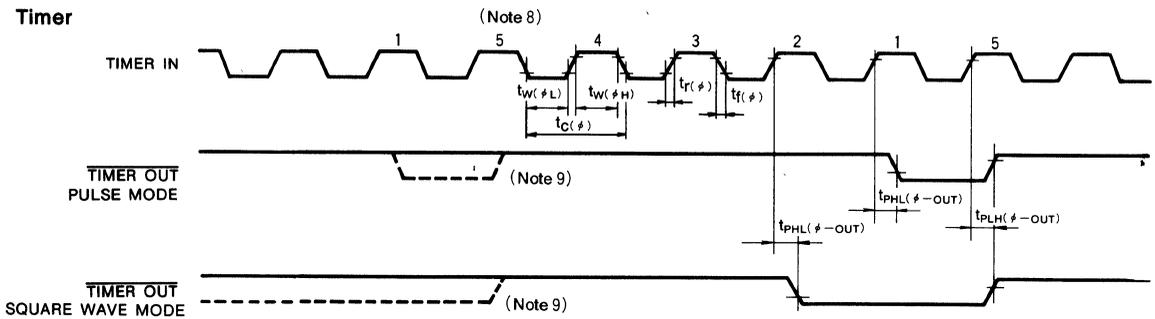
Note 8 : The wave form is shown for the case of counting down from 5 to 1
