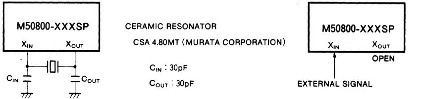
Externally connected ceramic resonator circuit
