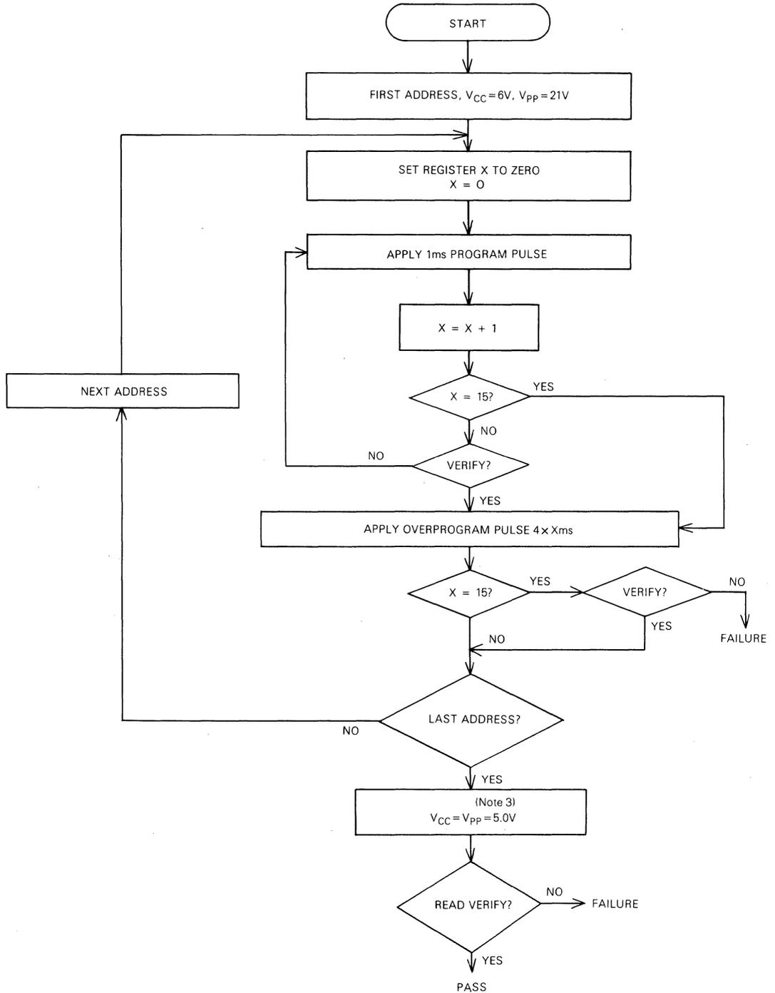
Note 3:  $4.75 \leq V_{CC} = V_{PP} \leq 5.25V$
