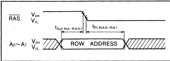
Fig. 1.16 Row address latching timing relationships
