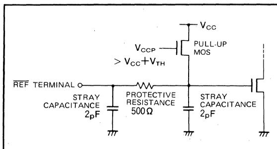
Fig. 1.33  $\overline{\text{REF}}$  input equivalent circuit
