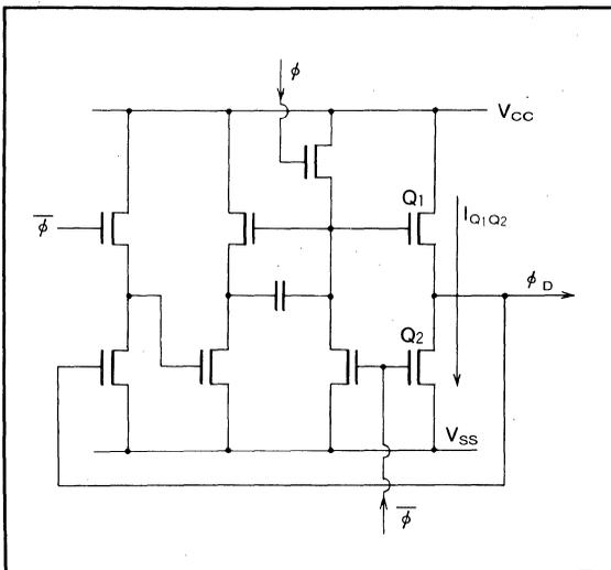
Fig. 1.4 Driver circuit
