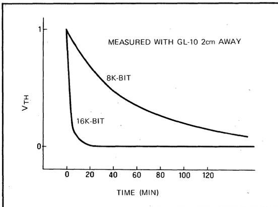
Fig. 3.4 Variation in  $V_{TH}$  with erasure time
