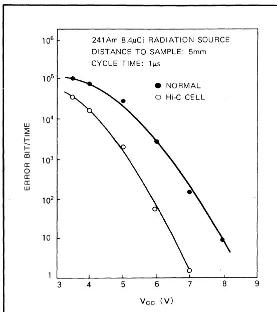
**Fig. 1.7 Soft error rate dependency on supply voltage**
