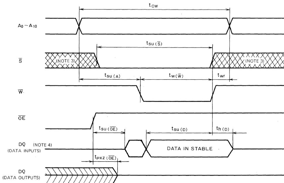
Write Cycle 2 ( $\overline{S}$  Control Mode)
