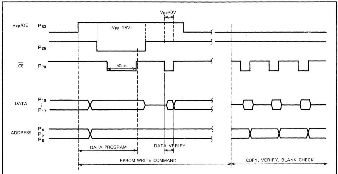
**Fig. 3.14 2732 Programming timing**
