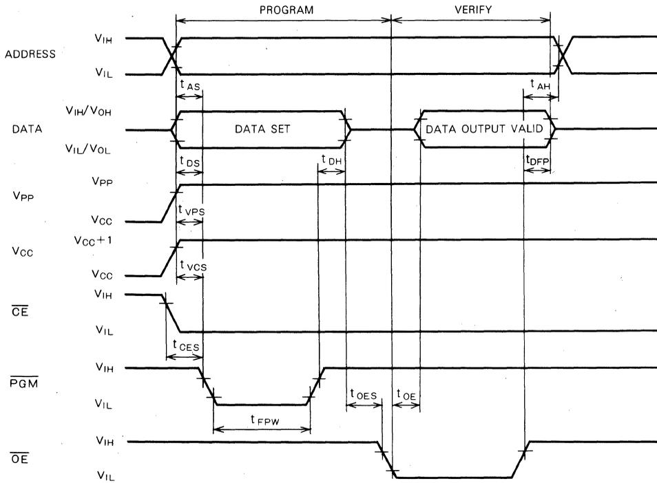
Test conditions for A.C. characteristics
