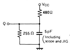
**Fig. 2 Output load for  $t_{en}$ ,  $t_{dis}$**
