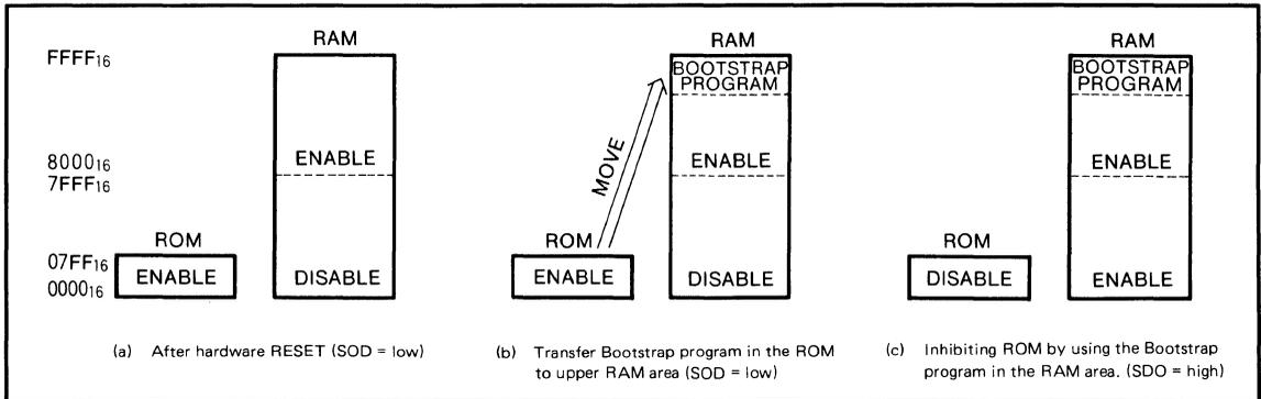
Fig. 1.49 Start-up procedure of the memory-overlapped system
