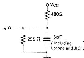
**Fig. 2 Output load for  $t_{en}$ ,  $t_{dis}$**
