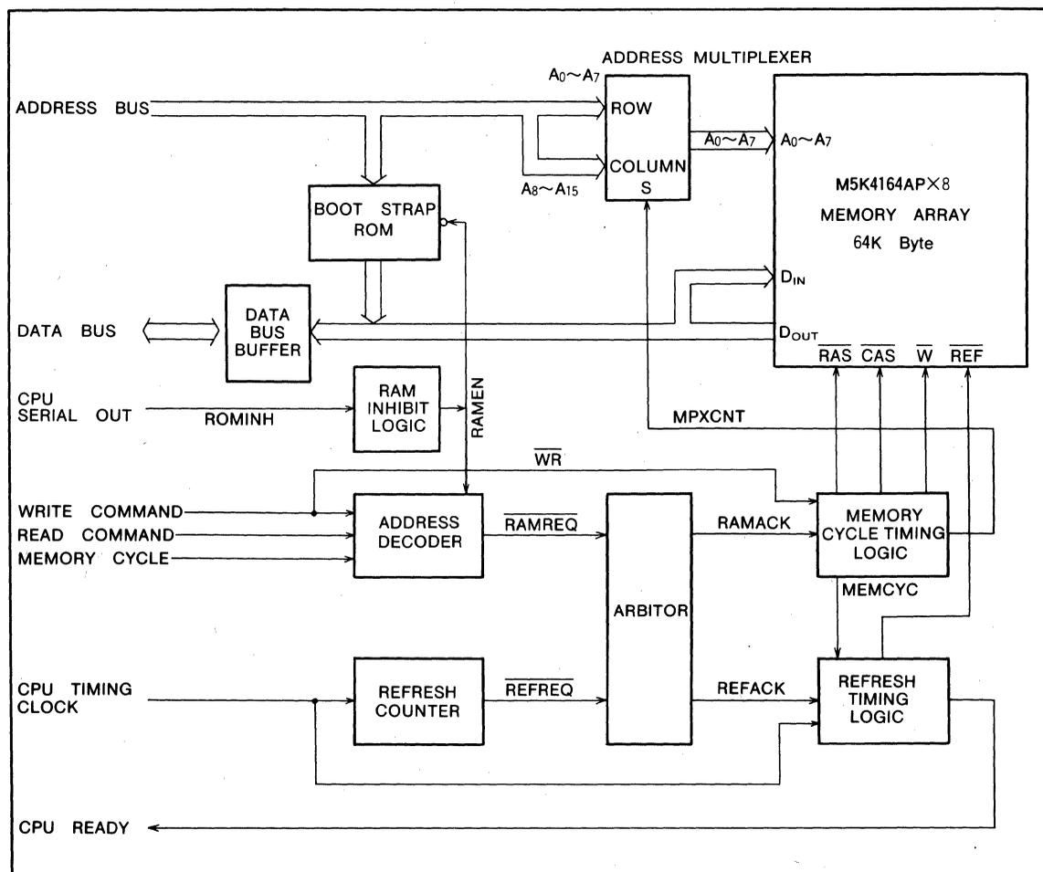
Fig. 1.46 Block diagram of the design example (Asynchronous)
