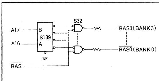
Fig. 1.42 (b)  $\overline{\text{RAS}}$  decoder using  $\overline{\text{REF}}$  pin
