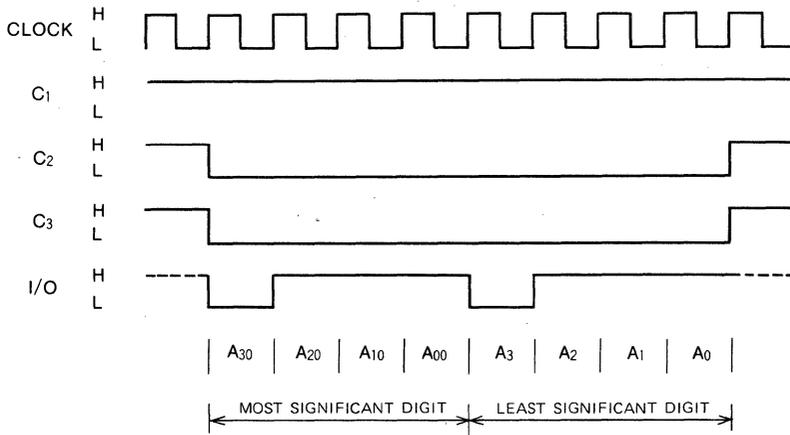
Note 2: The addresses from  $A_{00}$  to  $A_{33}$  are designated by two one-of-four coded digits. The above figure shows designation of address  $A_{33}$  (decimal address 15).
