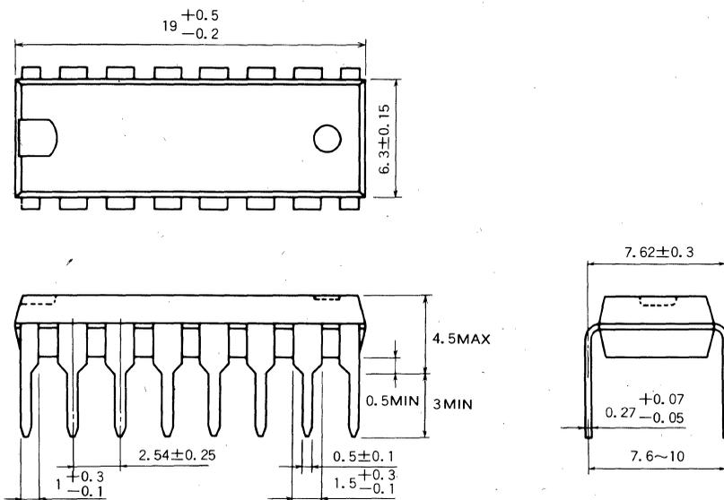
**TYPE 16S1 16-PIN METAL-SEALED CERAMIC DIL**
