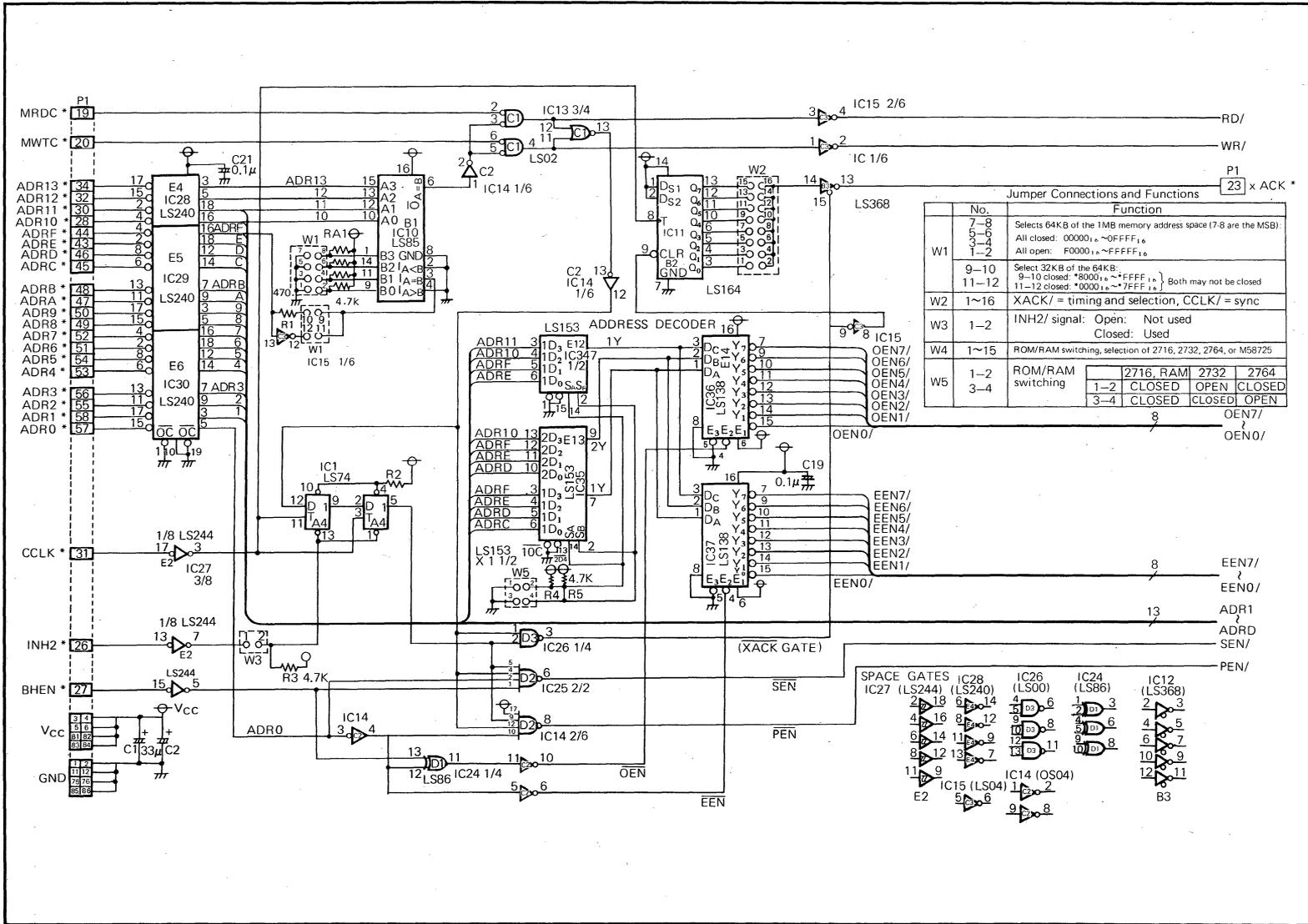
Fig. 3.16 Design example of EPROM/RAM board (2/2)
