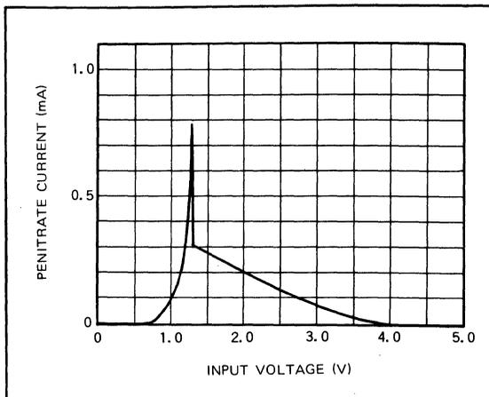
Fig. 2.17 Penetrate current of CMOS inverter
