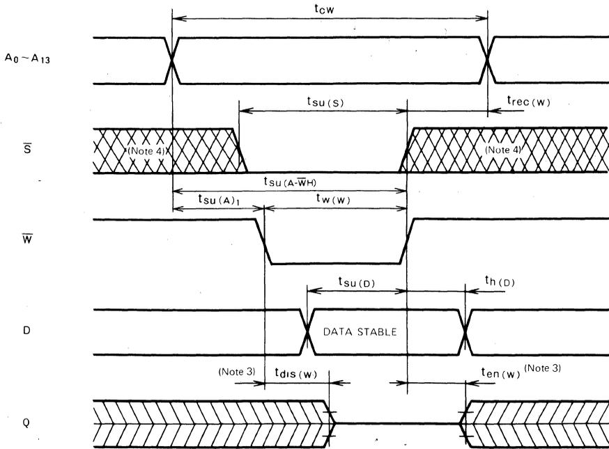
Write cycle 2 ( $\overline{S}$  control mode)
