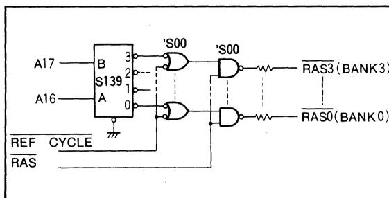
Fig. 1.42 (a)  $\overline{\text{RAS}}$  decoder in  $\overline{\text{RAS}}$ -only refresh
