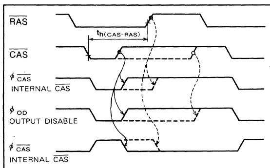
**Fig. 1.15 Relationship of  $\overline{\text{RAS}}$  and  $\overline{\text{CAS}}$  rising edges to internal clock timing**
