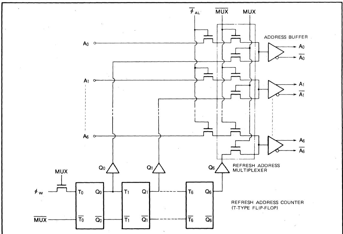
Fig. 1.28 Refresh address counter and multiplexer circuits
