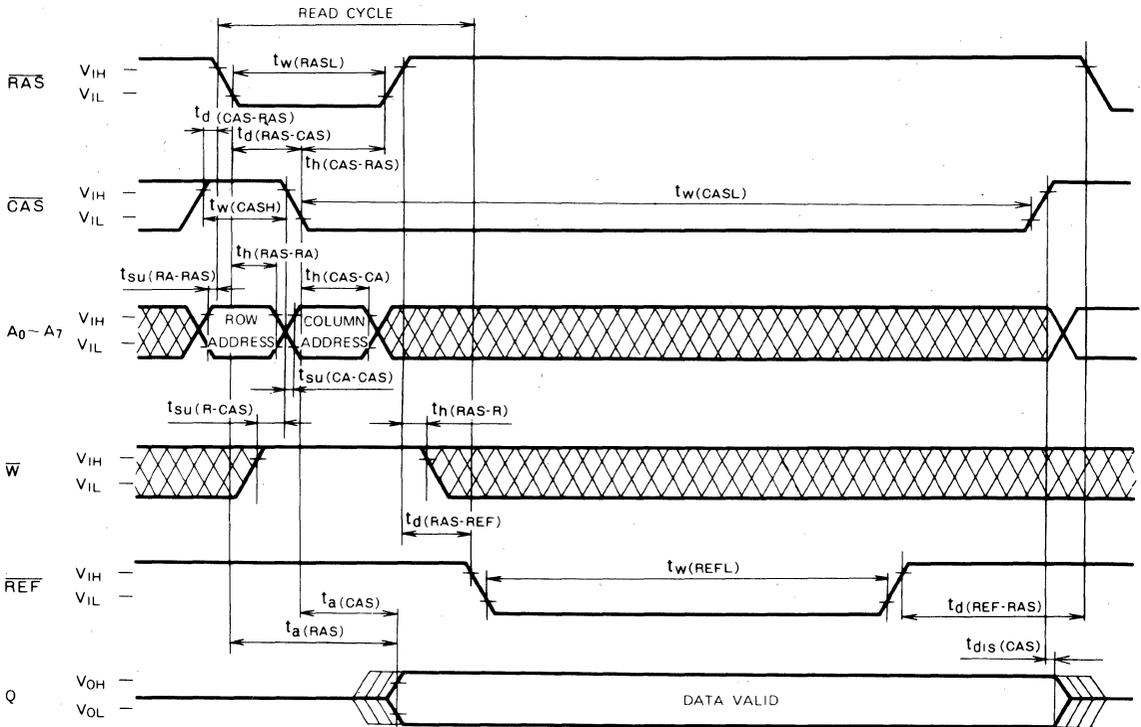
Note 22. If the pin 13 ( $\overline{\text{REF}}$ ) function is not used, pin 13 may be left open (not connect).
