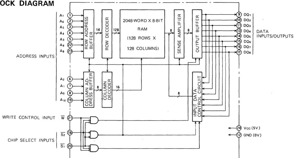
**16384-BIT (2048-WORD BY 8-BIT) CMOS STATIC RAM**
