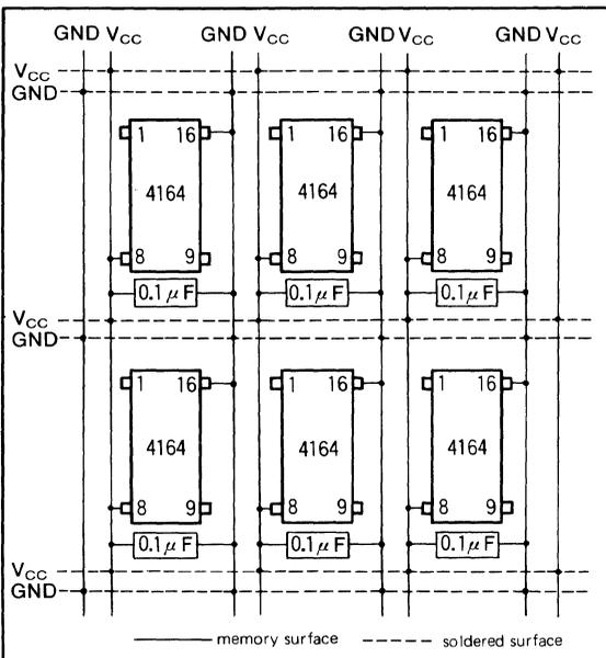
Fig. 1.39 (a) Gridded power distribution and decoupling capacitors
