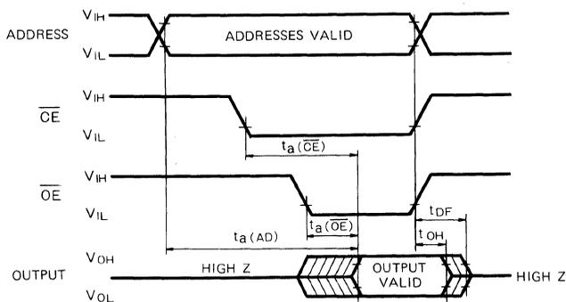
**Test Conditions for A.C. Characteristics**
