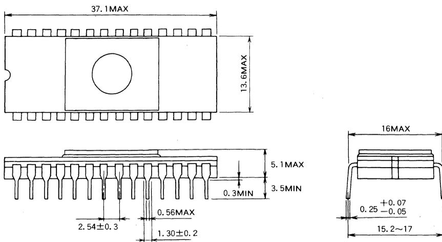
TYPE 28K4 28-PIN GLASS-SEALED CERAMIC DIL WITH TRANSPARENT LID
