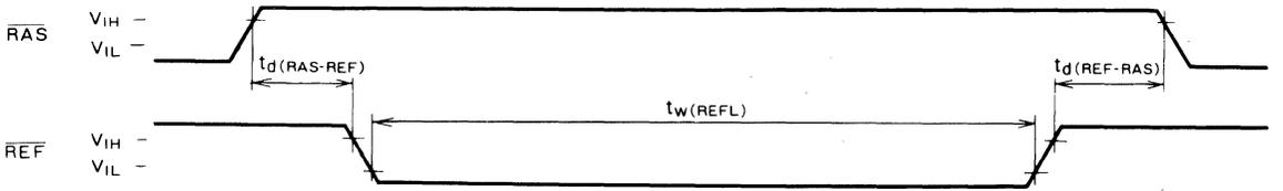
Note 21  $\overline{\text{CAS}}$ , Addresses, D and  $\overline{\text{W}}$  are don't care.
