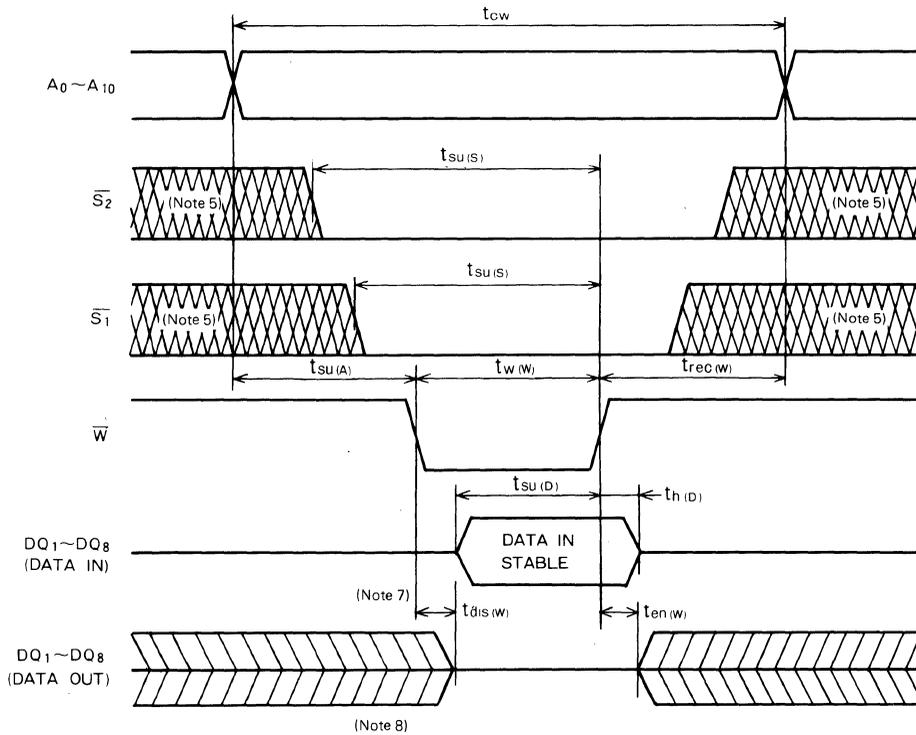
**16384-BIT (2048-WORD BY 8-BIT) CMOS STATIC RAM**
