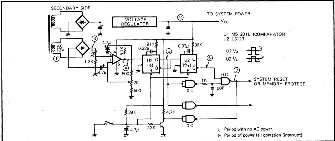
Fig. 2.21 Power-fail-detect circuit
