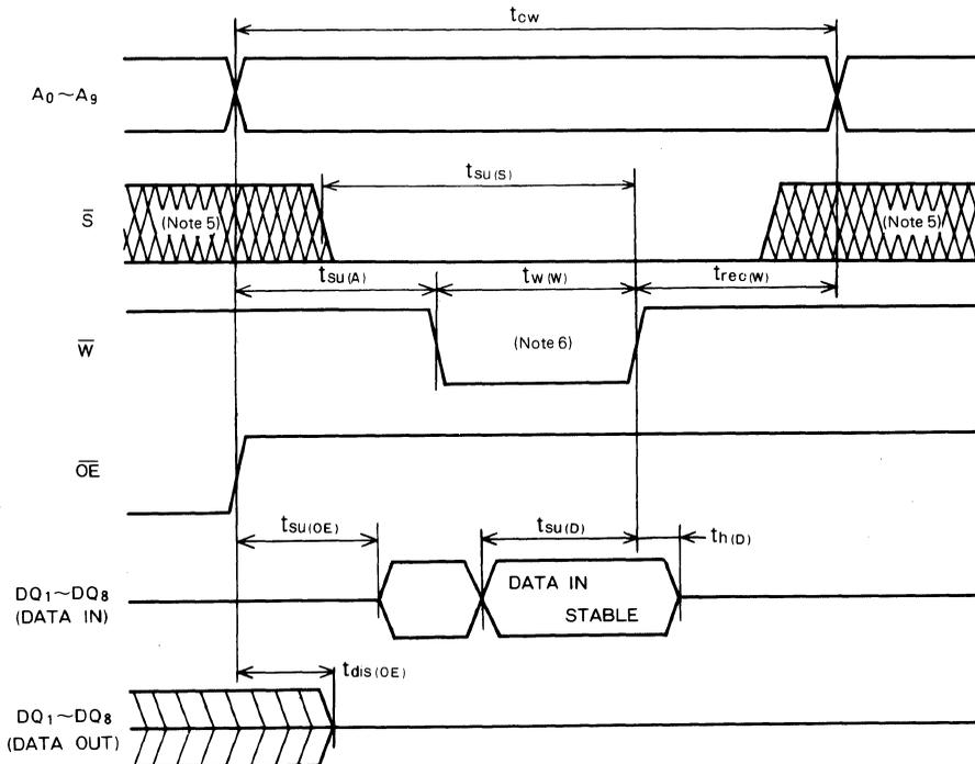
**16384-BIT (2048-WORD BY 8-BIT) CMOS STATIC RAM**
