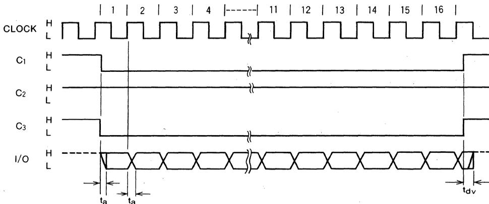
**Timing of clock,  $C_1$ ,  $C_2$ ,  $C_3$ , and data input**
