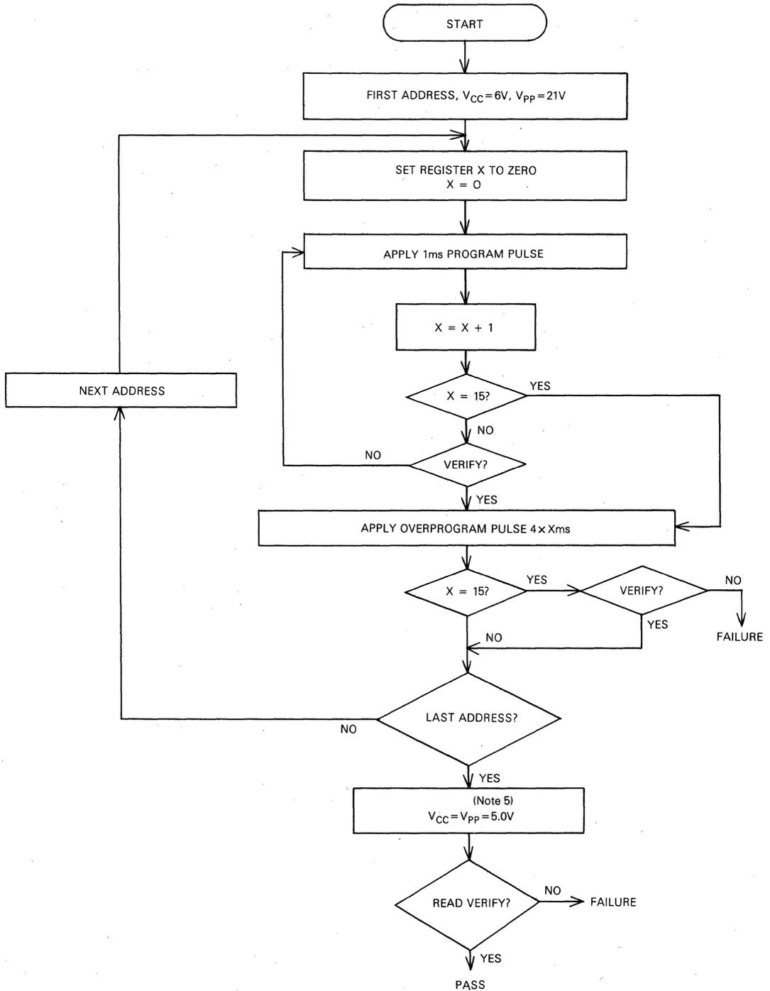
Note 5:  $4.75 \leq V_{CC} = V_{PP} \leq 5.25V$
