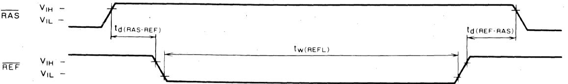
Note 20:  $\overline{\text{CAS}}$ , Addresses, D and  $\overline{\text{W}}$  are don't care.
