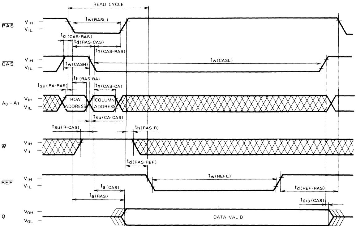
Note 21: If the pin 1 ( $\overline{REF}$ ) function is not used, pin 1 may be left open (not connect).
