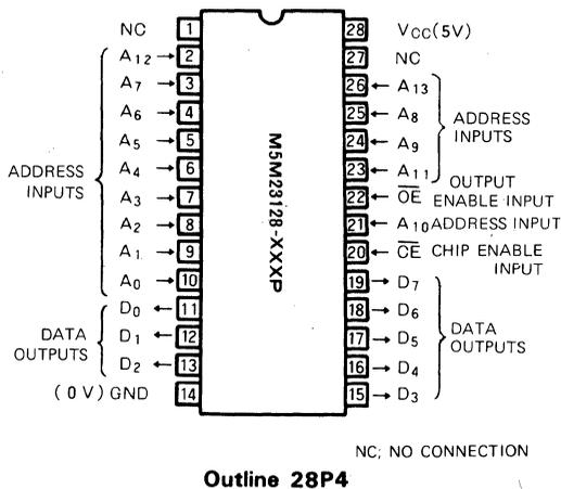
When the  $\overline{CE}$  or  $\overline{OE}$  signal is high, data output are in a floating state.
