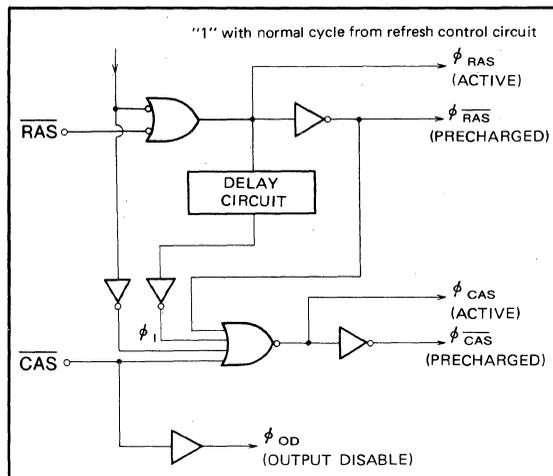
Fig. 1.12 Internal  $\overline{RAS}$  and  $\overline{CAS}$  clock generating circuit
