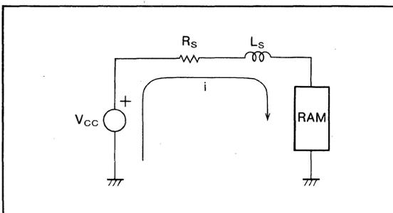
Fig. 1.38 (a) PC board trace equivalent circuit
