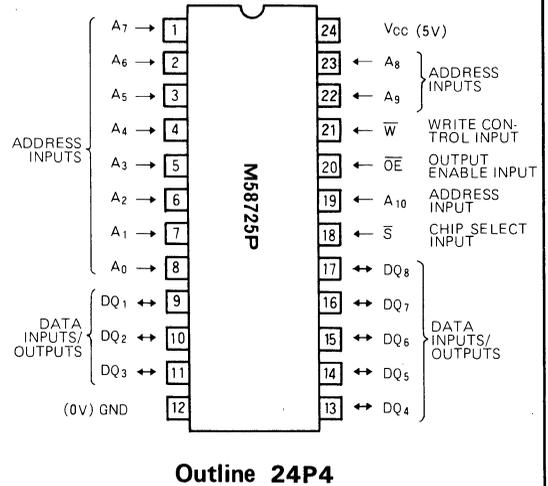
During a read cycle, when a location is designated by address signals  $A_0 \sim A_{10}$  the  $\overline{OE}$  signal is kept low to keep the DQ terminals in the output mode, signal  $\overline{W}$  goes high, and the data of the designated address is available at the I/O terminals.
