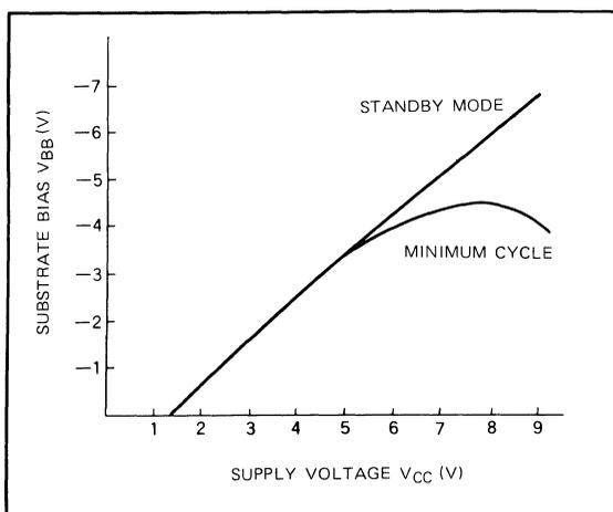
Fig. 1.3 Substrate bias vs supply voltage
