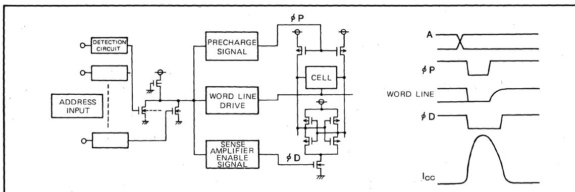
Fig. 2.3 Circuit diagram of internal synchronous circuit
