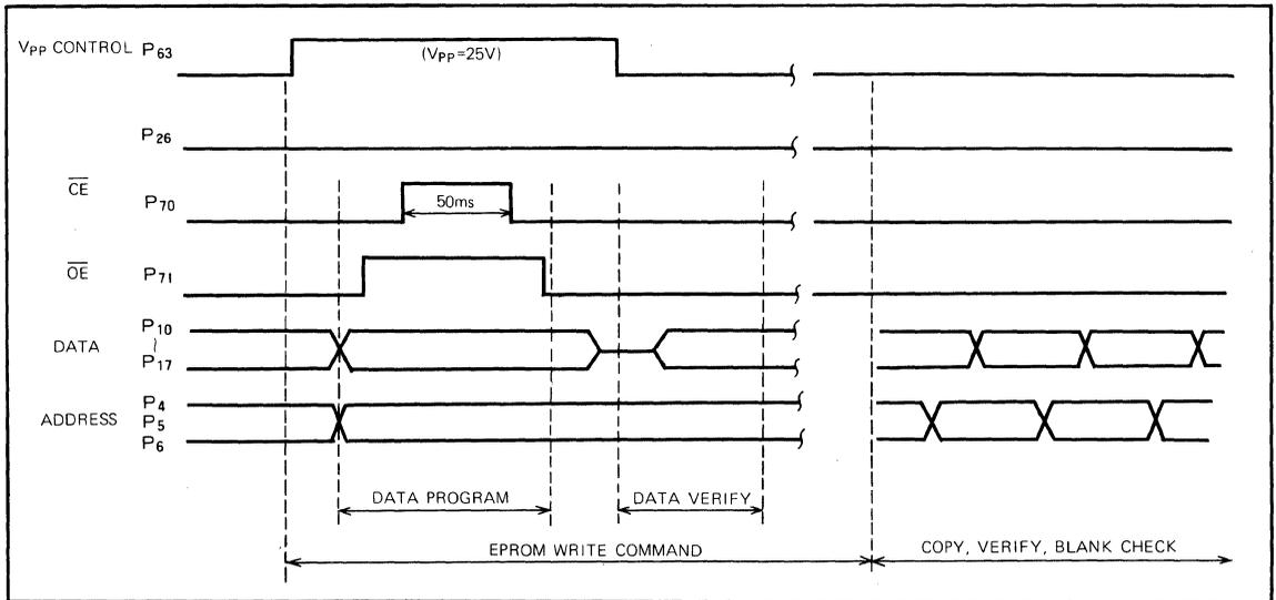
**Fig. 3.13 2716 Programming timing**
