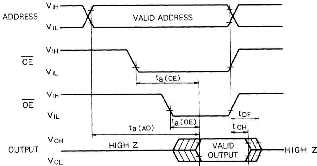
Switching Characteristics Test Conditions
