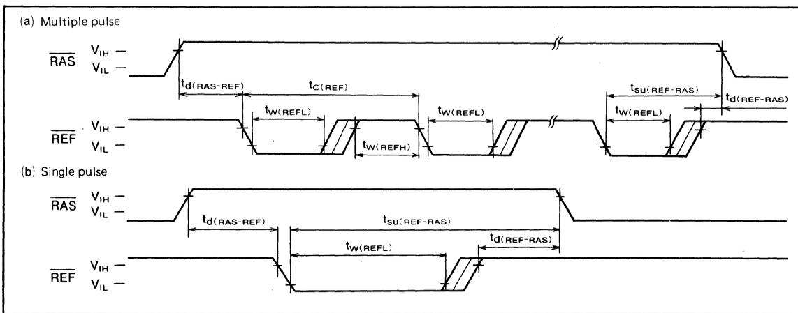
Fig. 1.31 Automatic refresh timing
