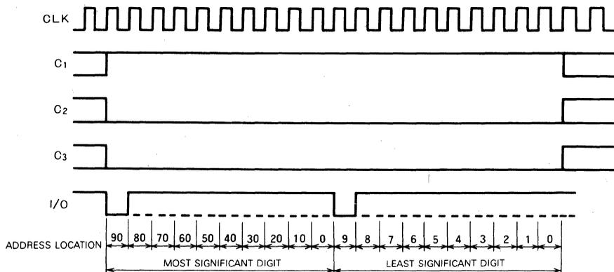
Note 3: The address is designated by two one-of-ten-coded digits. The figure shows designation of the address 99.
