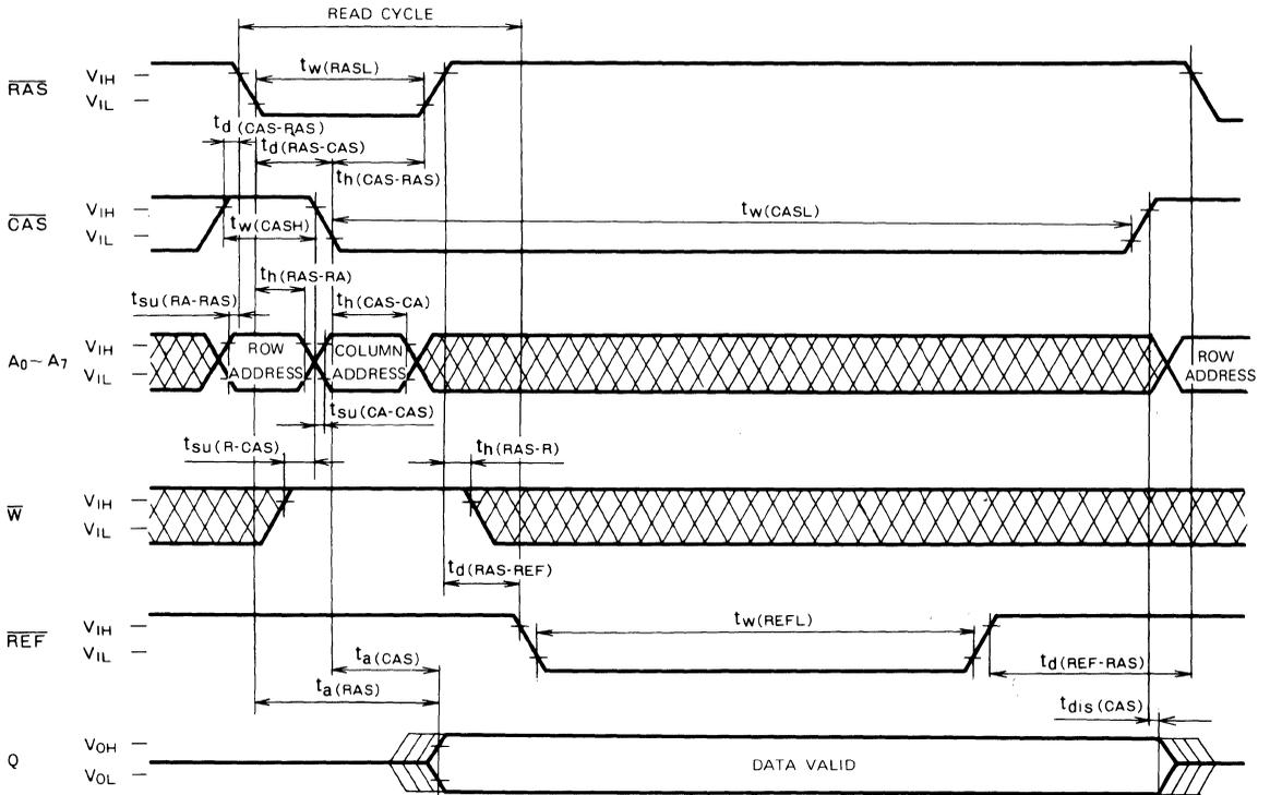
Note 22: If the pin 1 ( $\overline{\text{REF}}$ ) function is not used, pin 1 may be left open (not connect).
