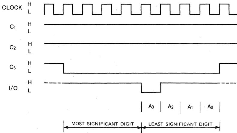
Note 3: In the AD accept address mode, the higher four are set high, and the lower four digits are designated by one of the four coded digits. This address mode allows designation of addresses from  $A_0$  to  $A_3$ . Each address has a 16 bits. The above figure shows designation of address  $A_3$ .
