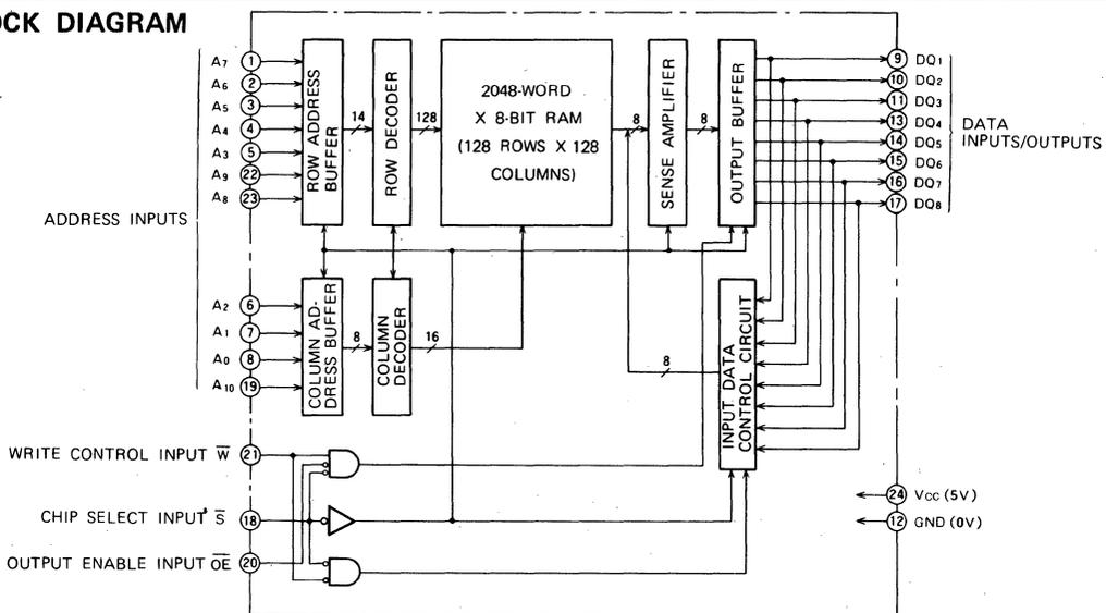
**16384-BIT (2048-WORD BY 8-BIT) CMOS STATIC RAM**
