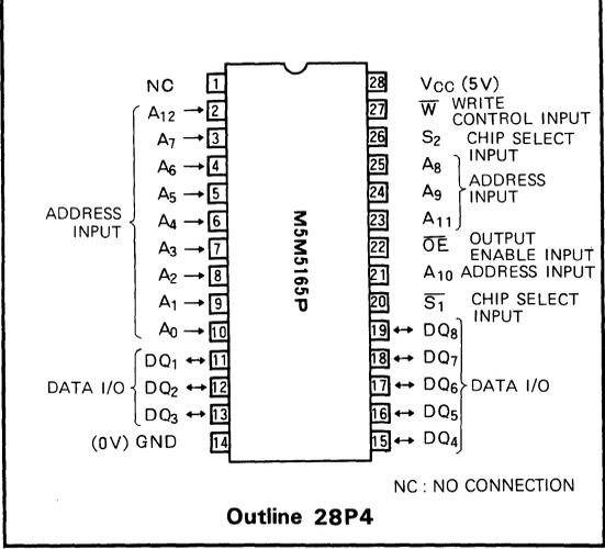
combination of the device control inputs  $\overline{S}_1, S_2, \overline{W}$  and  $\overline{OE}$ . Each mode is summarized in the function table. (see next page)
