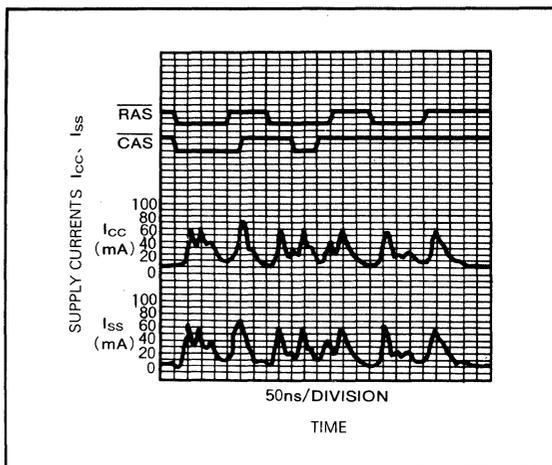
Fig. 1.37 Supply current vs time RAS/CAS cycle
