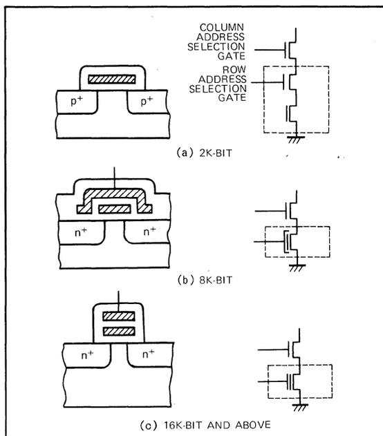
Fig. 3.1 Memory transistor construction
