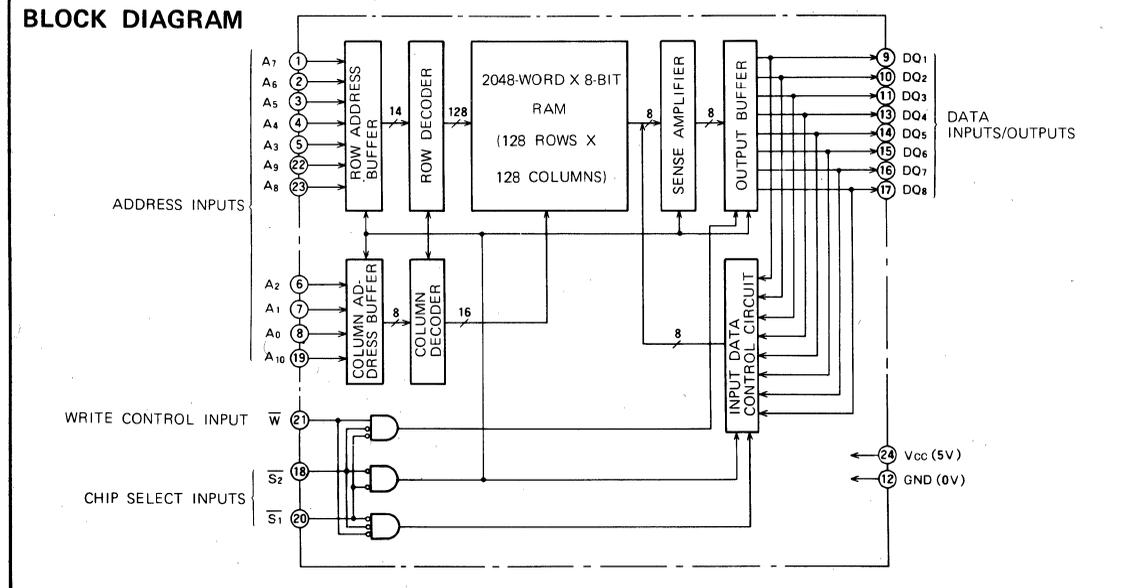
**16384-BIT (2048-WORD BY 8-BIT) CMOS STATIC RAM**
