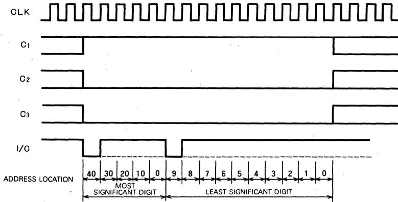
Note 3: The address is designated by two one-of-ten-coded digits. The figure shows designation of the address 49.
