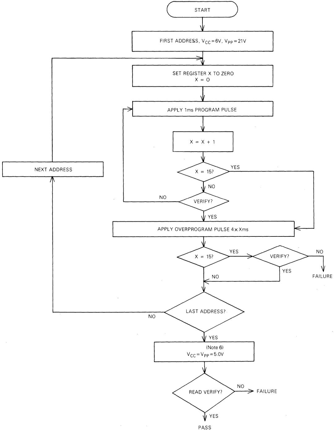
Note 6:  $4.75 \leq V_{CC} = V_{PP} \leq 5.25V$
