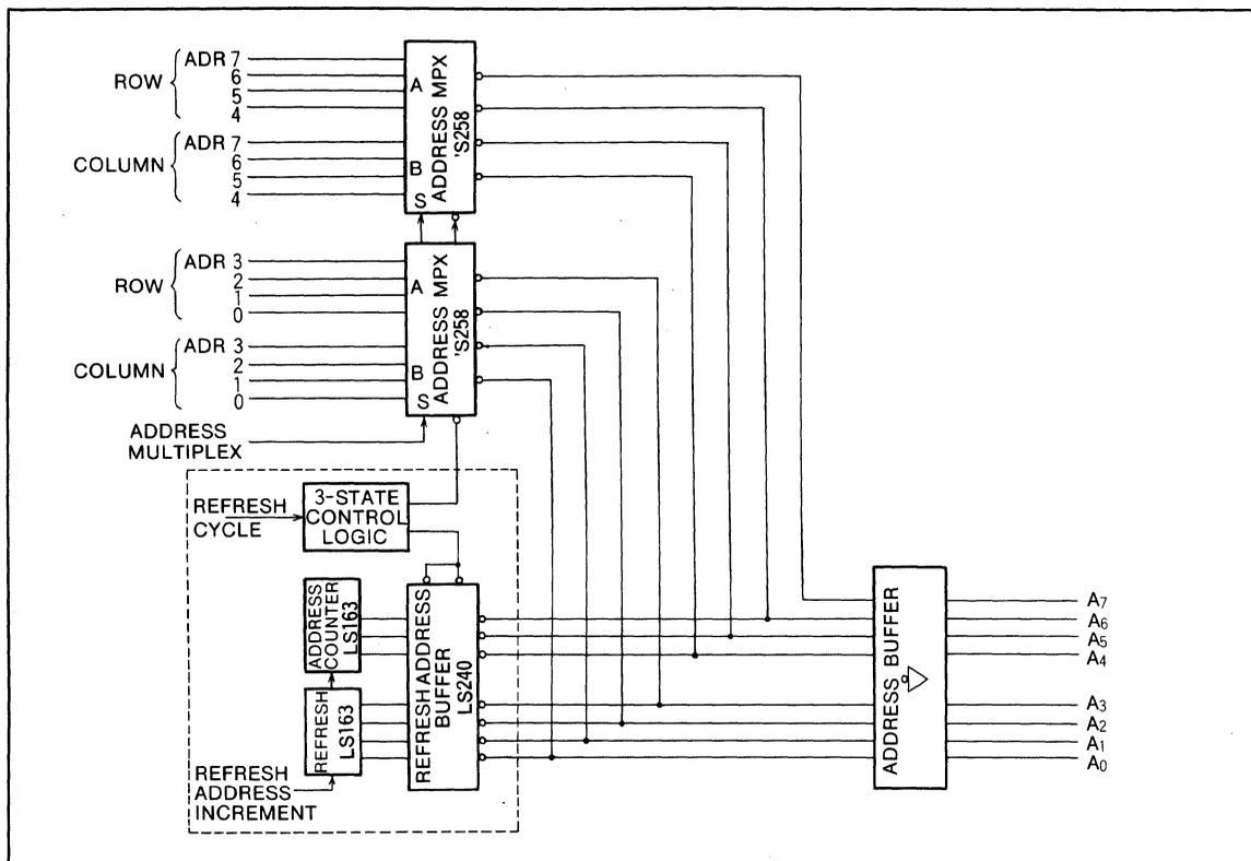
Fig. 1.41 Address multiplexer and refresh address counter
