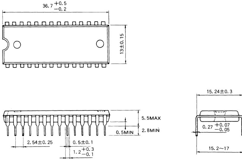
**TYPE 28K1 28-PIN GLASS-SEALED CERAMIC DIL WITH TRANSPARENT LID**
