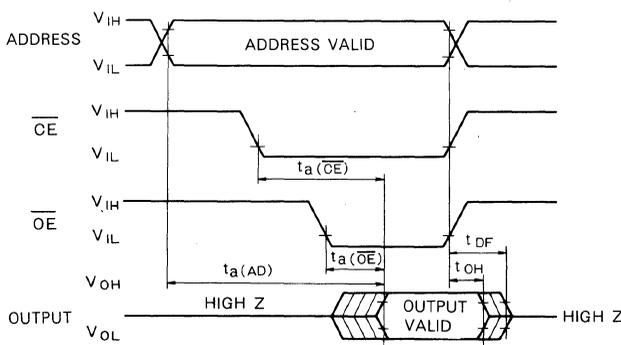
Test conditions for A.C. characteristics
