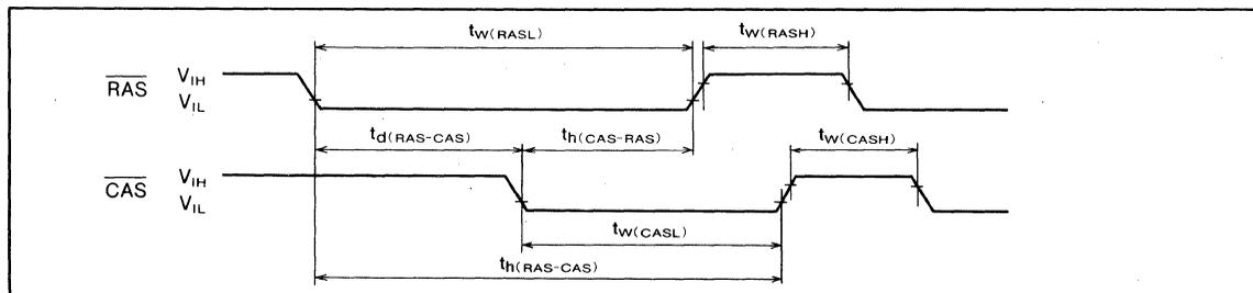
Fig. 1.13  $\overline{RAS}$ ,  $\overline{CAS}$  timing
