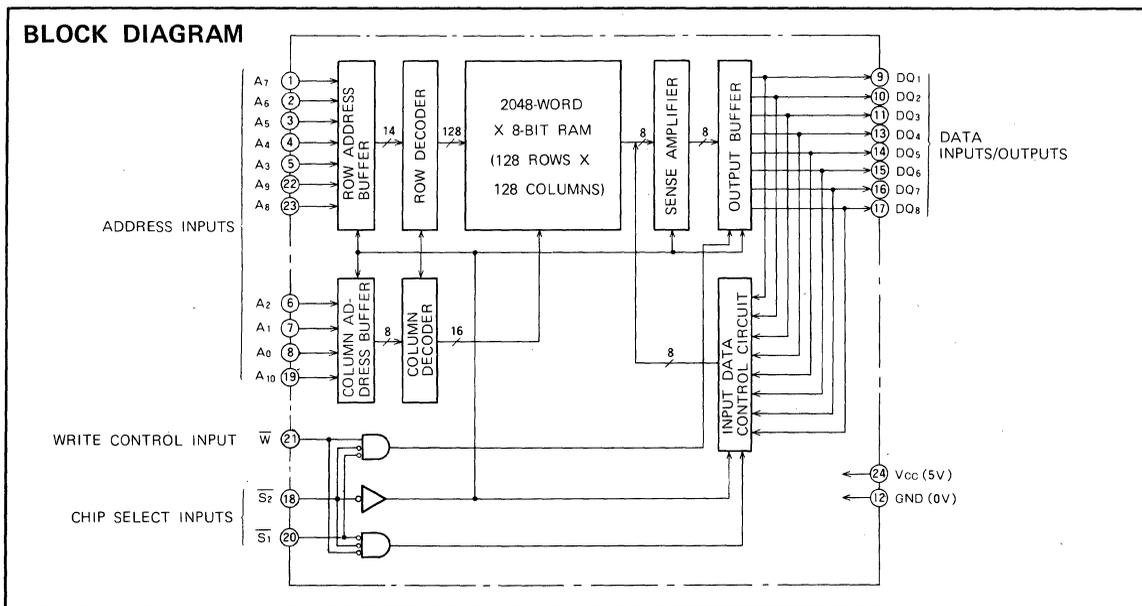
**16384-BIT (2048-WORD BY 8-BIT) CMOS STATIC RAM**
