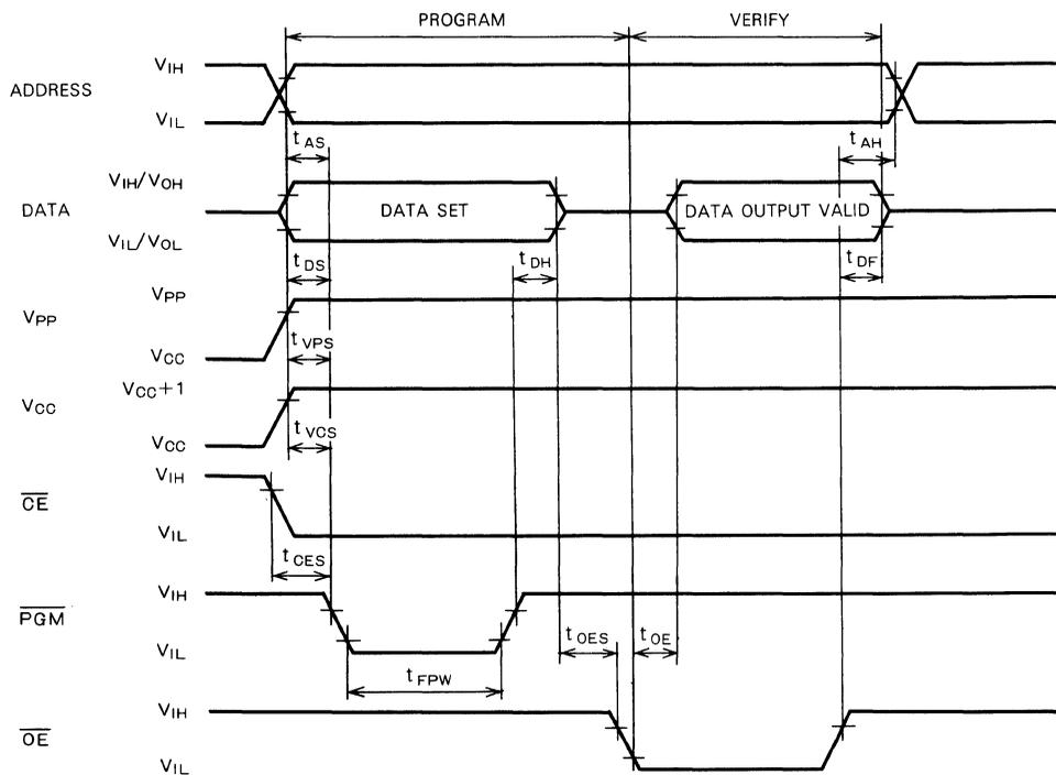
Test conditions for A.C. characteristics
