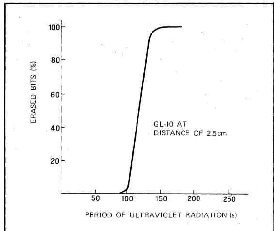
**Fig. 3.10 Erasure characteristics example for 2716 and 2732**
