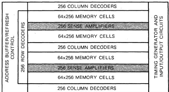
Fig. 1.9 M5K4164AP Chip arrangement
