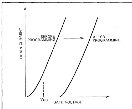
Fig. 3.2 Variation in memory transistor threshold voltage ( $V_{GO}$ : Read gate voltage, both vertical and horizontal scales are arbitrary)
