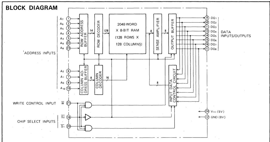
**16384-BIT (2048-WORD BY 8-BIT) CMOS STATIC RAM**
