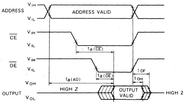
Test conditions for A.C. characteristics
