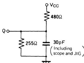
**Fig. 1 Output load**
