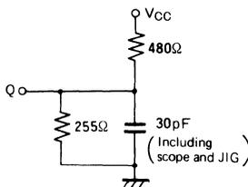
**Fig. 1 Output load**
