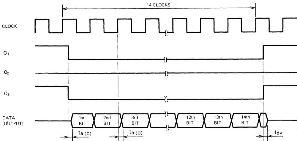
The 1st bit of output data is output after access time of  $t_{a(c)}$  from the mode control transition. And other bits are output after  $t_{a(c)}$  from positive edge of clock.
