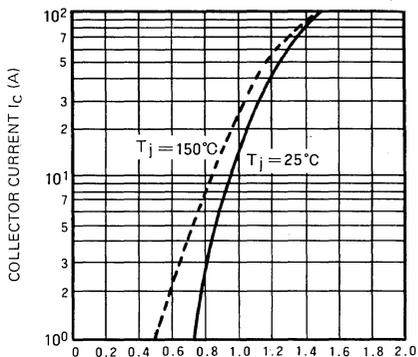
COLLECTOR-EMITTER REVERSED VOLTAGE -  $V_{CE0}$  (V)
