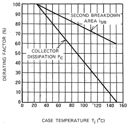
ELECTRICAL CHARACTERISTICS ( $T_j = 25^\circ\text{C}$ )
