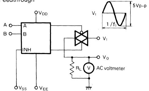
The feedthrough is taken as that frequency  $f$ , at which, using a sine wave input of  $\pm 2.5V_p$ ,  $20 \log_{10} (V_o/V_i) = -50\text{dB}$ . Refer to the function table for conditions of control inputs A and B.
