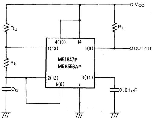
takes place when the negative going trigger pulse reaches  $1/3 V_{CC}$  and circuit stays in the output high state until the set time elapses. The time the output remains in the high state is  $1.1 R_a \cdot C_a$  and can be determined by the graph.
