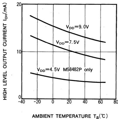
(4)  $I_{OL}-T_a$  (OUT 1, OUT 2, OUT 3)  $V_{OL}=V_{DD}$
