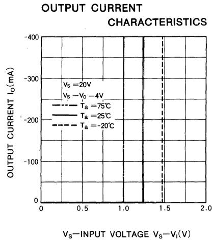
7-UNIT 300mA SOURCE TYPE DARLINGTON TRANSISTOR ARRAY
