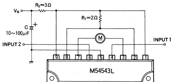
2) Motor speed control by the  $V_{CC'}$
