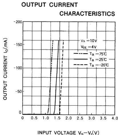
**7-UNIT 150mA SOURCE TYPE DARLINGTON TRANSISTOR ARRAY**
