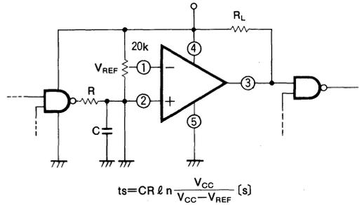
Window comparator (alarm circuit)
