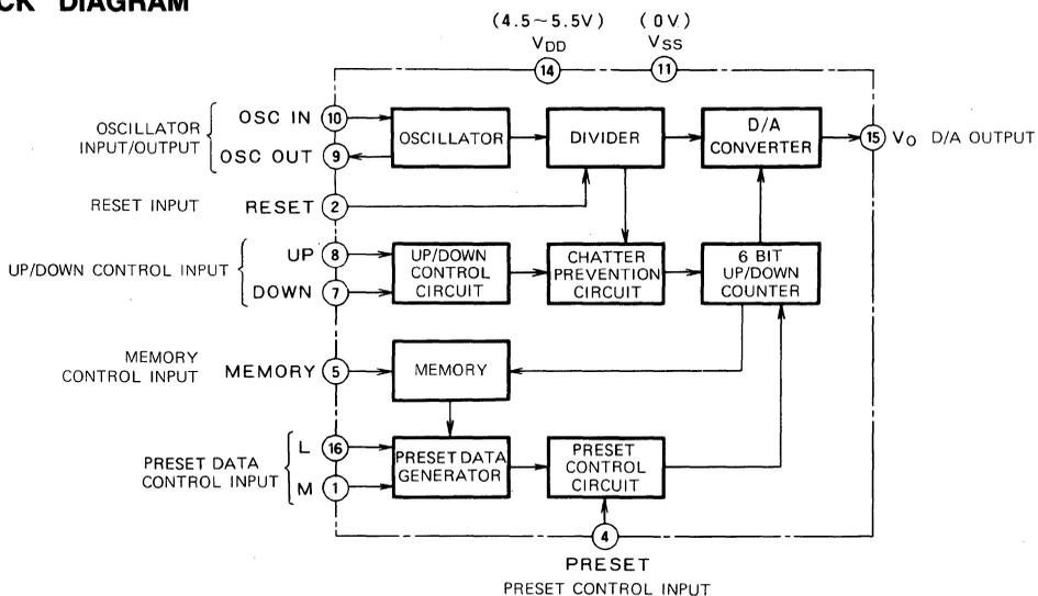
ELECTRONIC VOLUME CONTROL CMOS 6-BIT D/A CONVERTER
