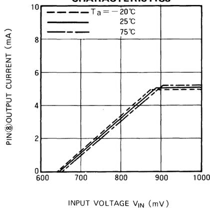
**PIN ① OUTPUT CURRENT VS INPUT VOLTAGE TEMPERATURE CHARACTERISTICS**
