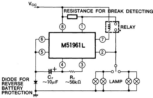
(2) Example in case of adjusting the threshold voltage for break detecting
