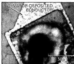
Fig. 2 Example of corrosion of an aluminum vapor-deposited conductor (analyzed using a metallogical microscope)
