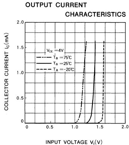
**4-UNIT 1.5A DARLINGTON TRANSISTOR ARRAY WITH CLAMP DIODE**
