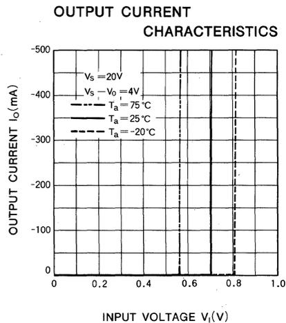
**8-UNIT 500mA SOURCE TYPE DARLINGTON TRANSISTOR ARRAY**
