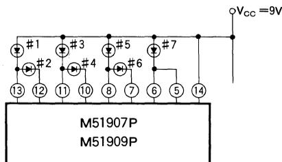
Connect similar to 1~3 according to a number of LED is odd or even. For example, in case of no use of #8 LED, connect similar to the case of no use of #2 LED.
