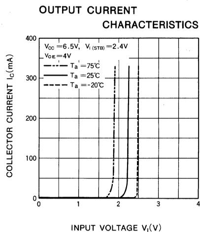
6-UNIT 320mA TRANSISTOR ARRAY WITH CLAMP DIODE AND STROBE
