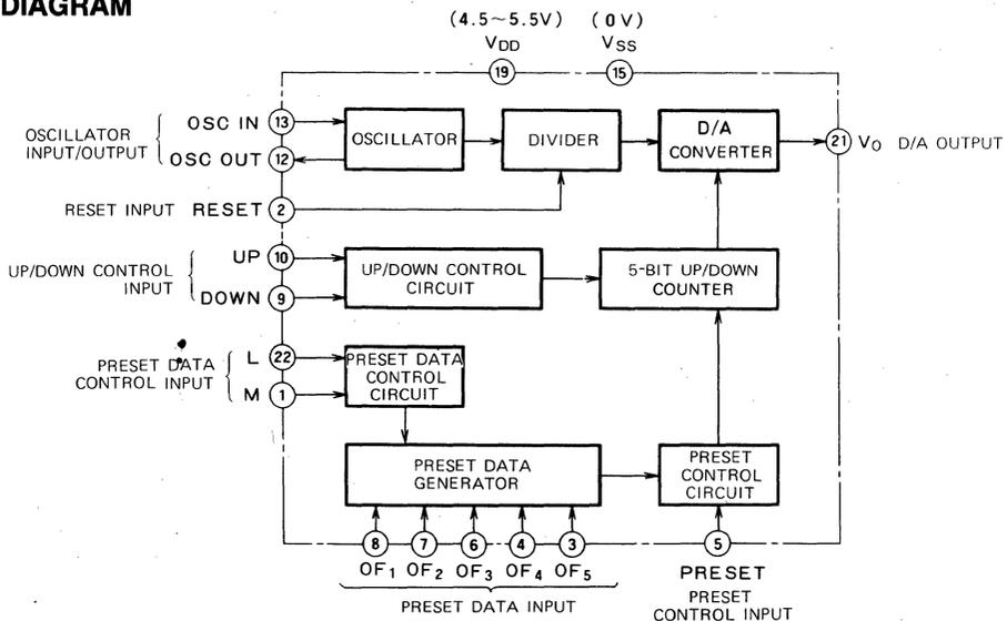
ELECTRONIC VOLUME CONTROL CMOS 5-BIT D/A CONVERTER
