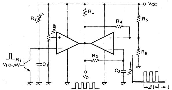
$$\Delta t = C_1 C_2 \cdot \ln \frac{V_{CC}}{V_{CC} - V_{REF}}$$
