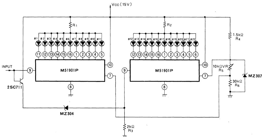
Note  $R_5$  is chosen such that the lower drive level limit for LED #12 is just 0.24V higher than higher drive level limit for LED #10.
