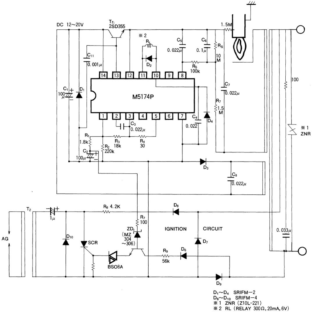
(3) FLAME DETECTOR USING A PHOTO TRANSISTOR
