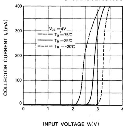
7-UNIT 400mA DARLINGTON TRANSISTOR ARRAY WITH CLAMP DIODE
