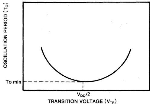
Fig. 2. Oscillation period ( $T_O$ ) VS Transition Voltage ( $V_{TR}$ )
