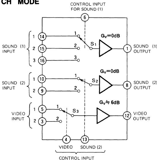
**Table 1 Switch Mode versus Control Input**
