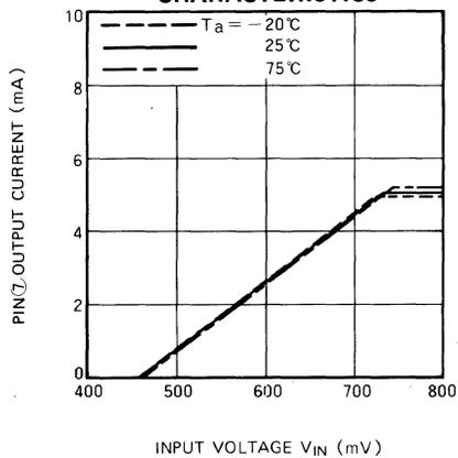
**PIN ⑧ OUTPUT CURRENT VS INPUT VOLTAGE TEMPERATURE CHARACTERISTICS**
