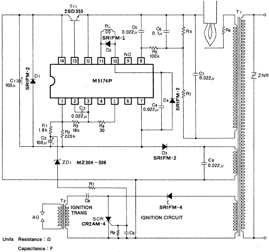
(2) FLAME DETECTOR USING FLAME CURRENT (2)
