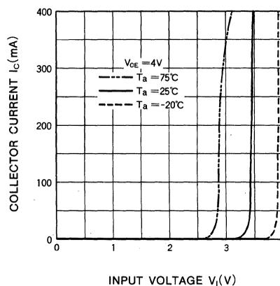
7-UNIT 400mA DARLINGTON TRANSISTOR ARRAY WITH CLAMP DIODE
