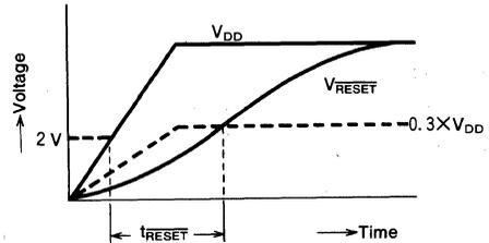
In case the power is on again after it is off and the voltage of  $\overline{RESET}$   $V_{RESET}$  is not perfectly down, the  $t_{RESET}$  must be also kept in over 1msec, which was mentioned in the above diagram. When the prescribed condition is not satisfied, add the circuit illustrated below to the  $\overline{RESET}$  and make the power-on reset function accurately. In this case, make sure to select an external capacitance to satisfy the  $V_{RESET} \geq 1$  msec.
