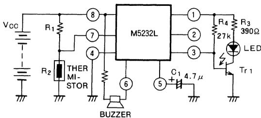
In normal circumstances the LED is set off and the current dissipation is kept down. In abnormal circumstances, the LED turn ON and OFF. It is also possible to drive a relay or indicator using a buzzer at pin (6).
