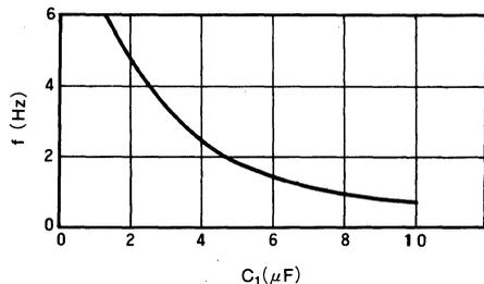
\* If the  $C_1$  capacitance is reduced to a low level, oscillation is still possible up to a frequency of about 10kHz.
