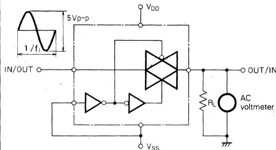
The feedthrough is taken as that frequency  $f_i$  at which, using a sine wave input of  $\pm 2.5V_{p-p}$ ,  $20 \log_{10}(V_O/V_I) = -50dB$ .
