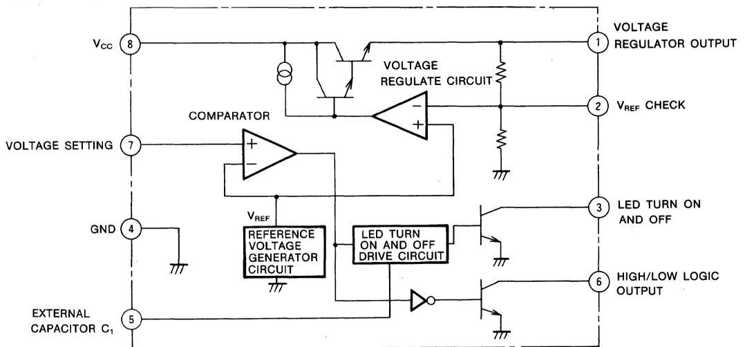
**VOLTAGE DETECTION FOR ALARM SYSTEM
