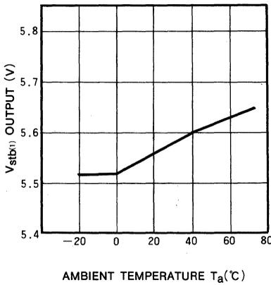
**THRESHOLD VOLTAGE OF COMP. 1 VS AMBIENT TEMPERATURE**
