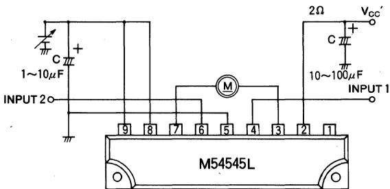
3) Motor speed control by the  $V_{CC}'$
