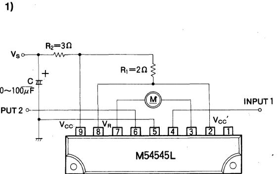
2) Motor speed control by the  $V_R$  and  $V_{CC}$
