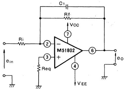
$$R_{eq} = \frac{R_f \cdot R_i}{R_f + R_i} \quad e_o = \frac{1}{R_i C_1} \int e_{in} dt$$
