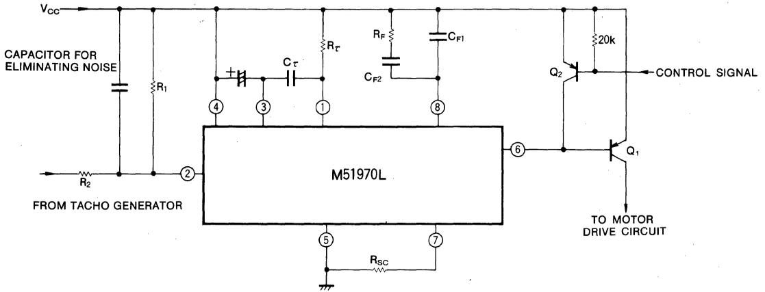
The motor is off when Q<sub>2</sub> is on.
