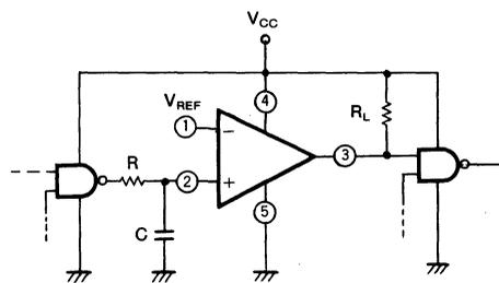
$$t_{\text{delay}} \approx 0.7CR \text{ [s]}$$
