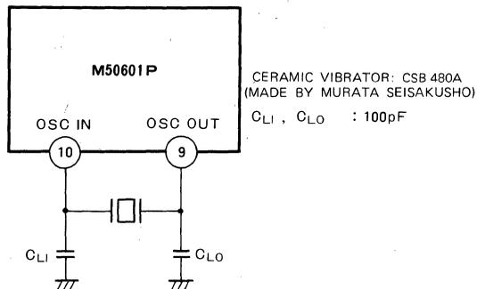
Fig. 1 Typical oscillator circuit (using ceramic vibrator)
