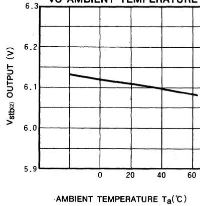
**OUTPUT VOLTAGE OF REGULATOR (1) VS AMBIENT TEMPERATURE**
