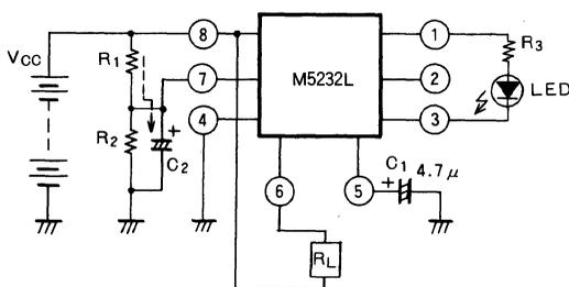
By connecting  $C_2$  in parallel with  $R_2$ ,  $V_{CC}$  is turned on, the charging current indicated by the dotted line in the figure is made to flow, and until the pin (7) voltage reaches :
