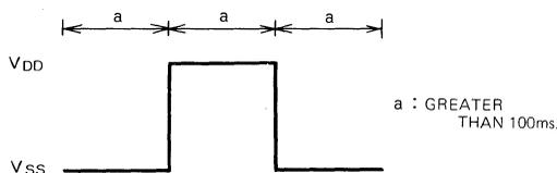
Fig. 3 L pin/M pin/PRESET pin input waveform
