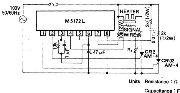
(2) THERMO CONTROLLER USING THERMISTOR (ZERO VOLT SWITCH OF SCR)
