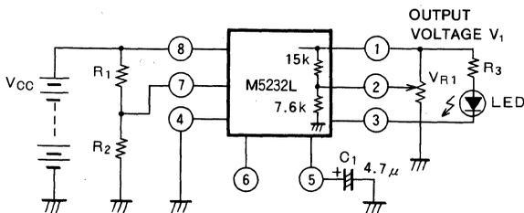
The M5232L has its output voltage  $V_1$  set by the built-in resistor, as shown in the figure, but this can be changed by connecting a semi-fixed resistor across GND and pins (1) and (2).
