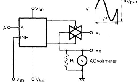
The feedthrough is taken as that frequency  $f_i$  at which, using a sine wave input of  $\pm 2.5V_{p-p}$ ,  $20 \log_{10}(V_0/V_i) = -50dB$ . Refer to the function table for conditions of control input A.
