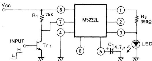
When the base of transistor  $T_{r1}$  is set low (normal), the pin (7) comparator input voltage is set high, pin (3) is set low and the LED is turned off.
