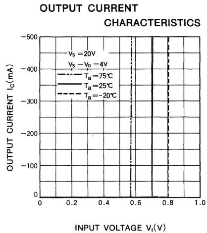
**8-UNIT 500mA SOURCE TYPE DARLINGTON TRANSISTOR ARRAY**
