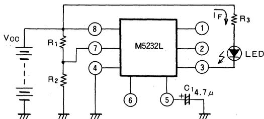
The output is not stabilized at  $V_{CC} < 5V$  since the output voltage at pin (1) of M5232L is not regulated at 4V. When an LED is connected directly from  $V_{CC}$  as shown in the figure on the left, it is possible to configure a battery checker of less than  $V_{CC} 5V$ . In this case, however, the  $I_F$  of the LED will fluctuate in accordance with the changes in  $V_{CC}$ .
