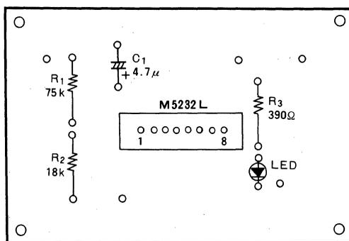
VOLTAGE DETECTION FOR ALARM SYSTEM
