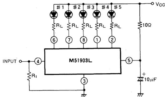
Note 1. The value of  $R_L$  is chosen to suit the LED devices to be used. The maximum LED current  $\approx (V_{CC} - \text{LED forward voltage drop} - 1.0) / R_L \leq 15\text{mA}$
