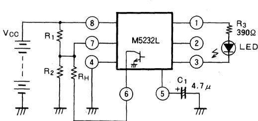
By connecting  $R_H$  across pins (6) and (7), as shown in the figure on the left, the turn ON and OFF start voltage is set at :
