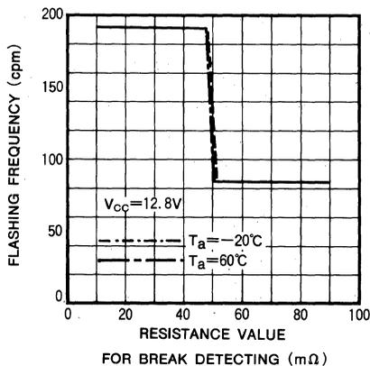
Note : 1. Flashing frequency characteristics was measured by changing the resistance value for break detecting instead of the lamp resistance used lamp; one 23W lamp
