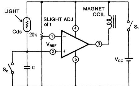
$$t \approx 0.7CR_{cds} \cdot \ln \frac{V_{CC}}{V_{CC} - V_{REF}}$$
