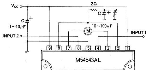
3) Motor speed control by the  $V_{CC}$
