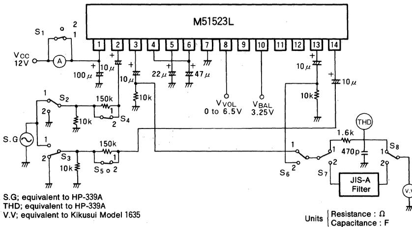
The circuit below can be substituted for JIS-A Network.
