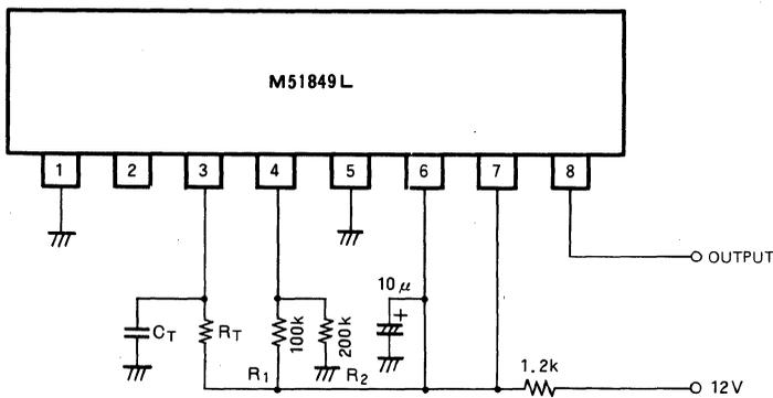
With the circuit connected as shown and it will trigger itself free run as a multivibrator.
