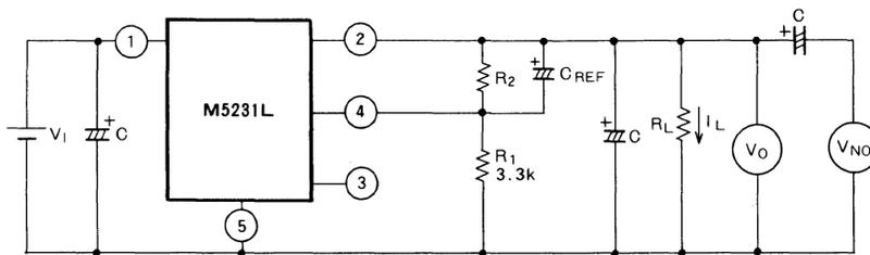
**(b) Ripple rejection test circuit**
