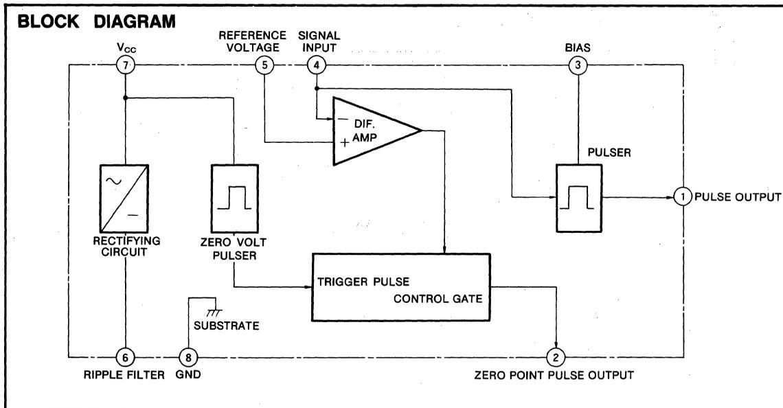
\* CAPACITOR MUST BE CONNECTED BETWEEN PIN 6 AND GND.
