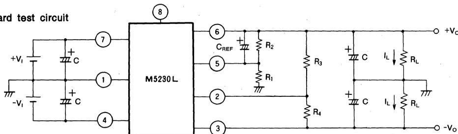
$$+V_O = V_{REF} \left(1 + \frac{R_2}{R_1}\right) \approx 1.8 \times \left(1 + \frac{R_2}{3.3}\right) (V)$$
