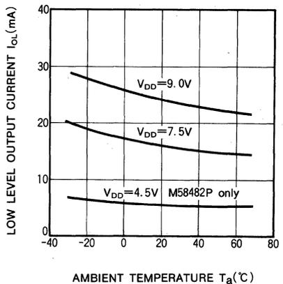
(5)  $I_{OL}-T_a$  (OUT 1, OUT 2, OUT 3)  $V_{OL}=0.4\text{V}$
