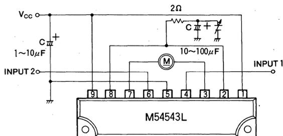
3) Motor speed control by the  $V_{CC}$
