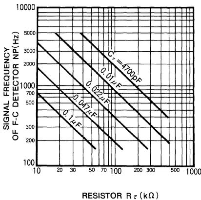
$R_r \cdot C_r$  determine the speed of motor
