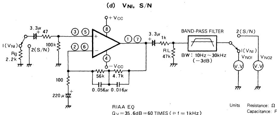
1.  $V_{NI} = V_{NO1} / 60$  ( $\mu\text{Vrms}$ )
