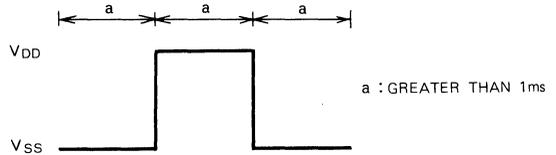
Fig. 2 L pin/M pin/PRESET pin input waveform.
