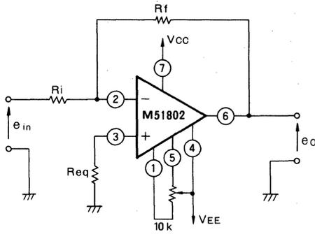
$$R_{eq} = \frac{R_f \cdot R_i}{R_f + R_i} \quad A_{vo} = \frac{R_f}{R_i}$$
