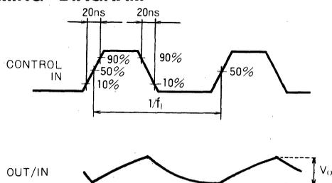
$f_{max}$  ( $C_{IN}$ ) is taken as that frequency  $f_i$  at which the output amplitude  $V_O$  is 1/2 that at kHz.
