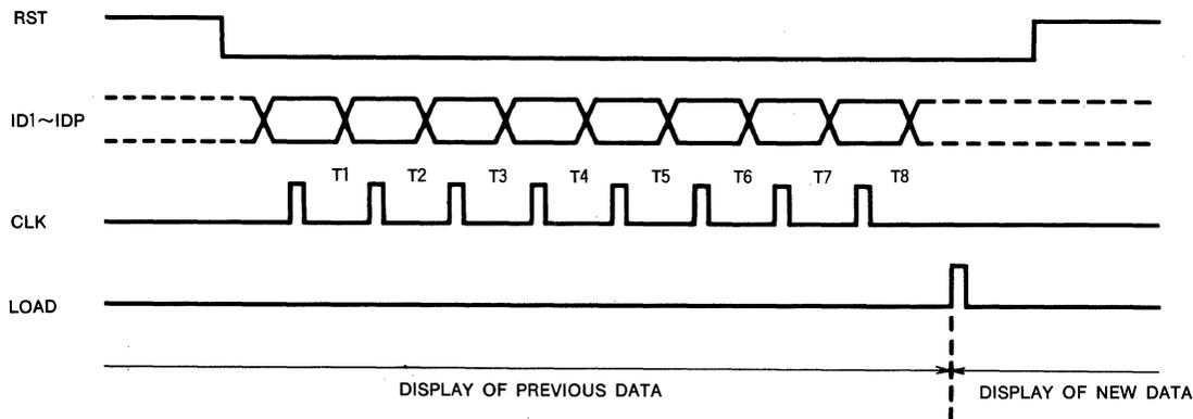
After the 8th clock input, the LOAD is valid only in the period while RST="L". Furthermore, if there is 9th CLK input before the LOAD input, the LOAD input is ignored.
