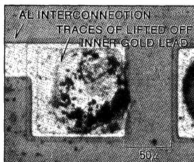
**Fig. 3** Lift off of inner gold lead (analyzed using a metallurgical microscope)
