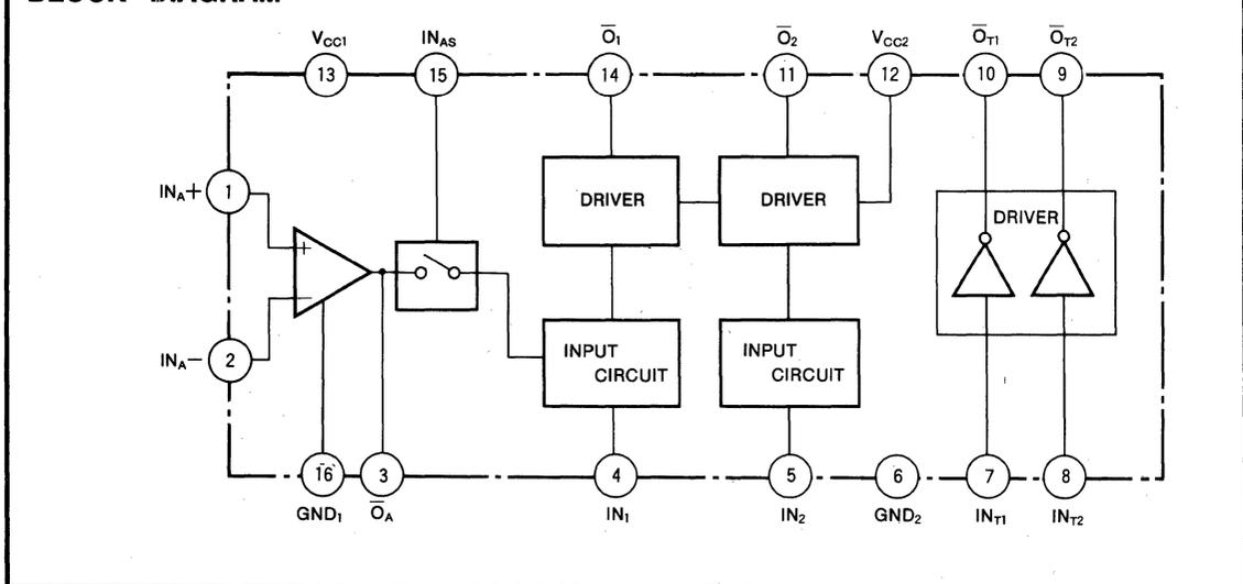
**BI-DIRECTIONAL MOTOR DRIVER WITH OP AMP AND TRANSISTOR ARRAY**
