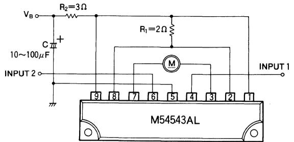
2) Motor speed control by the  $V_{CC'}$
