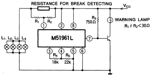
The warning lamp is on when one or more lamps of the four break.
