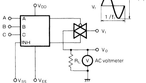
The feedthrough is taken as that frequency  $f_i$  at which, using a sine wave input of  $\pm 2.5V_{p-p}$ ,  $20 \log_{10}(V_O/V_i) = -50\text{dB}$ . Refer to the function table for conditions of control inputs A, B, and C.
