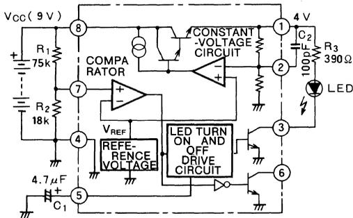
This is a battery reduced voltage checker which is set so that the LED starts turn ON and OFF when the voltage drops by 25% ( $V_{CC}=6.8V$ ) of the supply voltage ( $V_{CC}=9V, 1.5V \times 6$ ).  $C_1=4.7\mu F \rightarrow f \approx 1.8Hz$
