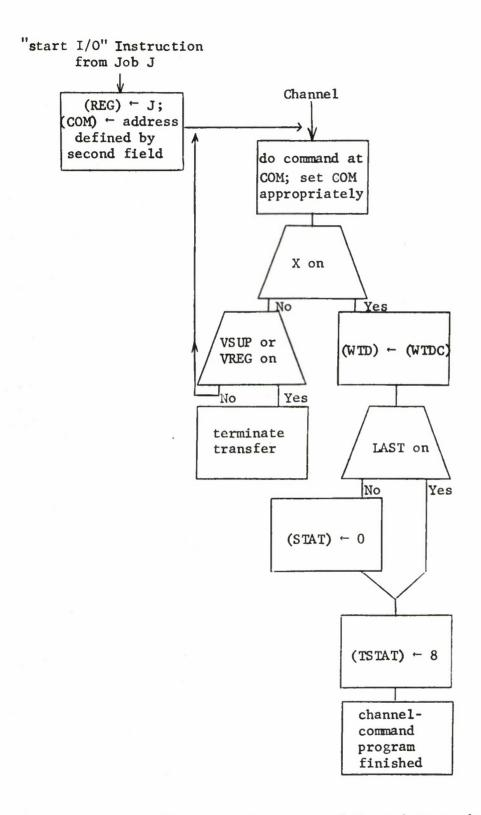
Figure 4. Execution of Channel Commands
