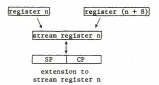
Figure 1. The Relationship between Registers, Stream Registers and Extensions
