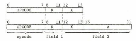
The opcode is 8 bits long. The first field, R, is 4 bits long  $ew^3$  usually contains the number of a general register. The second field is either 4 bits long or 20 bits long. If it is 4 bits long, it contains the number, X, of a general register and the instruction is called a short instruction. A short instruction is written:
