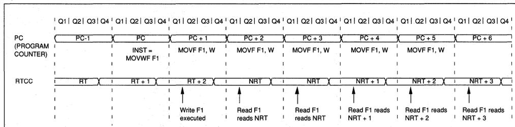
**FIGURE 4.2.2B - RTCC TIMING: INT CLOCK/PRESCALE 1:2**
