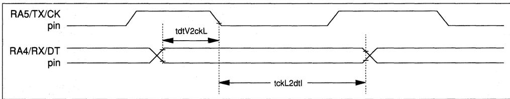
FIGURE 12.4.13: I/O PORT INPUT/OUTPUT TIMING (PORTA, PORTB)
