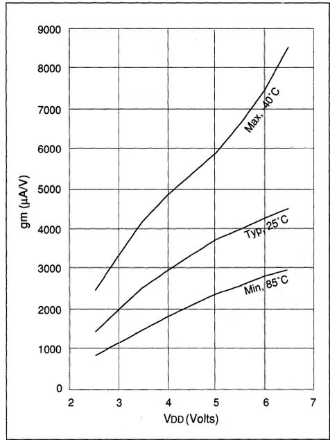
FIGURE 9.0.16 - Transconductance (gm) of LP Oscillator vs VDD
