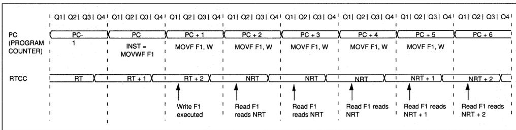
FIGURE 6.4.3 - RTCC TIMING: INT CLOCK/PRESCALE 1:2
