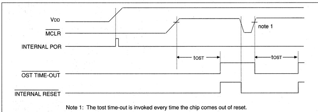
**FIGURE 13.1.6 - USING ON-CHIP POR (FAST VDD RISE TIME)**
