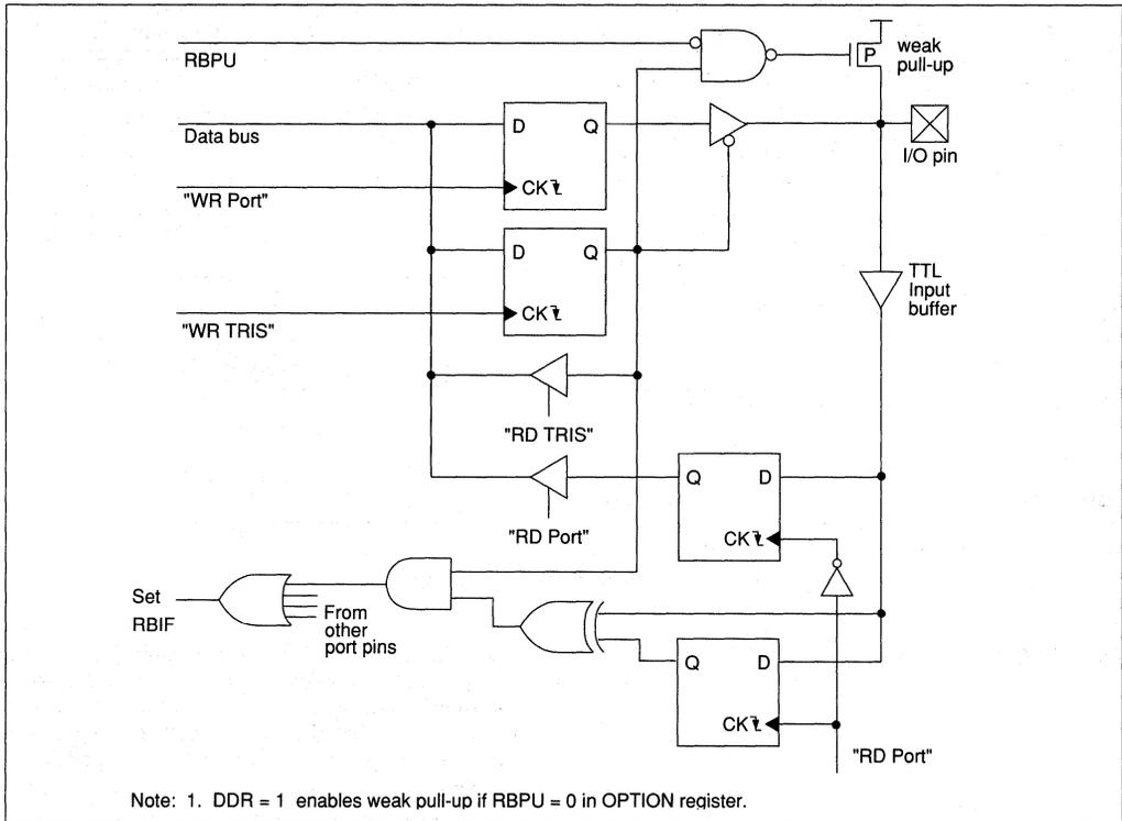
**FIGURE 6.2.2 - BLOCK DIAGRAM OF PORT PINS RB<3:0>**
