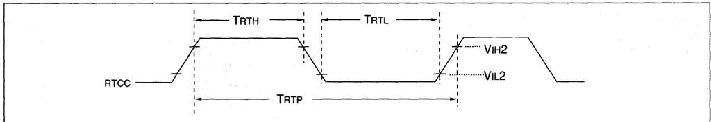
**FIGURE 8.0.2 - OSCILLATOR START-UP TIMING (PIC16C71RC)**
