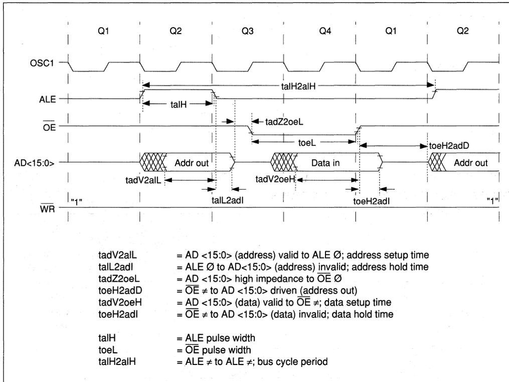
FIGURE 12.4.2: TIMING DIAGRAM - EXTERNAL PROGRAM MEMORY WRITE
