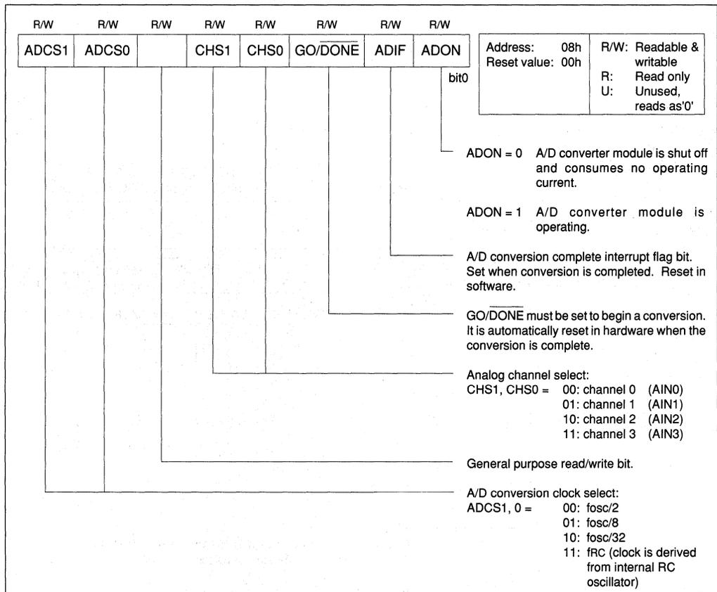
FIGURE 6.6.2 - A/D CONTROL REGISTER (ADCON1, ADDRESS 88h)
