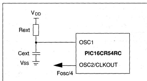
**FIGURE 13.1.1 - EXTERNAL POWER ON RESET CIRCUIT**
