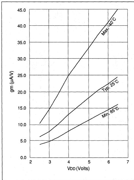
FIGURE 9.0.17 - Transconductance (gm) of XT Oscillator vs VDD
