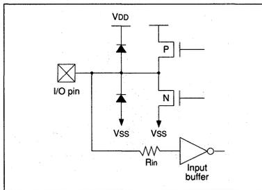
FIGURE 16.9.2 - ELECTRICAL STRUCTURE OF MCLR AND RTCC PINS
