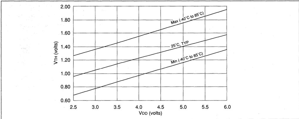
**FIGURE 18.0.8 - V<sub>IH</sub>, V<sub>IL</sub> OF MCLR, RTCC AND OSC1 (IN RC MODE) vs V<sub>DD</sub>**
