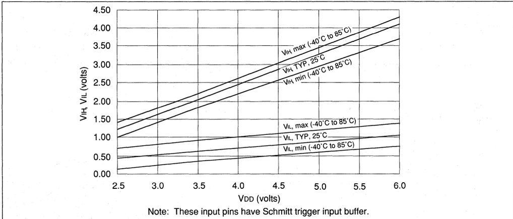
**FIGURE 18.0.9 - V<sub>TH</sub> (INPUT THRESHOLD VOLTAGE) OF OSC1 INPUT (IN XT, HS, AND LP MODES) vs V<sub>DD</sub>**
