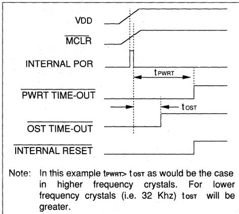
FIGURE 4.4.6: INTERNAL RESET (VDD AND MCLR TIED TOGETHER): SLOW VDD RISE TIME
