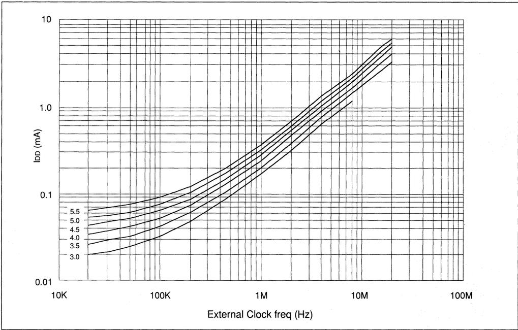
FIGURE 9.0.13 - MAXIMUM I<sub>DD</sub> vs FREQ (EXT CLOCK, -40° to +85°C)
