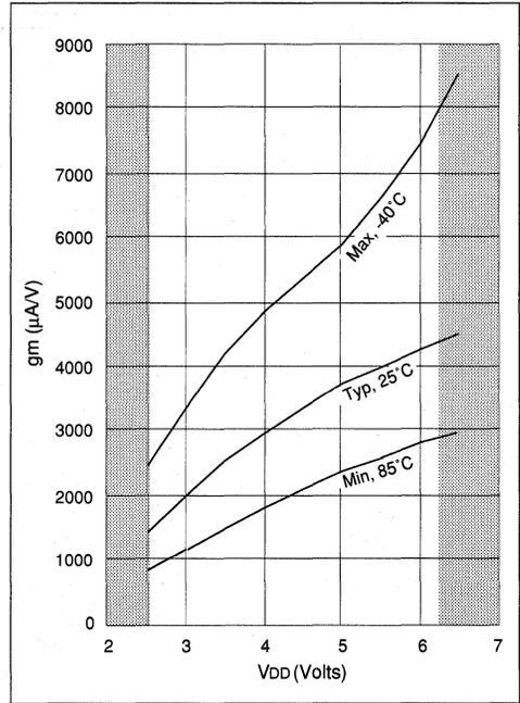
**FIGURE 18.0.14 -Transconductance (gm) of LP Oscillator vs VDD**
