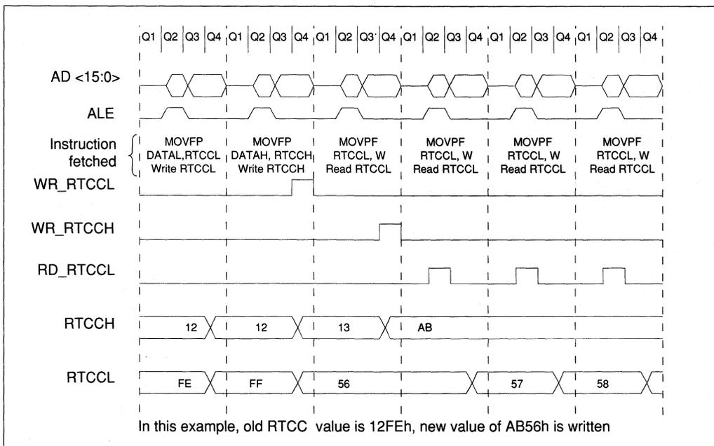
FIGURE 8.2.3.1: RTCC TIMING WITH EXTERNAL CLOCK
