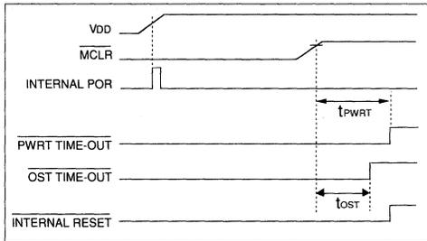
FIGURE 4.4.4: USING ON-CHIP POR
