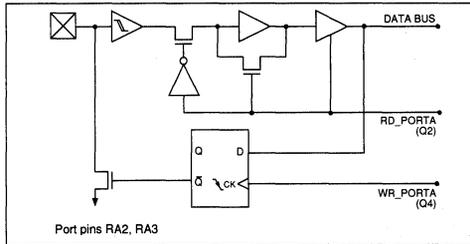
FIGURE 6.1.1: PORT A BLOCK DIAGRAMS
