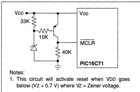
**FIGURE 5.2.6 - BROWN OUT PROTECTION CIRCUIT 2**
