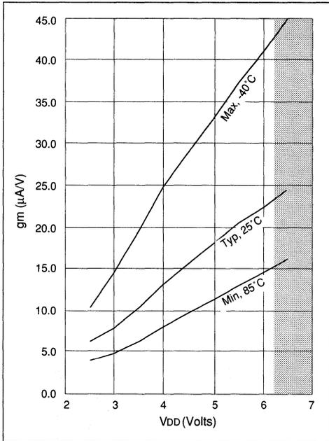
**FIGURE 18.0.18 - Transconductance (gm) of XT Oscillator vs V<sub>DD</sub>**
