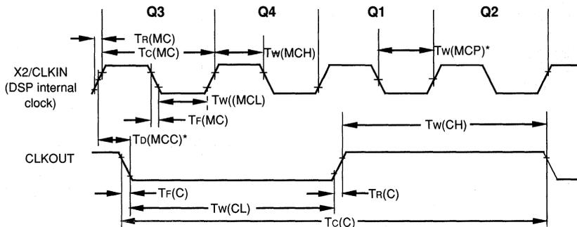
\* TD(MCC) and TW(MCP) are referenced to an intermediate level of 1.5 volts on the CLKIN waveform.
