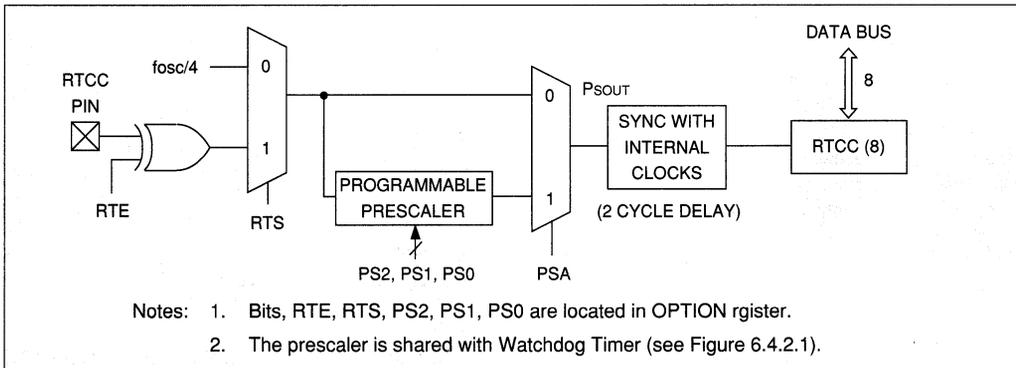
FIGURE 6.4.2 - RTCC TIMING: INT CLOCK/NO PRESCALE
