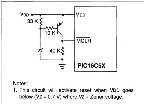
**FIGURE 13.1.3 - BROWN OUT PROTECTION CIRCUIT**
