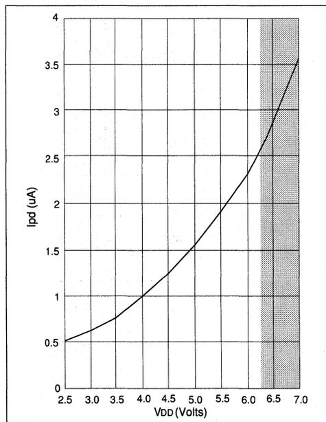
**FIGURE 18.0.6 - TYPICAL I<sub>pd</sub> vs V<sub>DD</sub> WATCHDOG ENABLED 25°C**
