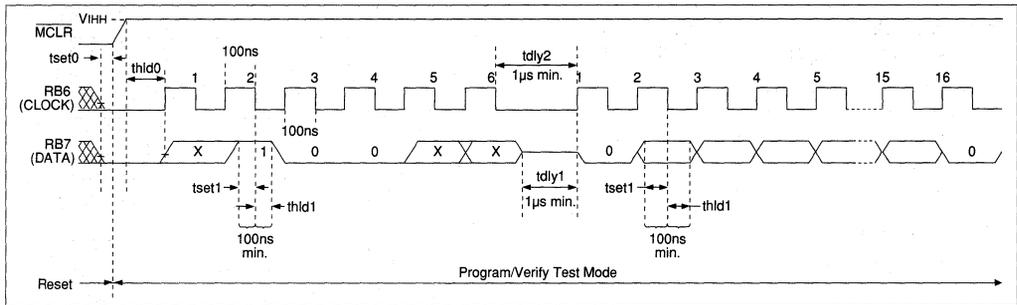
FIGURE 11.4.3.1 - READ DATA COMMAND (SERIAL PROGRAM/VERIFY)
