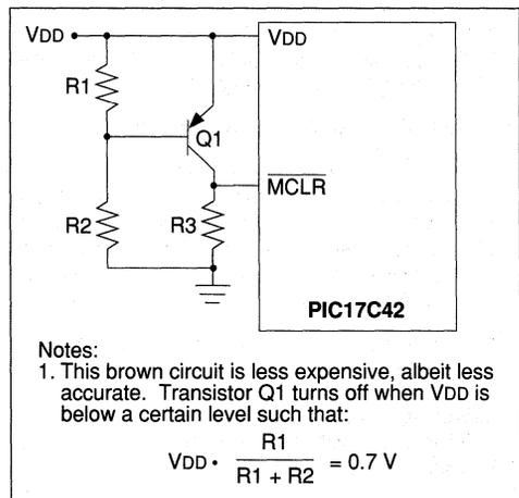
FIGURE 4.4.3: EXTERNAL RESET PULSE
