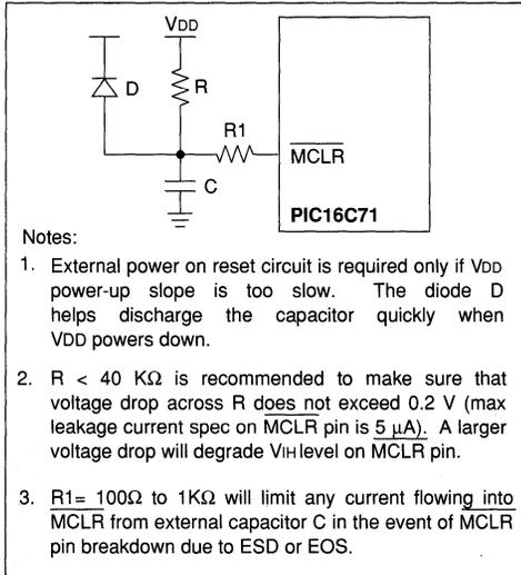
**FIGURE 5.2.5 - BROWN OUT PROTECTION CIRCUIT 1**
