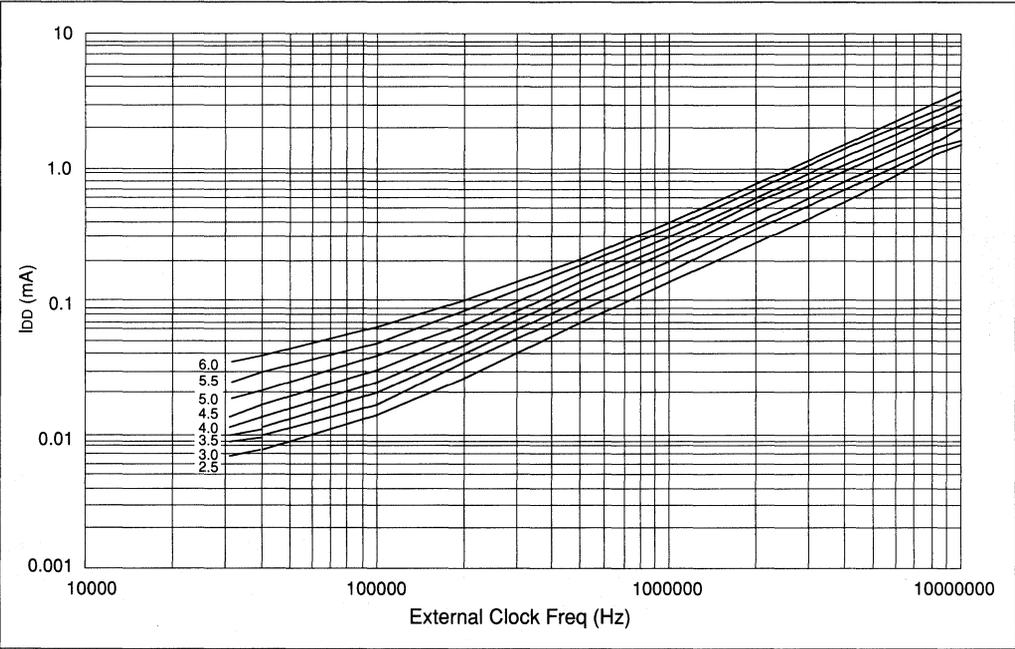
FIGURE 18.0.11 - MAXIMUM I<sub>DD</sub> vs FREQ (EXT CLOCK, -40°C TO +85°C)
