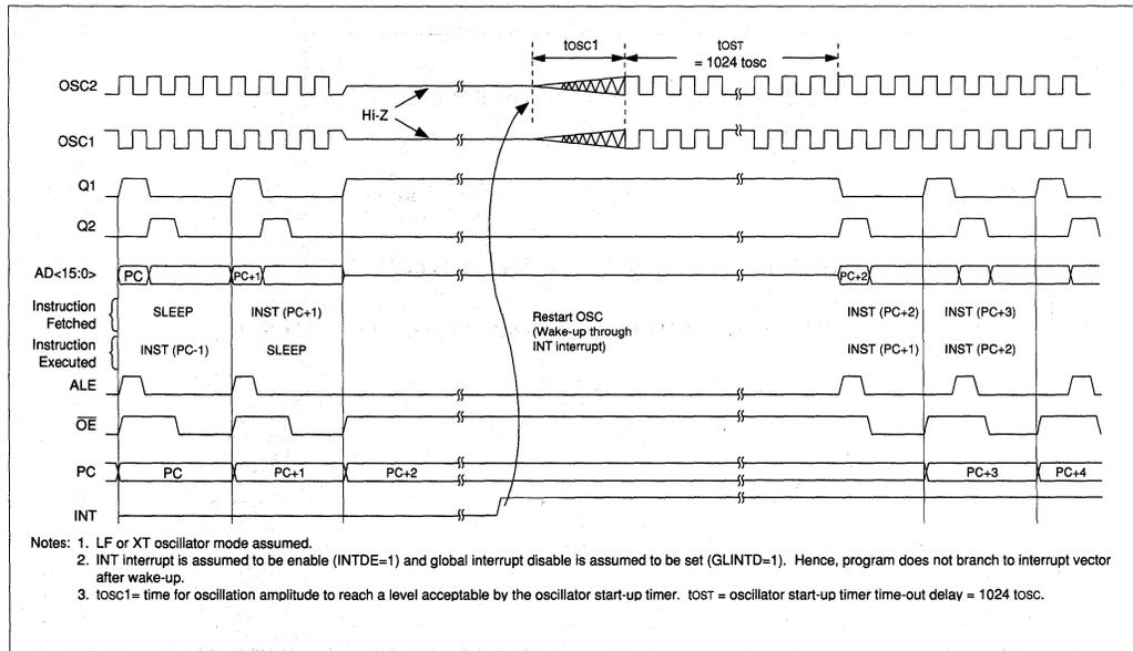
FIGURE 12.4.10: SLEEP/WAKE-UP THROUGH INT (RC MODE)
