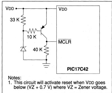
FIGURE 4.4.2: BROWN OUT PROTECTION CIRCUIT
