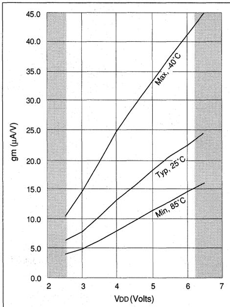
**FIGURE 18.0.15 -Transconductance (gm) of XT Oscillator vs VDD**
