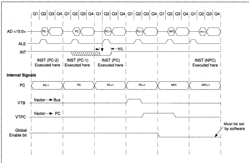
**FIGURE 12.4.4: RESET TIMING**
