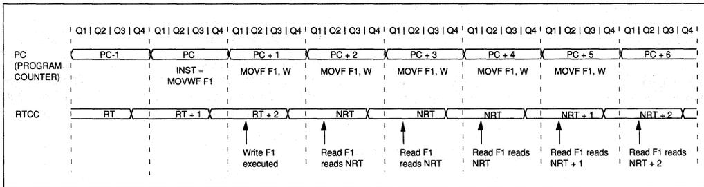
**FIGURE 4.2.2B - RTCC TIMING: INT CLOCK/PRESCALE 1:2**
