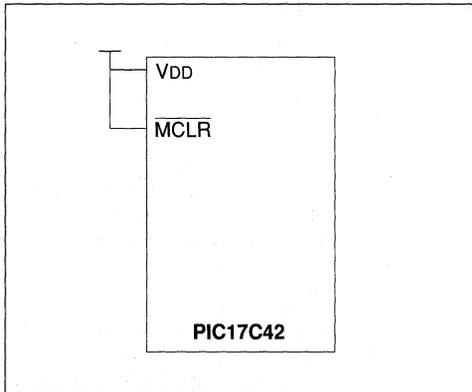
FIGURE 4.4.5: INTERNAL RESET (VDD AND MCLR TIED TOGETHER)
