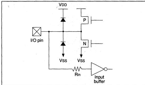
**FIGURE 7.6.2 - ELECTRICAL STRUCTURE OF MCLR AND RTCC PINS**
