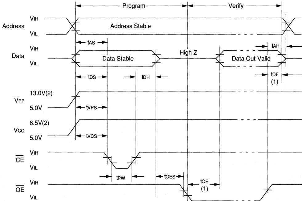
Notes: (1) tDF and tOE are characteristics of the device but must be accommodated by the programmer
