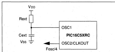
**FIGURE 13.1.1 - EXTERNAL POWER ON RESET CIRCUIT**
