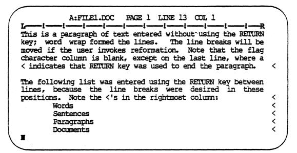
Figure 2-7. Appearance of Text on the Screen
