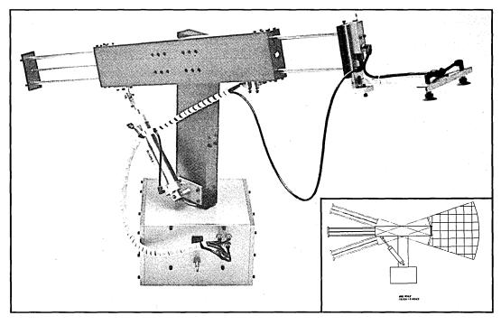
Figure 1 — BR 100 Series Pick and Place Robotic Arm.
