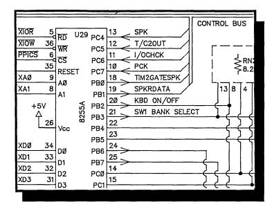
At last you can plumb the mysteries of your computer with this single sheet schematic of the IBM XT's main board. A wealth of information for both True Blue and clone owners.
