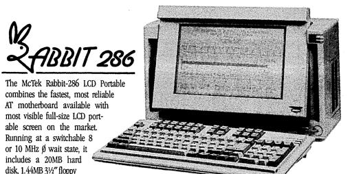
drive, parallel & serial ports, Award 3.03 bios, 640k & turbo indicator LCD. The screen is a fantastically readable, electroluminescently backlit, 80-column by 25-line, high
