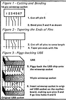
I also used a wirewrap socket to take care of the U86 modifications for the speed-up. I bent up pins 4 and 5 on a 14-pin socket and soldered the leads from the speed switch to them. Then (as above) I shortened and filed all the pins, put U86 into the new socket, and put the assembly back into the original U86 socket.
