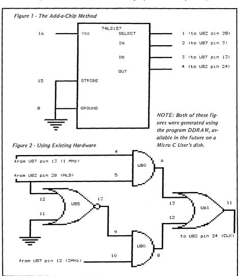
multiplexer, using leftover gates on your Kaypro circuit board. You'll need to cut six traces and then add eight wires. You won't need to bend out any with this method. The trace cutting requires precision and dexterity; read before attempting. See Figure 2.
