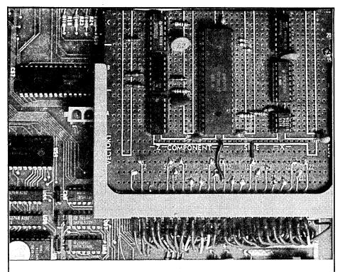
New disk controller card mounted on flexible leads on the Xerox 820-II motherboard. The card plugs into a 44 pin socket which is wired to the J12 connector pads.
