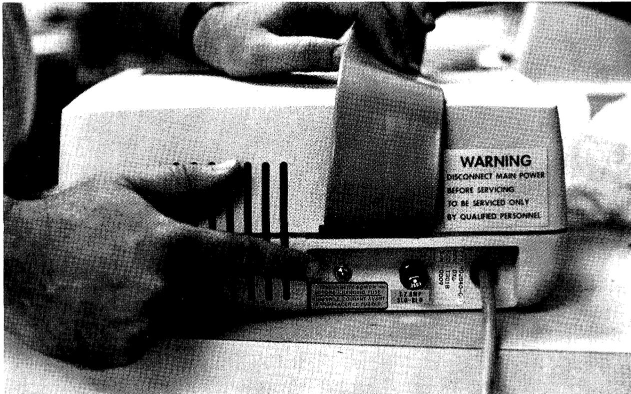
Figure 3-11. Tape cartridge drive power switch
