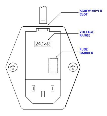
FIGURE 2.2.2 SUPPLY VOLTAGE SETTING
