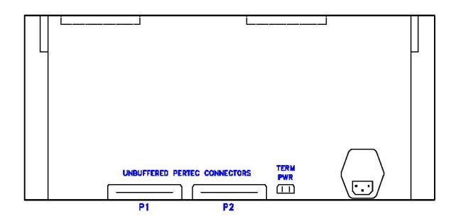
FIGURE 2.6.2 (a) CONNECTOR LOCATIONS, UNBUFFERED PERTEC
