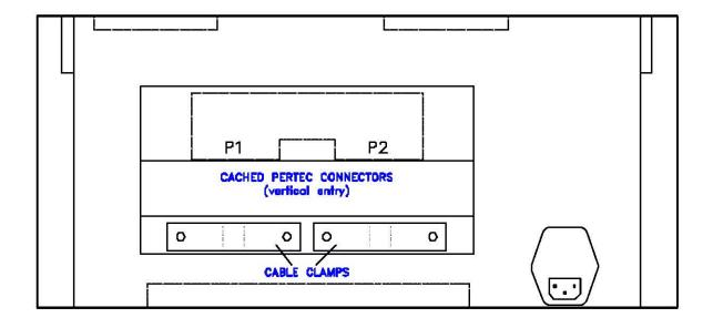
FIGURE 2.6.2 (b) CONNECTOR LOCATIONS, CACHED PERTEC
