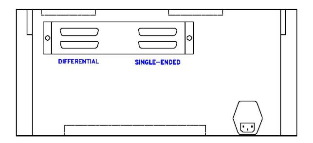
FIGURE 2.6.1 (a) SCSI CONNECTOR LOCATIONS, RACK-MOUNTED MODELS
