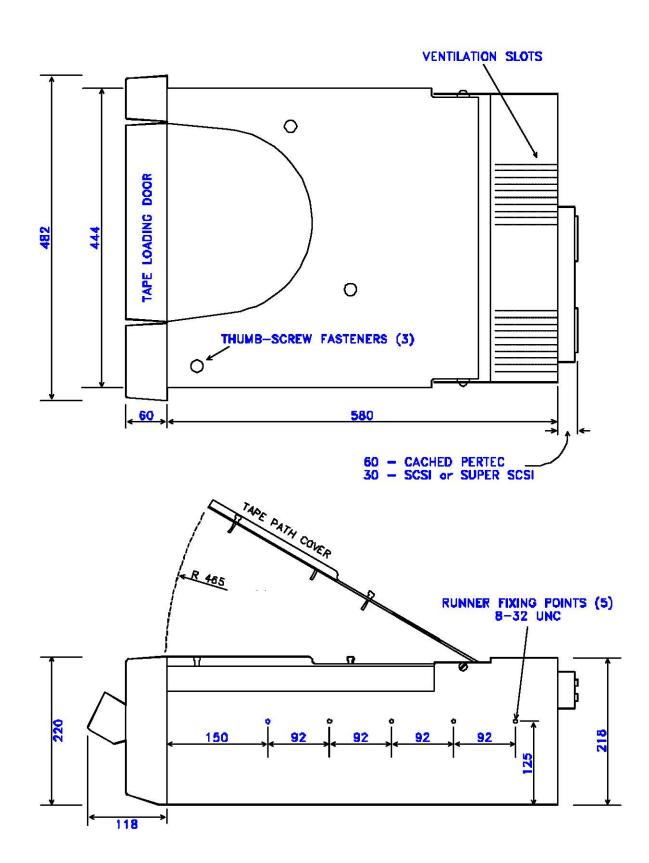
FIGURE 2.3(b) 9914 RUNNER FIXING POINTS
