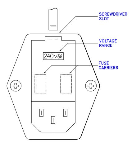
FIGURE B.1.2 VOLTAGE SETTING (I.T. MAINS)
