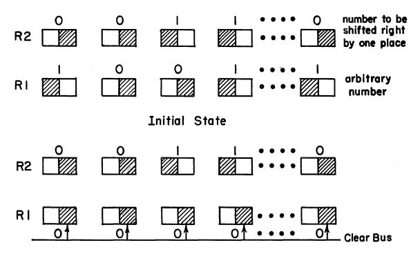
Step 1. Clear RI to ZEROS by voltage pulse on Clear Bus. Symbol = Co RI
