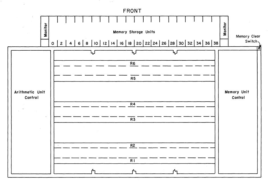
The display neons for the various registers have not been brought out to the panel but are physically located with their register. They are readily visible from the operating panel table. In line with this, the monitor tubes for visible memory display are mounted in the memory rack rather than on the operating panel (See Figures 2 and 3).
