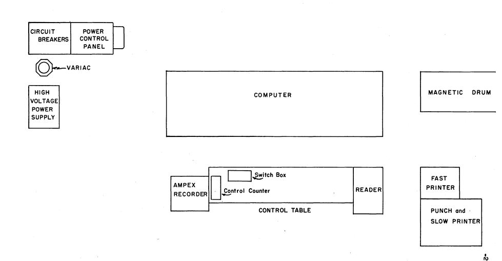
FLOOR LAYOUT of COMPUTER and AUXILIARY EQUIPMENT
