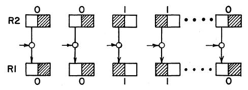
Step 2. Flip-flops of R2 containing "I" cause corresponding flip-flops of RI to set to "I" when voltage pulse is applied to gate tubes.
