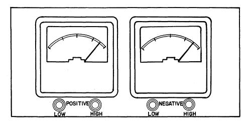
GENERATOR VOLTMETER PANEL - POWER SUPPLY
