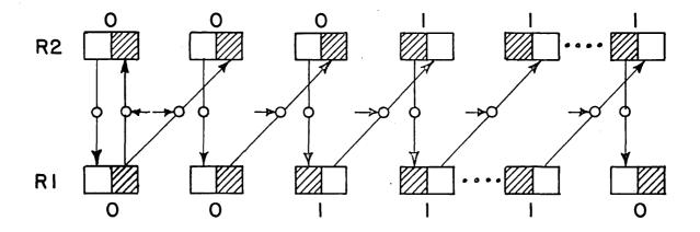
Step 4. Flip—flops of RI containing "O" cause corresponding flip-flops of R2 to set to "O".
