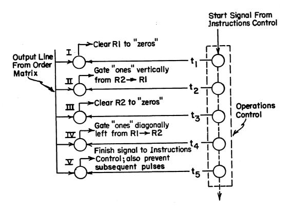
Fig. 9 Gate connections for a simplified order.
