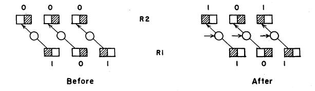
R2 is cleared to 0's. When these gates are opened, the information in R1 is transferred to R2 displaced once to the left. Thus, by these sequences of operations, a number originally in R2 is shifted one place to the left.
