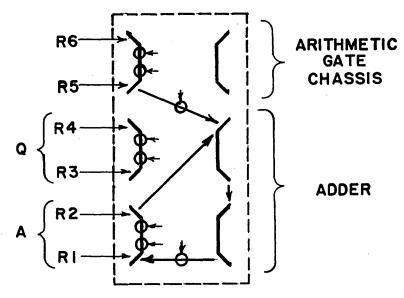
Fig. 1 Schematic Cross-Section of Arithmetic Unit. Circles with the small arrows indicate gate tubes, or electronic switches. Also shown are the interconnections for the addition process.
