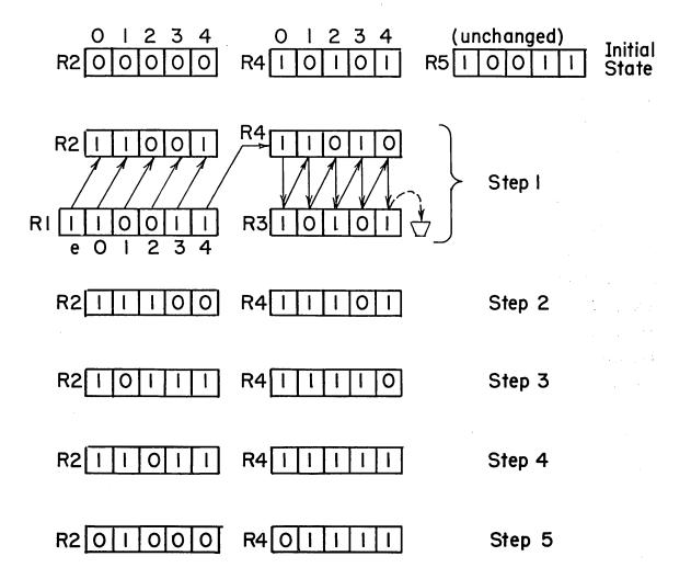
At the end of Step 4 the iterative procedure is completed, and the sign of the multiplier is by now at the extreme right flip-flop. Step 5 is a true addition of the complement of the multiplicand, inasmuch as the multiplier is negative. Simultaneously R4 is shifted to the right by one so that the right half of the final product is properly positioned. For reasons of uniformity OR4 is always set to 0 in this step, irrespective of the true sign of the product.
