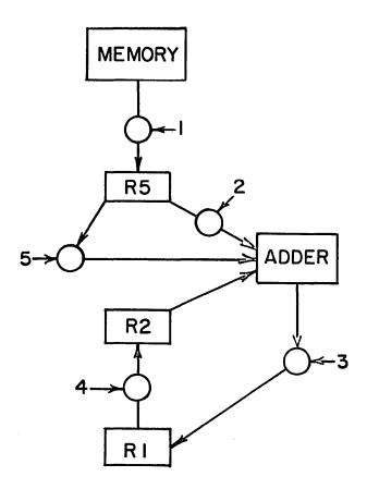
Fig. 4 Schematic cross-section of the arithmetic unit that participates in the addition process. As usual, circles indicate gate tubes. The small arrows represent symbolically the signals that stimulate the gating action. The clearing actions associated with each gating action are not shown.
