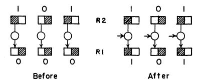
Rl has been previously cleared to 0's. The information in R2 is 101. When an appropriate voltage change is applied to the gate tubes, the first flip-flop of Rl will change its state to represent a 1, the second remains unchanged, and the third behaves like the first. Rl will then have received the information 101.
