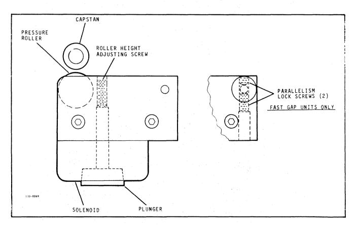
Figure 5-2. Pinch Roller Adjustments
