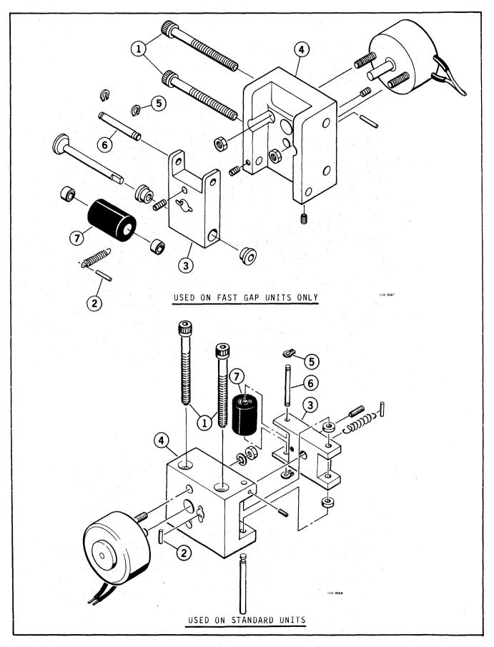
Figure 5-4. Pinch Roller Replacement
