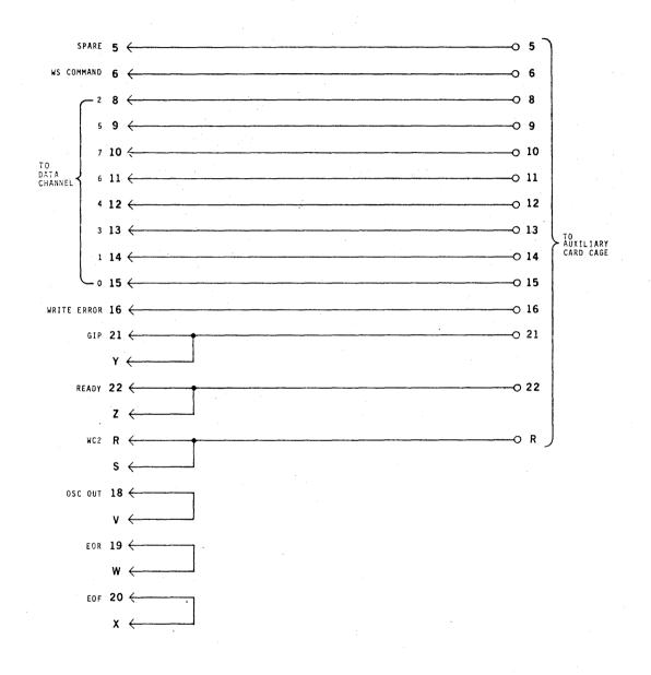
Interface, Type 2569-001A, Schematic Diagram
