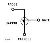
The SUS conducts at an anode voltage of about 7 volts if the gate terminal is open. Once fired the device continues to conduct until current drops below a threshold value.
