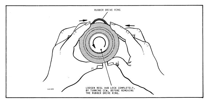
Figure 5-5 Rubber Ring Drive Replacement
