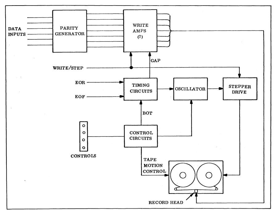
Figure 1-1. Incremental Recording System
