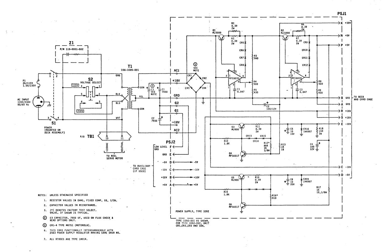
Power Supply Regulator, Type 3392-001 Schematic Diagram
