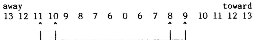
This example has jitter. The display will not remain stationary, and we can not see exactly how far the R/W head is off track centerline. One unit of jitter would be all right, but here you see two units of jitter. Something is wrong with the motor, drive belt, or shaft bearings. You may need to replace the drive. But sometimes the jitter may be caused by EMF noise that enters the electronics of either the drive or the computer.
