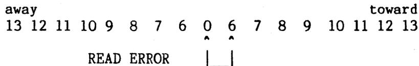
Here is a very bad example of the radial reading. The read quality is very bad and sometimes the READ ERROR message shows. However, the R/W head maybe only slightly toward the spindle. There is no way to read radial displacements between 0 and 6.
