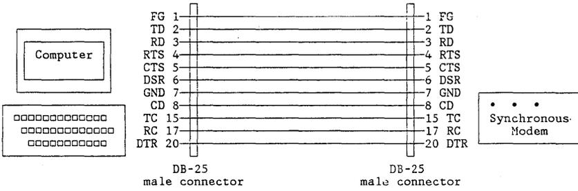
**Figure 6.1 Connecting the Microcomputer to a Modem**
