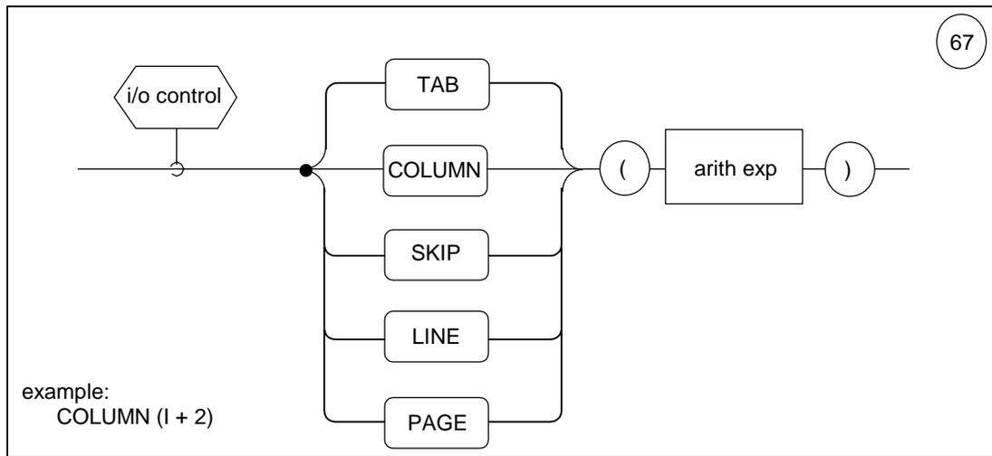
**Figure 10-3 i/o control function - #67**
