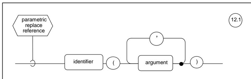
**Figure 4-4 parametric replace reference - #12.1**
