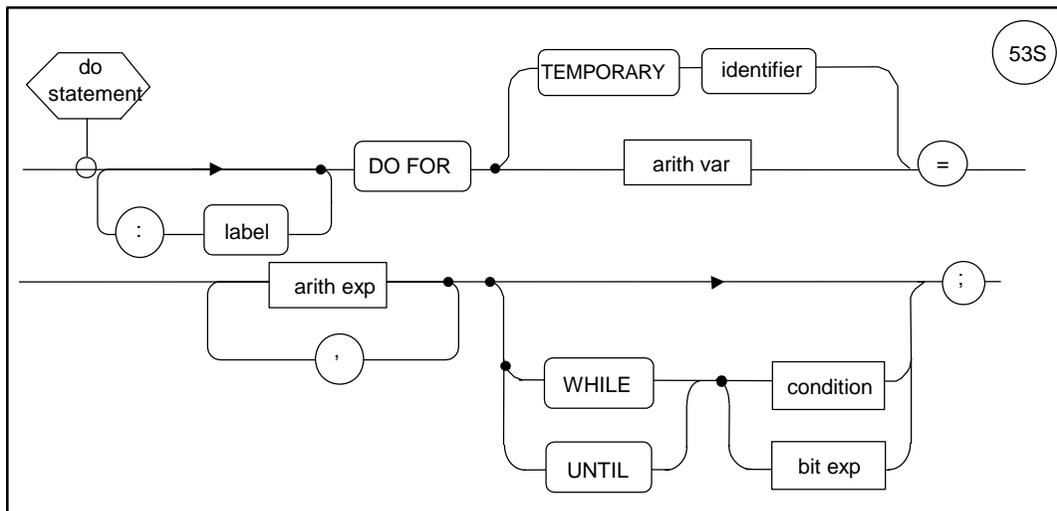
**Figure 11-10 discrete DO FOR with loop TEMPORARY variable index - #53**
