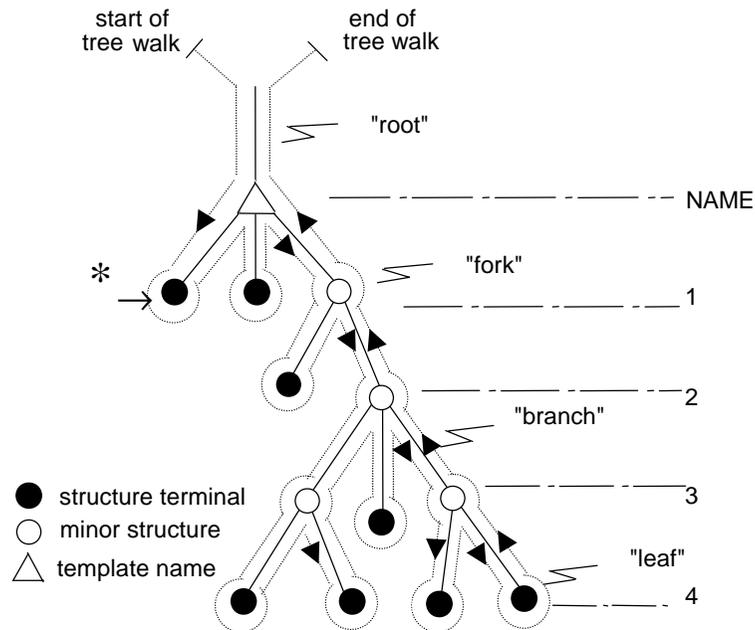
**Figure 4-6 Tree diagram for a typical structure template**
