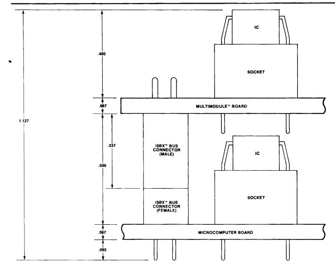
Figure 2-2. Mounting Clearances (Inches)
