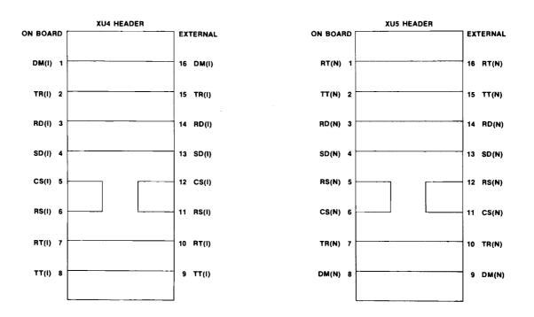
Figure A-5. Master Header Wiring Diagram
