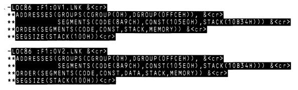
The CGROUP and DGROUP base address must be specified in order to compute offset information. The final base address assigned to DGROUP by LOC86 will be rounded down to 0FFC0H.
