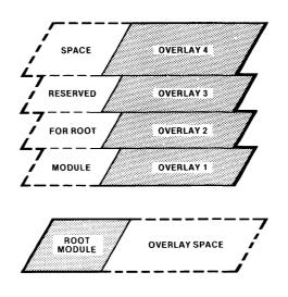
Figure 1-7. Memory Configuration of Program with Overlays 639-7
