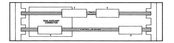
Figure B-2. ICE<sup>™</sup> Boards in Dual Auxiliary Connector
