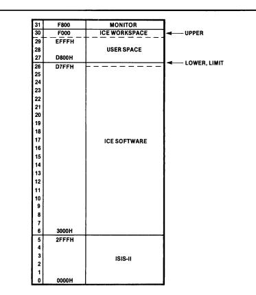
Figure 5-2. Memory Allocation for Dual-ICE85/4X<sup>™</sup>
