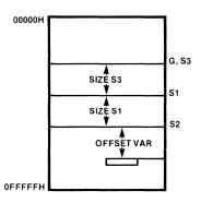
The value of OFFSET G:VAR will include the sum of the size of S3, the size of S1, and OFFSET S2:VAR, but this sum must be adjusted for the align-types and ending points of S3, S2, and S1.
