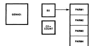
Example 4 below shows how this process can be written in the 8086 assembly language. GENAD returns the sum in the accumulator. It receives the address of the array in the BX register, and the number of array elements in CX.
