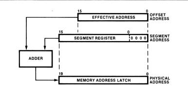
The 8086 memory can be thought of as an arbitrary number of segments. A byte or word within a segment is addressed with a 16-bit offset address. The 8086 automatically adds the offset address to the shifted 16-bit segment address, creating a 20-bit physical address.
