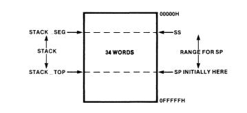
Note that the length of the combined segment is 34 words, the sum of the lengths of the pieces; but that the top-of-stack variables "stack\_top" and "top\_stack", whose names are local to each module, are assigned the same offset (68D = 44H bytes) at the high end of memory. You can set the stack segment base and the stack pointer by the instructions (in module 1):
