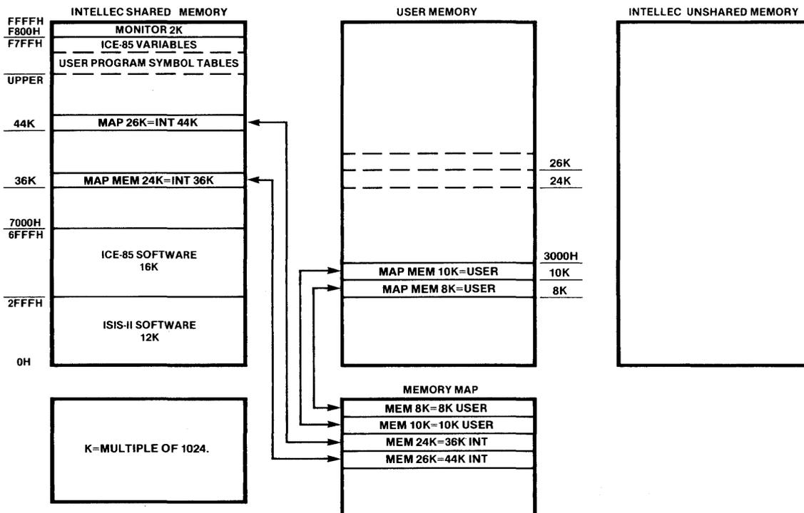
Figure 5-5. Mapping Into User and Shared Intellec Memory
