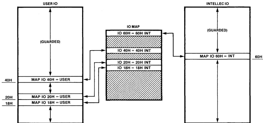
Figure 5-7. IO Port Segments Mapped to User and Intellec
