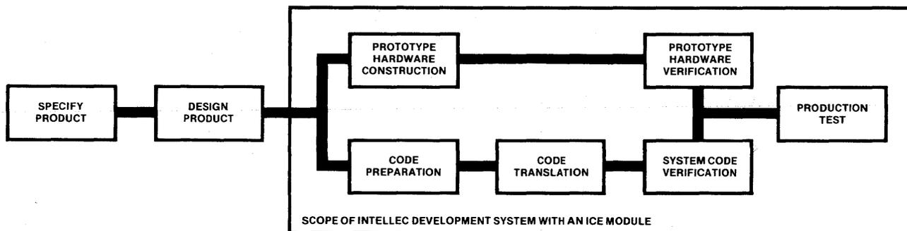
Figure 1-5. Typical Development Cycle with ICE Module
