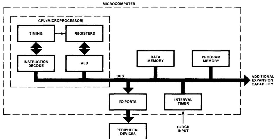
Figure 1-1. Logical Blocks in a Microcomputer System
