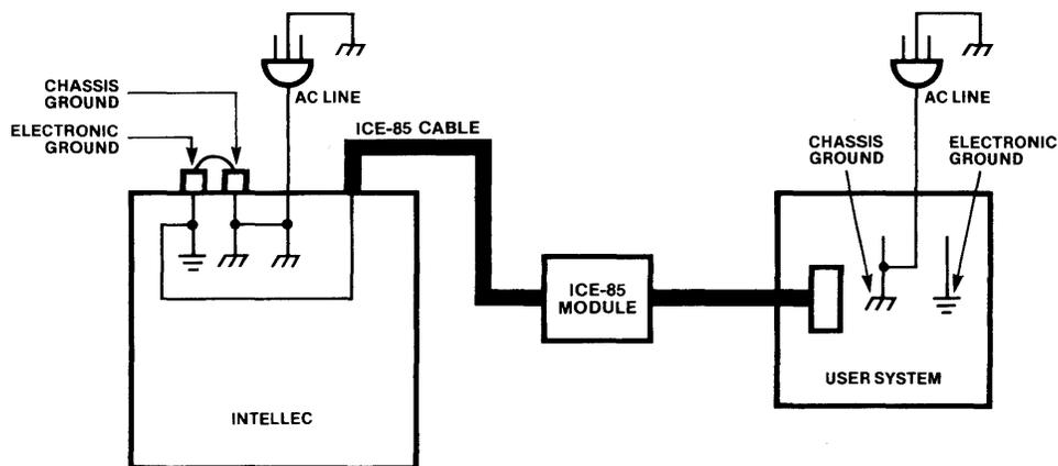
Figure 2-3. System Grounding for Intellec Series I
