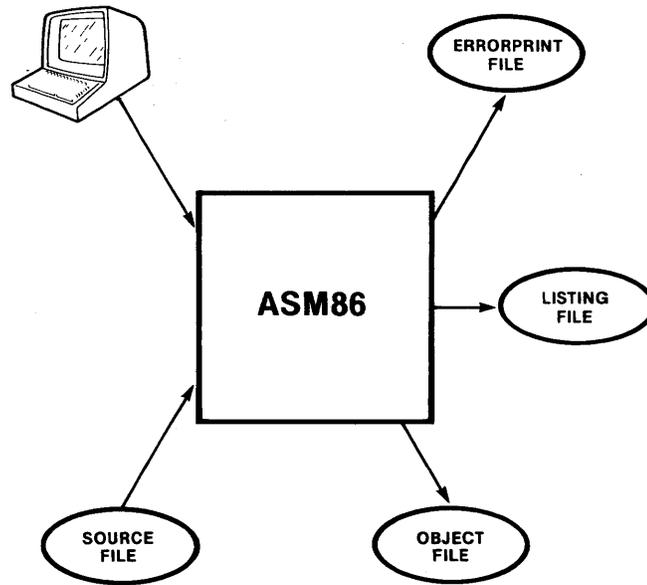
Figure 1-1. ASM86 Macro Assembler Logical Files
