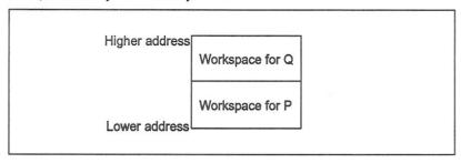
In a PAR or PRI PAR construct the last textually defined process is allocated the lowest addressed workspace. For example:
