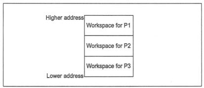
In a replicated PAR construct the instance with the highest replication count is allocated the lowest workspace address. For example:
