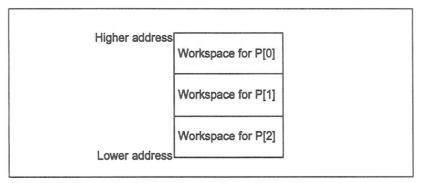
Unless separate vector space is disabled, most arrays are allocated in a separate data space, known as vector space, see section B.1.4. The allocation is done in a similar way to the allocation of workspace, except that the data space for a called procedure is at a *higher* address than the data space of its caller.
