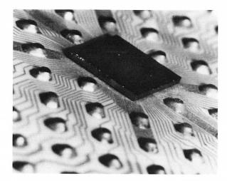
Figure 3 Closeup of mounted chip
