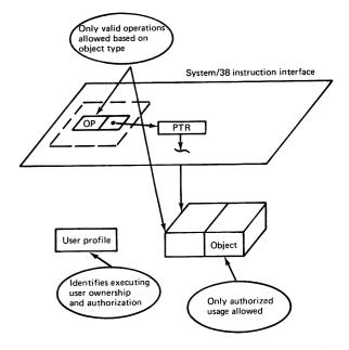
Figure 2 System/38 instruction interface integrity and authorization scheme
