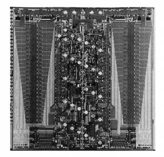
Figure 4 64K-bit array chip
