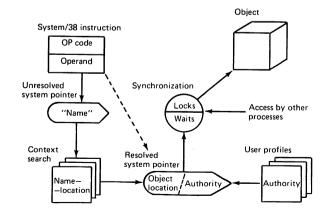
Figure 2 The object access path
