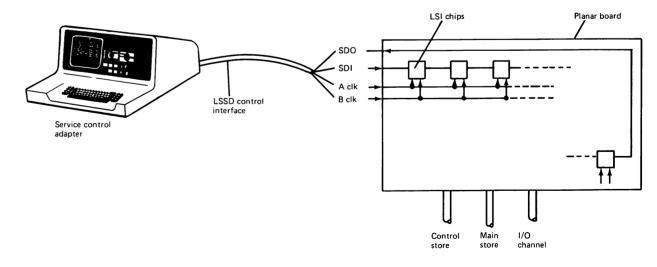
Figure 3 System/38 planar board and interfaces
