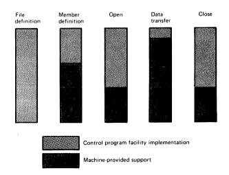
Figure 1 System/38 data base facility functional distribution
