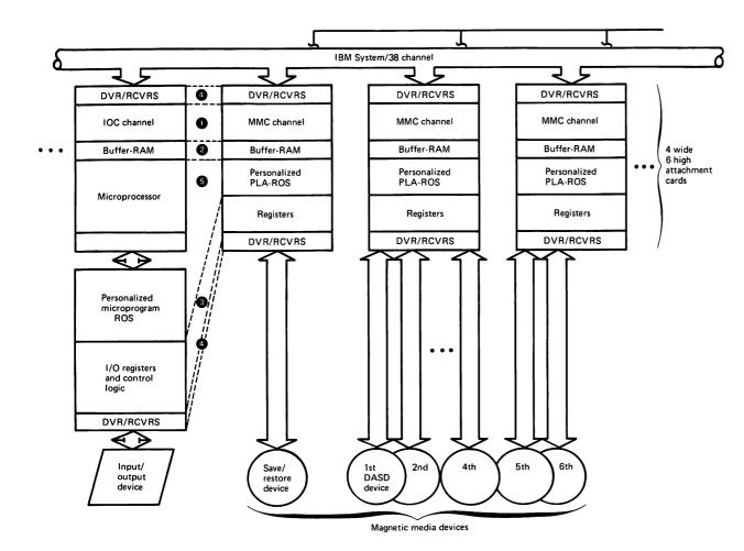
Figure 1 System/38 device attachments
