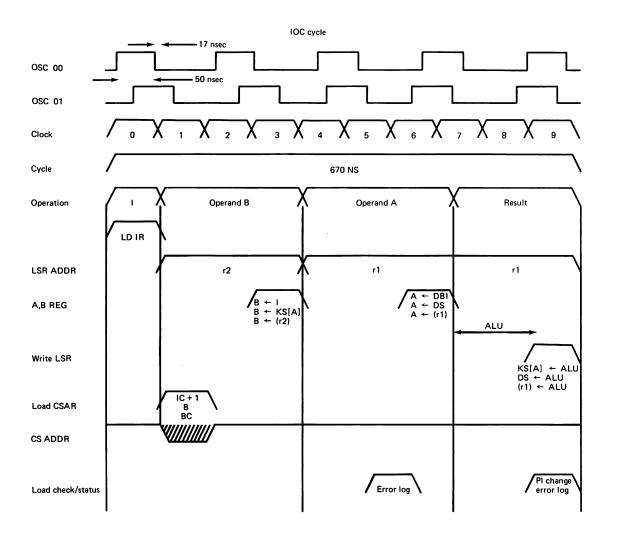
Figure 2 Operand register/destination sources
