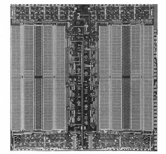
Figure 3 32K-bit array chip
