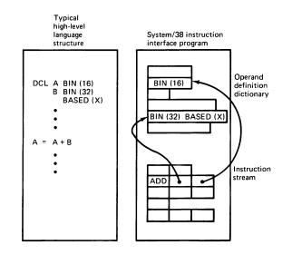
Figure 3 System/38 instruction interface program structure
