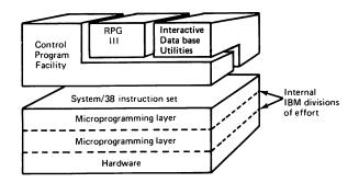
Figure 3 The total structure of System/38
