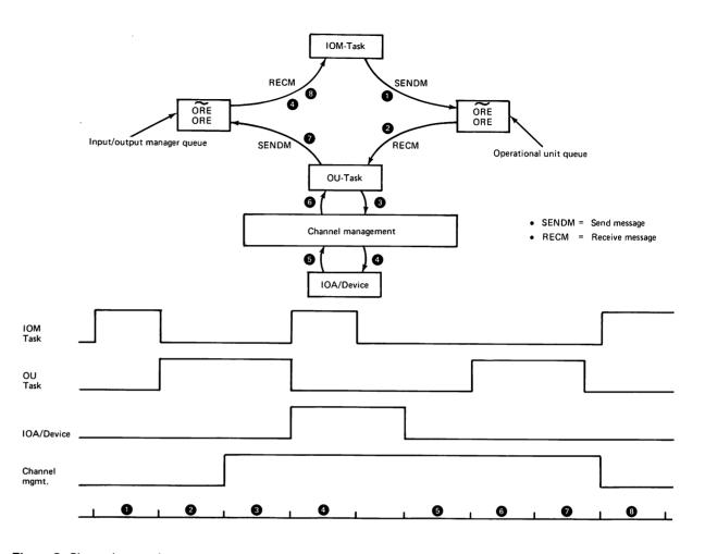
Figure 2 Channel operation
