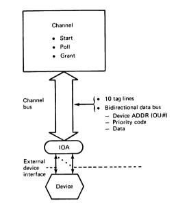
Figure 3 Channel dialog with device
