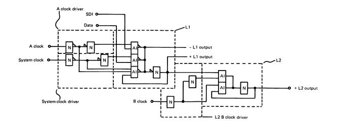
Figure 2 Shift register latch
