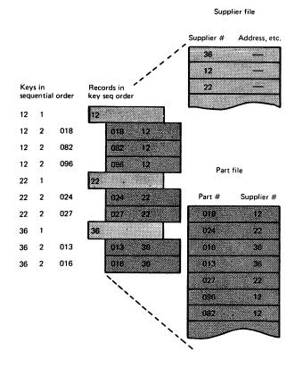
Figure 2 Use of keys in forcing logical hierarchical ordering
