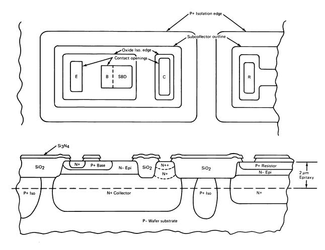
Figure 1 Top and section drawing of transistor, Schottky barrier diode, and resistor
