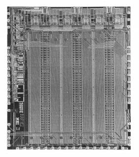
Figure 2 18K-bit array chip
