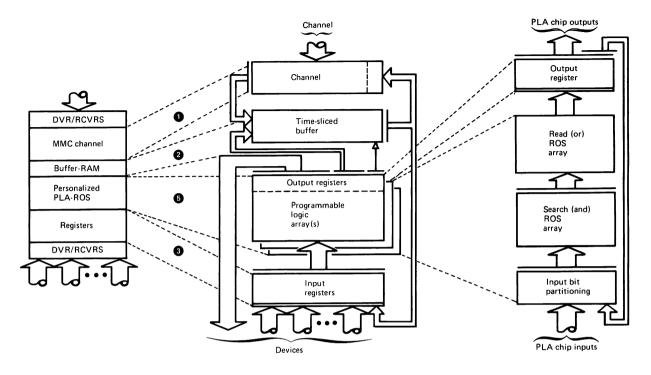
Figure 2 Magnetic media controller—functional data flow
