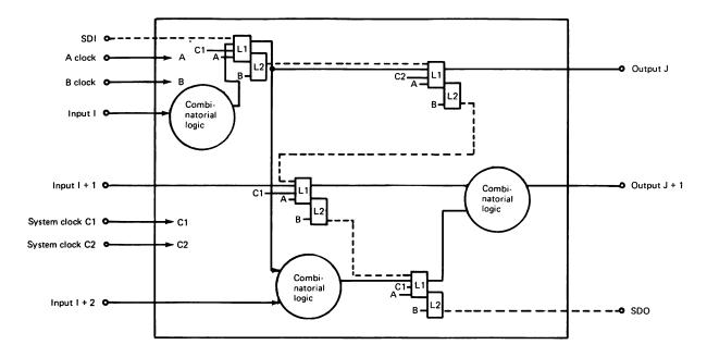
Figure 1 Typical LSSD LSI chip
