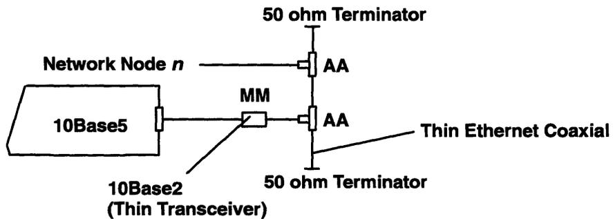
**Note:**  $n$  is a maximum of 30 nodes per segment (maximum of five segments connected by a repeater).
