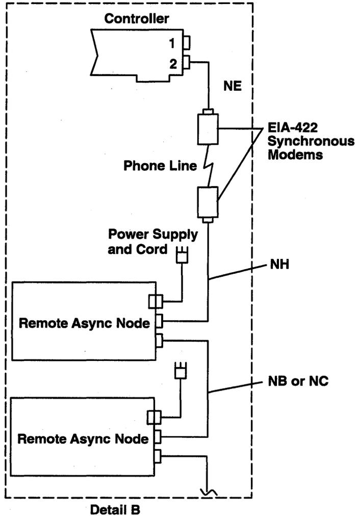
A choice of cables can be attached to any of the 16 Remote Async Node ports, as shown in the following illustration. These ports are labeled 0 through 15 and accept 4-, 6-, 8-, and 10-pin RJ-type connectors.
