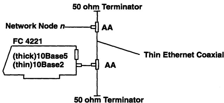
**Note:** *n* is a maximum of 30 nodes per segment (maximum of five segments with each segment connected by a repeater).
