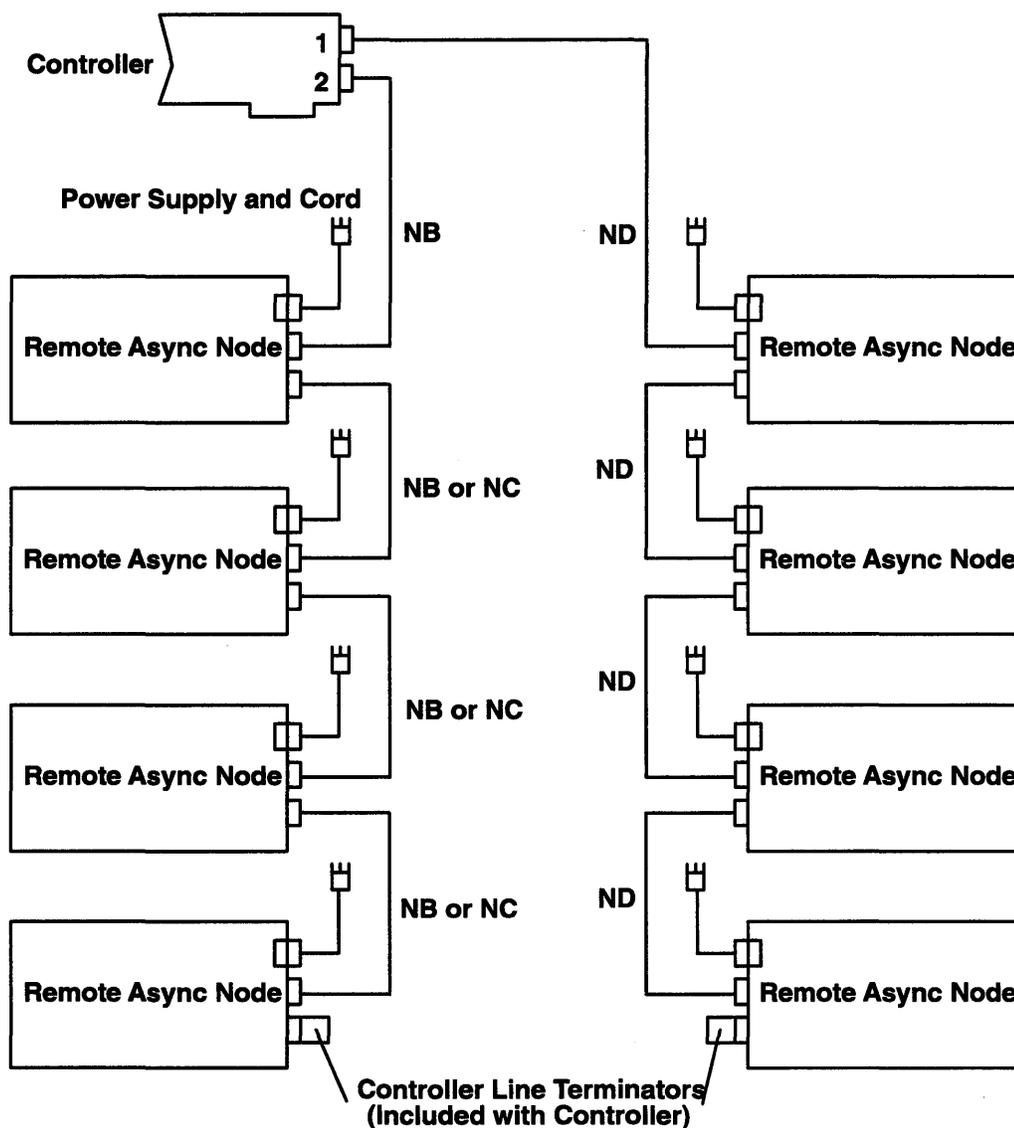
The 128-Port Async Controller supports up to four Remote Async Nodes on each controller line using the following attachment options:
