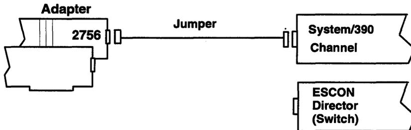
**Note:** The ESCON jumper cable can connect to any ESCON channel, trunk, or ESCON director.
