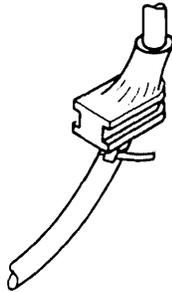
4. Lubricate the cable with wire pulling compound, and slide the grommet over the cable. Pull at least 150 mm (6 in.) of cable through the grommet.
