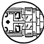
11. Position the bushing so that the flanges on the front are over the grounding towers in the back of the connector. Press the bushing into the back of the connector.
