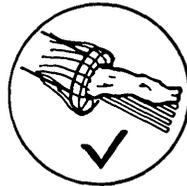
2. Fan out the braid and fold it back over the strain relief washer.
