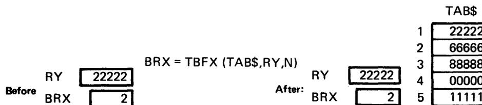
The search begins at index 3. After index 4 and 5 are searched and no equal entry is found, I125 and I127 are set on and the operation terminates.
