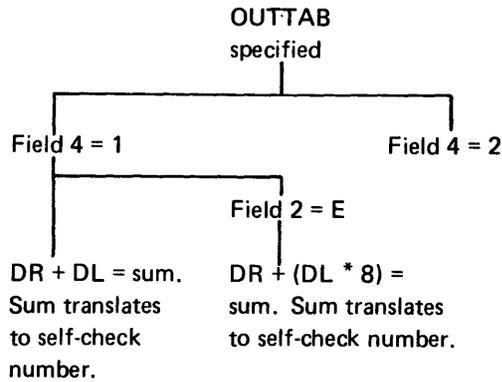
The output translate table is usually used if the modulus is greater than 10 and there is a single self-check digit. The 5280 uses the value of the DR or the DR and the DL to determine the byte of the output translate table that contains the character to insert into the self-check register.
