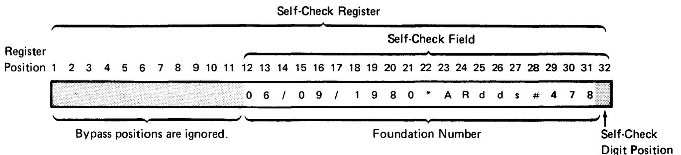
Figure 2-4. A Self-Check Field in a Decimal Double Register
