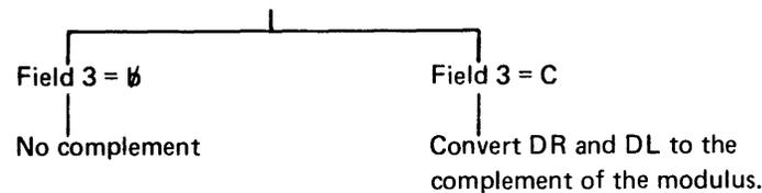
If Field 3 is blank, no complement is taken. If Field 3 is C, the DR and DL are taken to the complement of the modulus. This has the effect of subtracting the modulus value from the DR and DL value.
