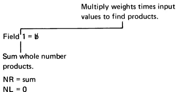
If Field 1 is blank, the input value is multiplied by the weight for each foundation position, and the whole number products are added. The sum is used for the NR, and the NL is forced to 0.
