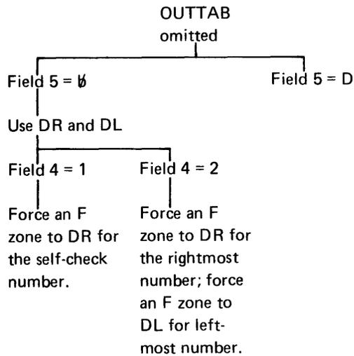
If no output translate table is specified, and Field 5 of the CNTL parameter is blank, both the DR and DL are used to determine the self-check number output.
