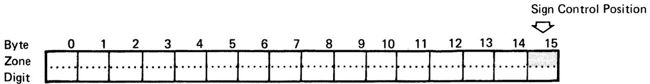
Figure 1-4. The Sign Control Position in a Decimal Register
