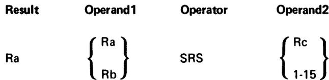
The bytes of the operand1 register are shifted right the number of bytes indicated by operand2, and the shifted result is placed into the result register. The high-order bytes of the result register contain zero (hex F0) for the number of bytes shifted. Any blanks present are shifted without change. If the unshifted contents of the operand1 register contained a negative value, the result register contains a hex D in the zone portion of the rightmost byte. All other zones remain unchanged.
