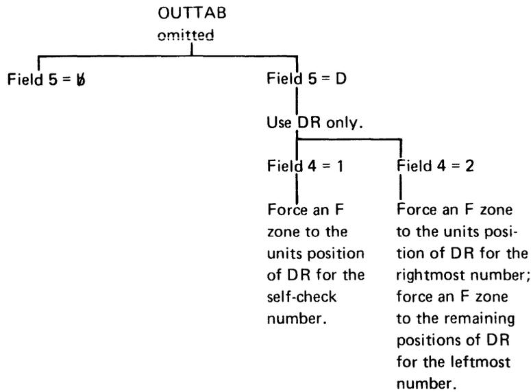
If Field 5 = D, only the DR is used to determine the self-check number output.
