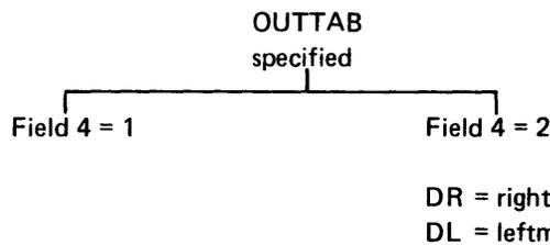
If Field 4 = 2, the value of the DR is used to find the character in the translate table for the rightmost digit, and the value of the DL is used to find the character in the translate table for the leftmost digit.
