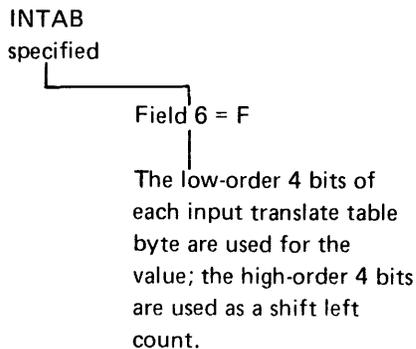
If an input translate table is specified, and field 6 of the CNTL parameter specifies F, the low order 4 bits of each input translate table byte are used for the input value, and the high order 4 bits are used as a shift left count. In the example above, the input translate table byte contained 82; the input value is 2 and the shift left count is 8. The foundation position, and all high order positions are shifted to the left 8 positions.
