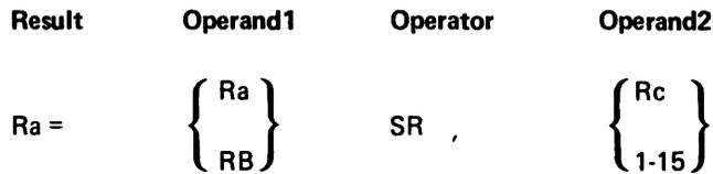
The bytes of the operand1 register are shifted right the number of bytes indicated by operand2, and the shifted result is placed into the result register. The high-order bytes of the shifted result contain blanks (hex 40) for the number of characters shifted. If a negative number is shifted right, the D-zone is shifted out of the register and the register contents are no longer negative.
