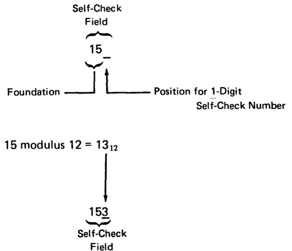
Usually, however, the number converted to the base of the modulus is not the foundation, but a number derived from the individual characters of the foundation. The most common way to derive a number from the characters of the foundation is to:
