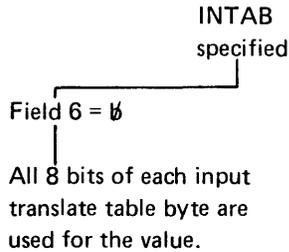
If an input translate table is specified, and if Field 6 of the CNTL parameter is blank, all 8 bits of the input translate table bytes are used for the input value. For example, the letter M is at displacement hex D4; the sample table has the value 82 at displacement hex D4. Therefore, the input value for the letter M is 82.
