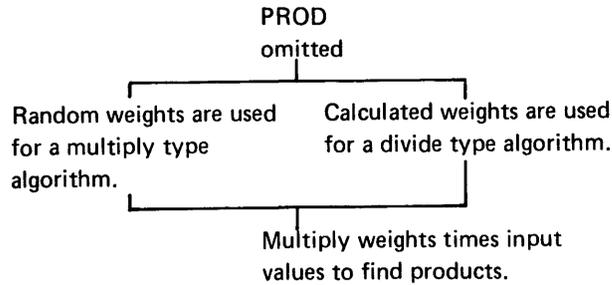
If no product table is specified, products are obtained by multiplying the input value by the corresponding weight. The weights are specified with the WGTS parameter. Enter a hex 00 in each position that corresponds to a self-check digit and to a position that is bypassed. Enter a 1-byte weight for each position that corresponds to a foundation position. The weight must be lower in value than the modulus.
