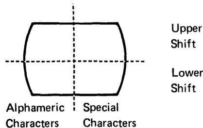
For a special characters shift field, the keyboard is initially positioned in lower shift. If a key is pressed that has both special and alphameric symbols, the lower rightside special symbol is selected unless a shift key is pressed.
