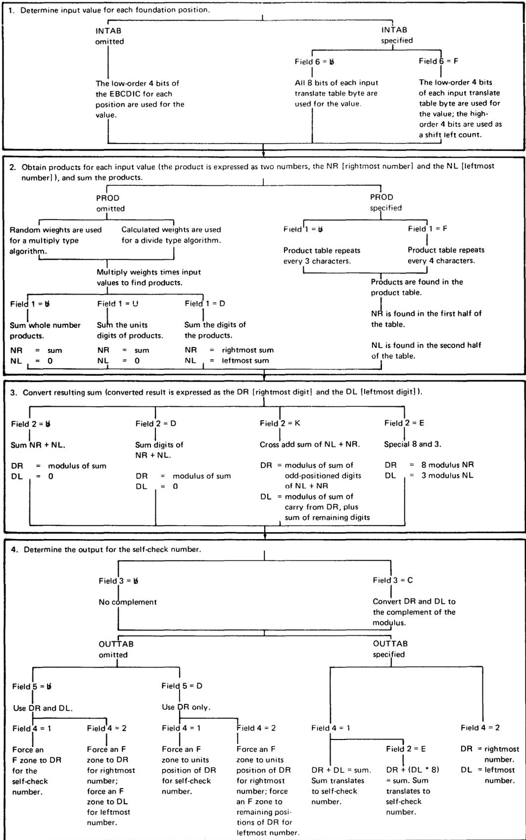
Figure C-1. Self-Check Computations According to .SELFCHK Parameters
