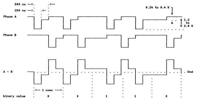
The transmission bit rate on twinaxial cabling is 1 megahertz. With this rate, 1 microsecond is required for each bit and 16 microseconds are required for each frame. 3196 and 3476 display stations use a slightly different frequency: 1.0368 megahertz. None of this section applies to 5520 printer lines.
