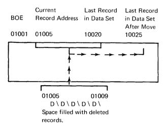
When using the record insert function, there must be enough space between EOD and EOE specified in the data set label. That is, if you want to insert 50 records but only have 40 sectors available (from EOD to EOE) in the data set, an error occurs.
