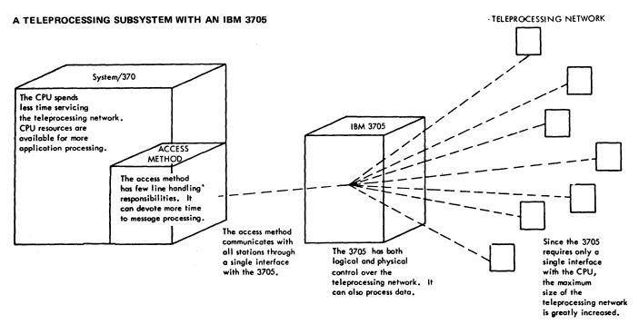
Figure 1.2 Advantages of the IBM 3705 over the IBM 2703
