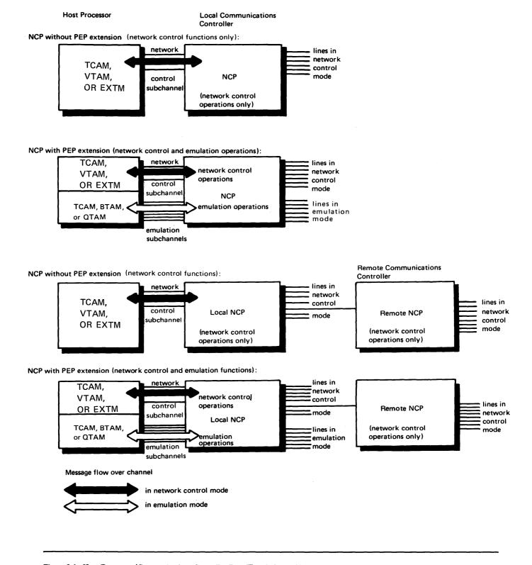
Figure 3.1 Host Processor/Communications Controller Data Flow Relationships
