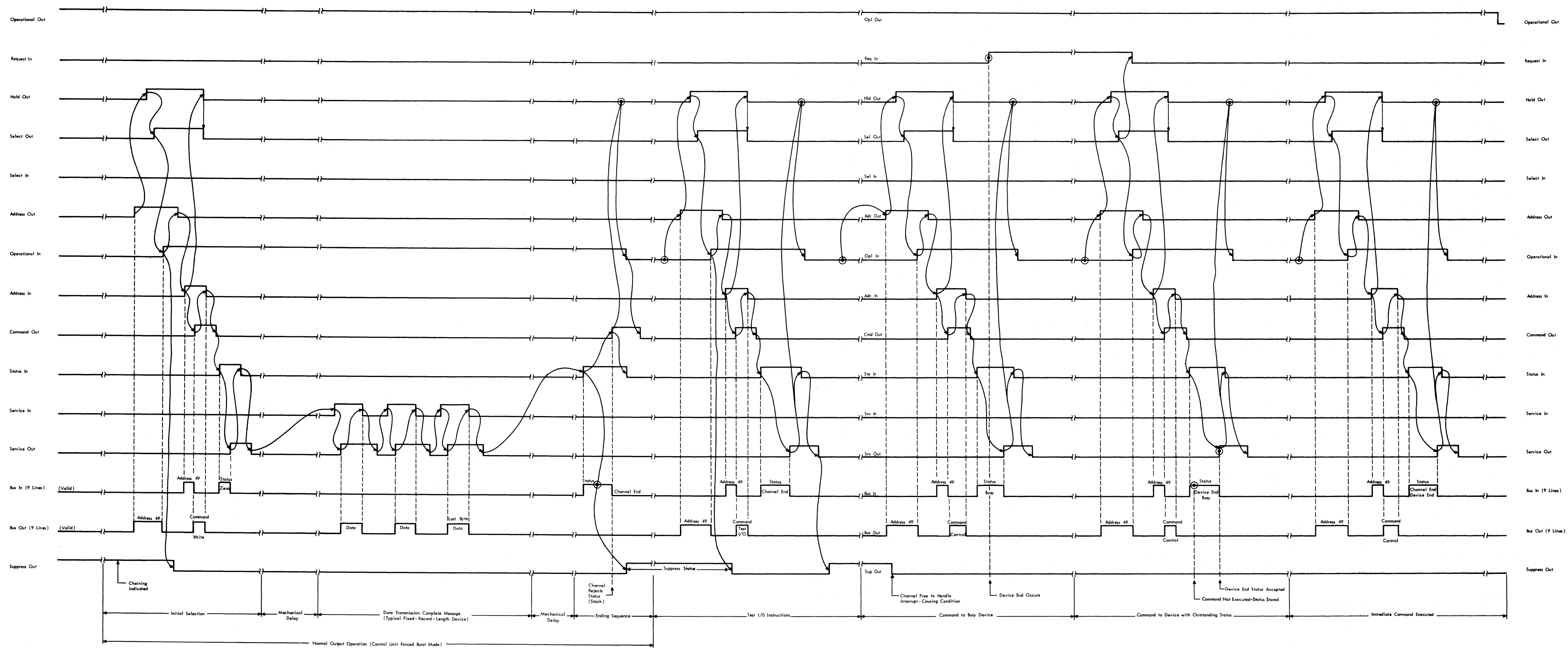
Sequence Chart 2. Control Unit Forced Burst Mode-Multiplexer Channel
