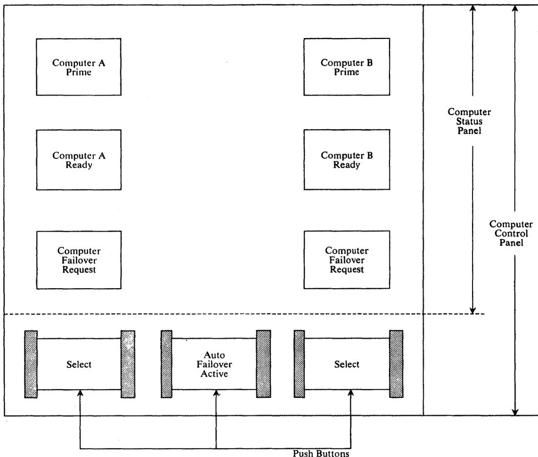
Figure 2-31. Computer Status Panel Indicators and Switches
