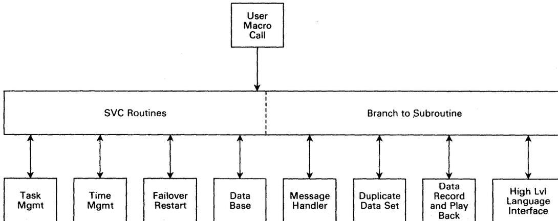
Figure 2-1. The Special Real Time Operating System Overview of the Online System
