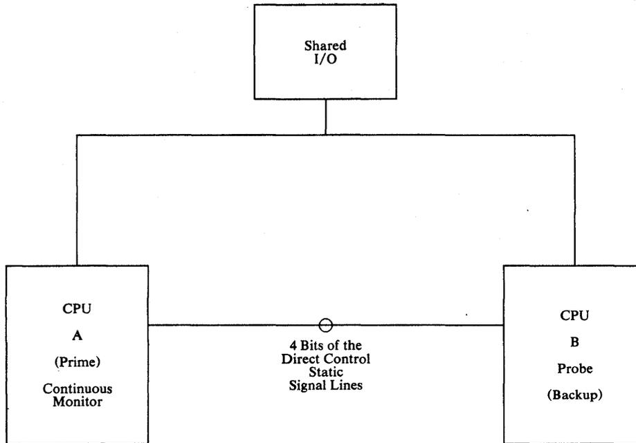
Figure 2-28. Probe Function Failure/Restart Feature
