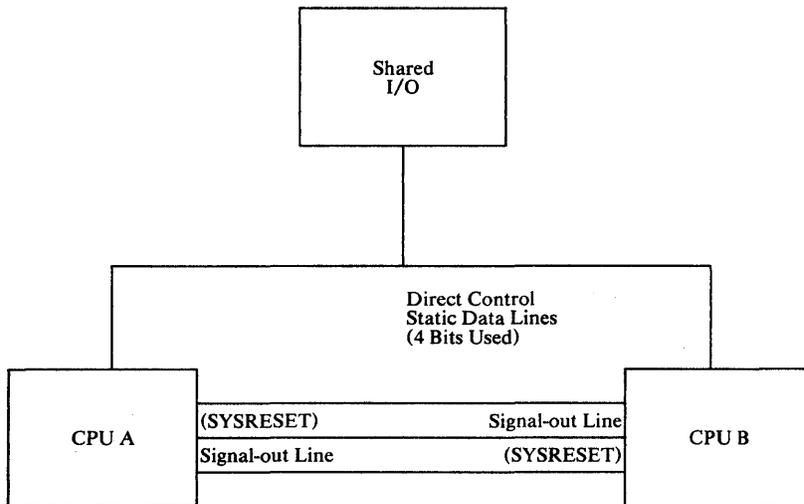
Figure 2-29. Remote System Reset Feature
