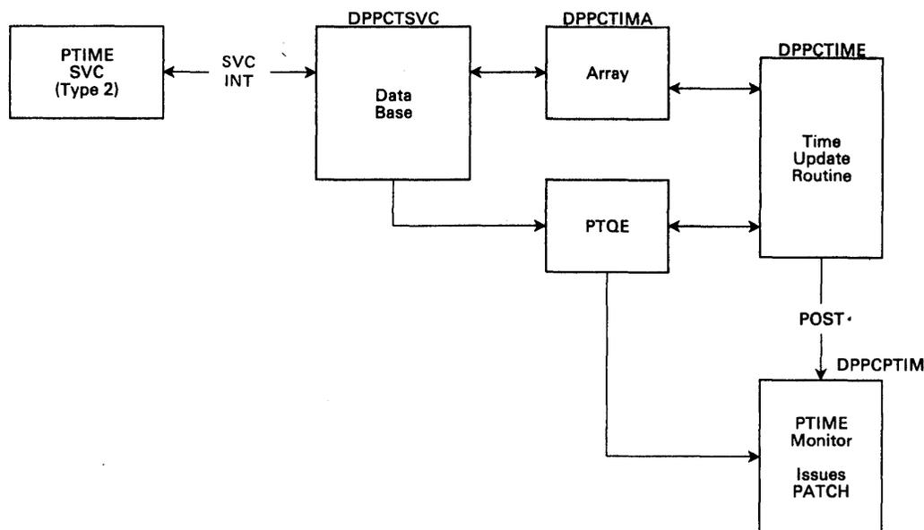
Figure 2-7. PTIME Logic and Control Flow
