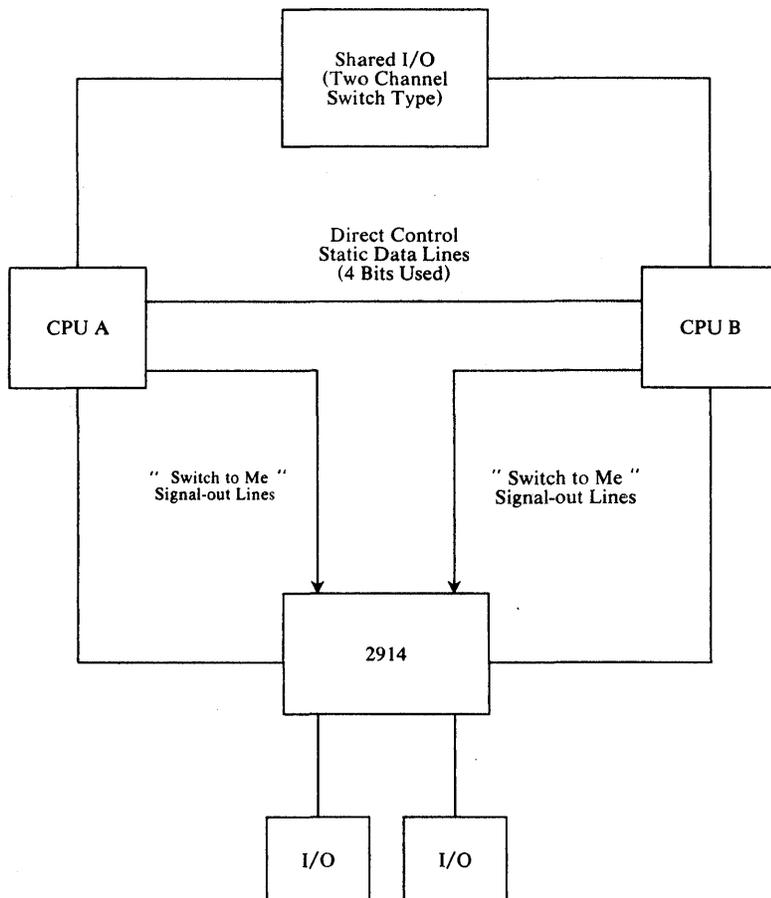
Figure 2-30. System With Automatic 2914 Switch
