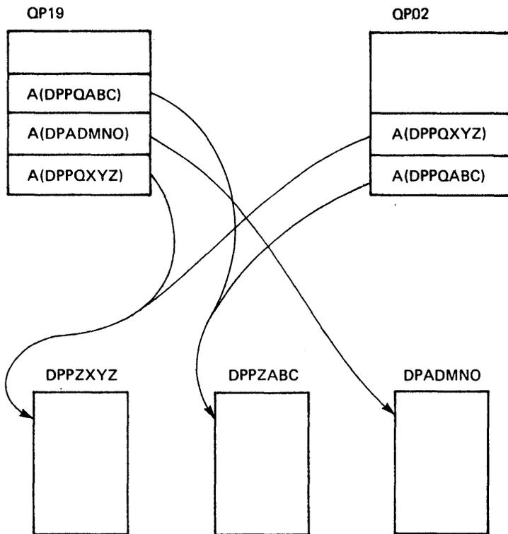
Figure 2-6.2. Queue Processor/Queue Holder Structure
