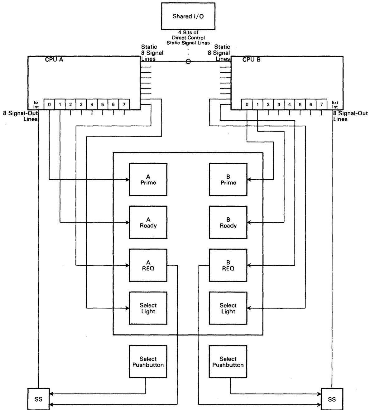
Figure 2-32. Computer Status Panel Connections (Functional)
