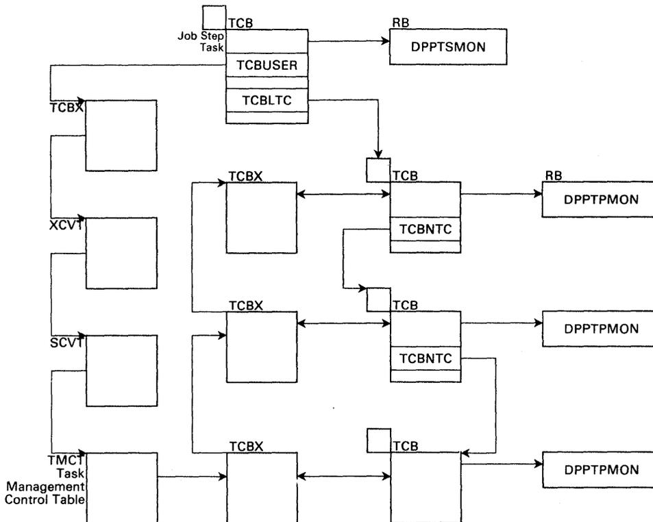
Figure 2-6. Control Blocks After Initialization
