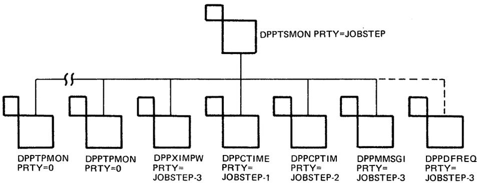
Figure 2-3. The Special Real Time Operating System Task Structure and Priorities
