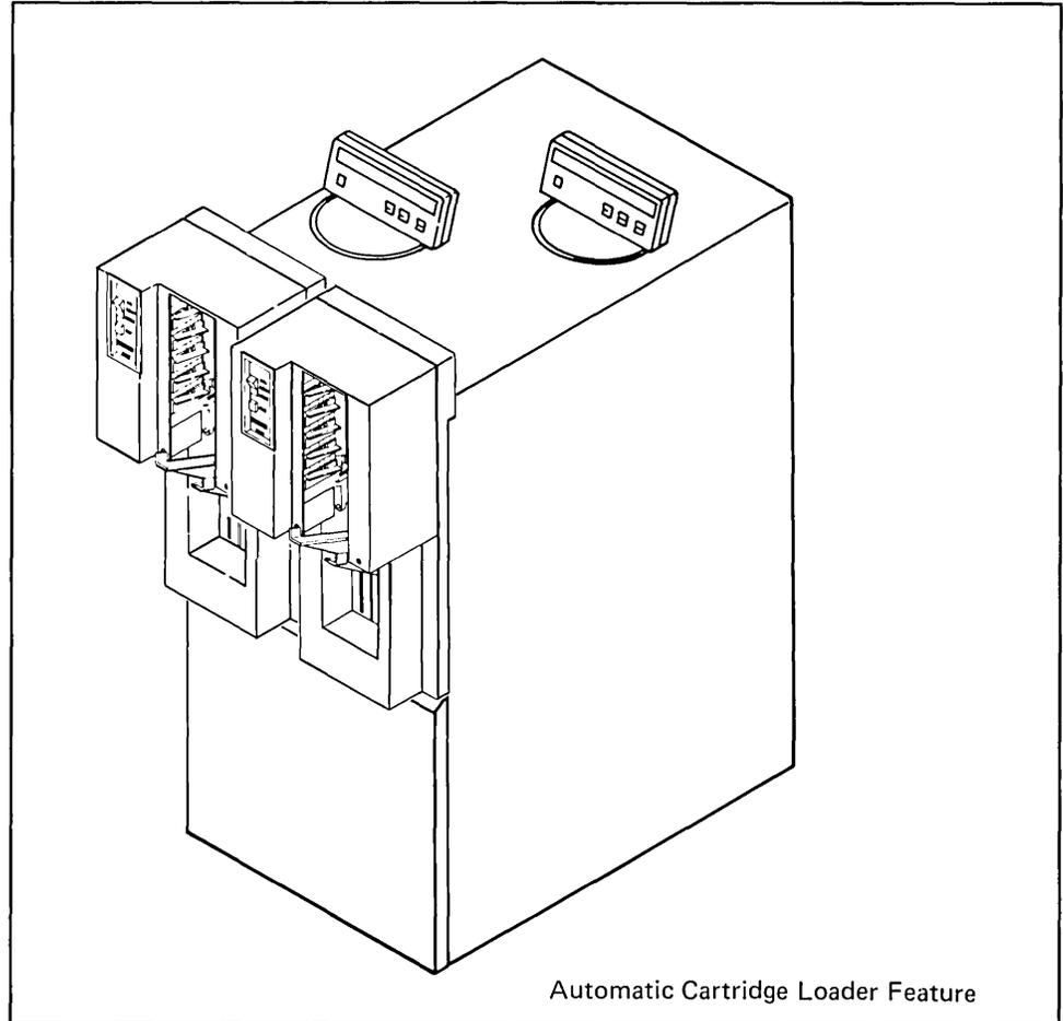
The Loader Operator Panel on the front of the Automatic Cartridge Loader allows the operator to switch between the following modes:
