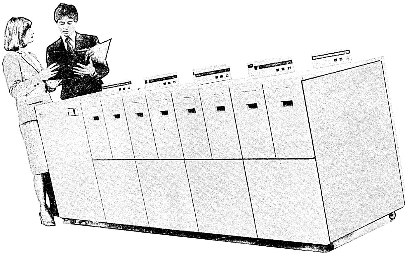
**IBM 3480 Magnetic Tape Subsystem**
