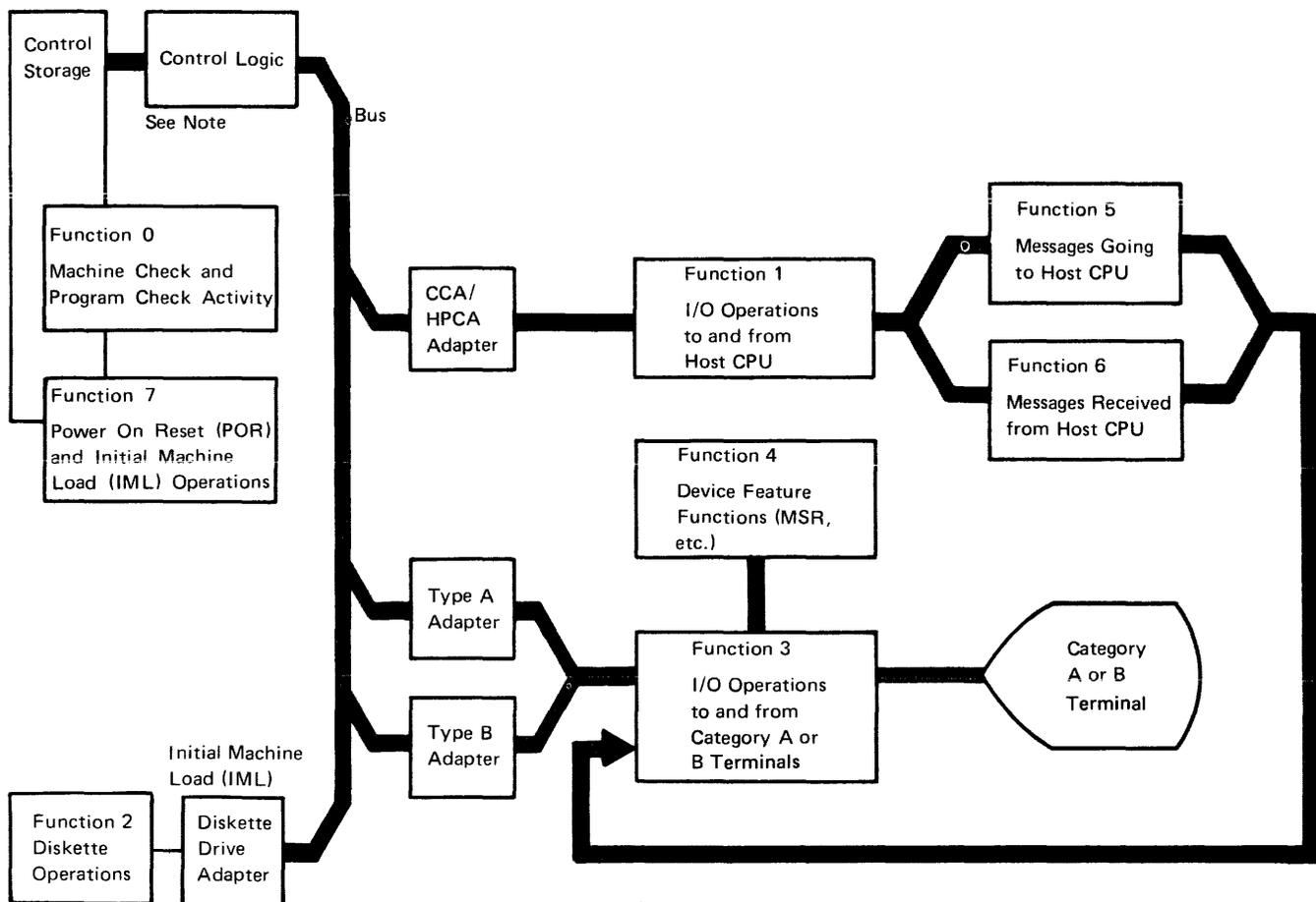
**Note:** The functions shown in this diagram are provided by the control logic.
