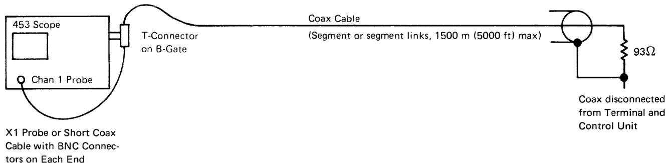
**Figure 4-12. Scope Setup**
