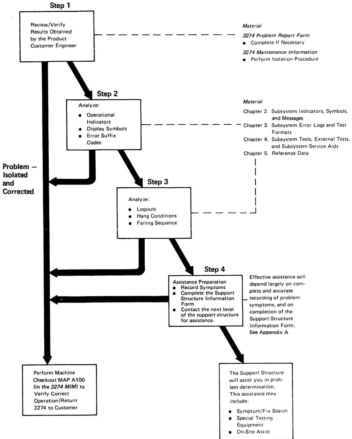
Figure 1-1. Support Customer Engineer Maintenance Approach
