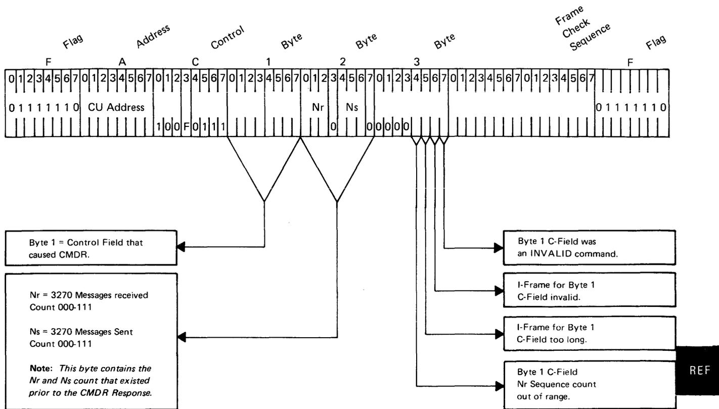
Figure 5-32. Command Reject (CMDR) Message Format
