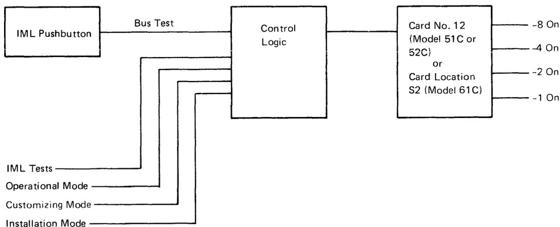
Figure 2-1. 8 4 2 1 Indicator Control Logic
