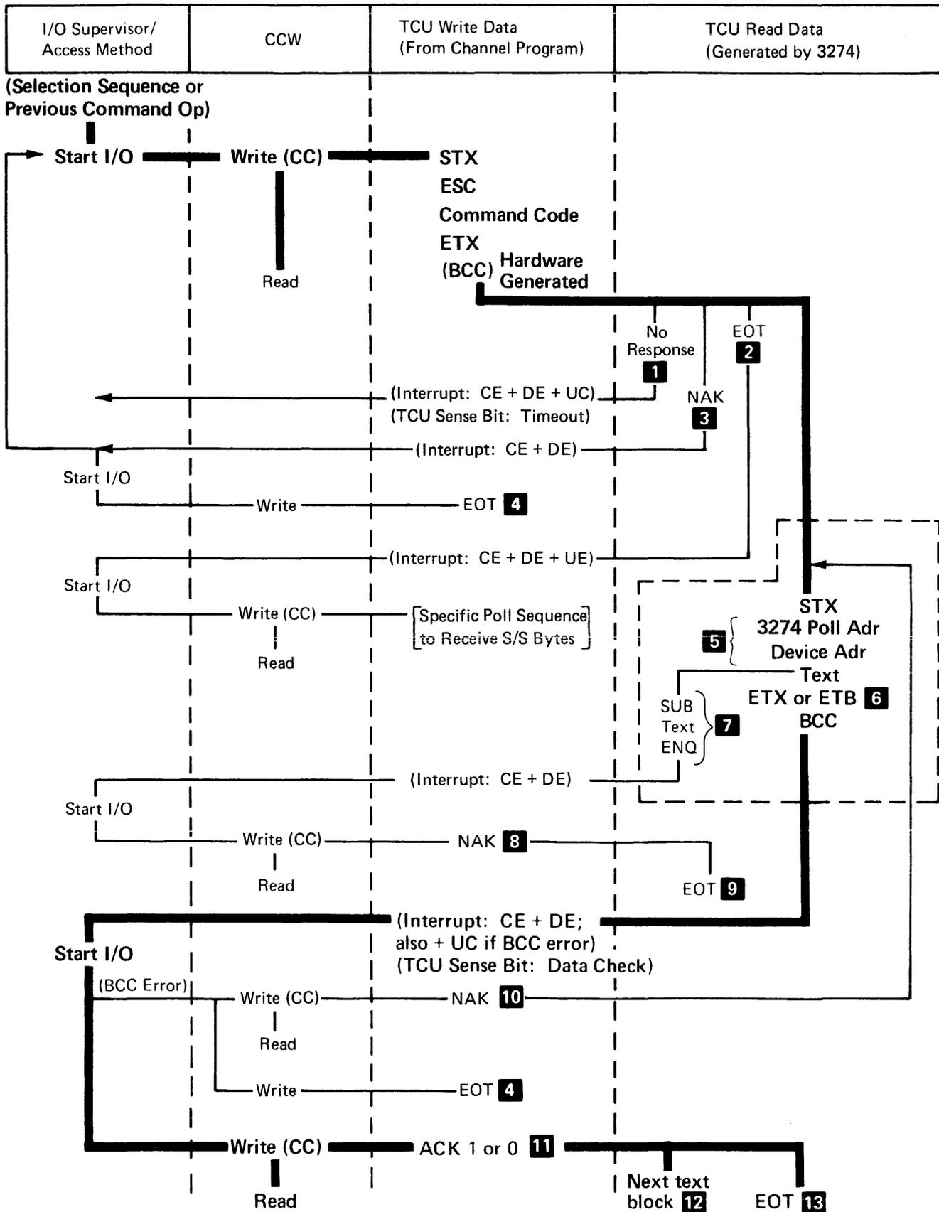
Figure 5-19 (Part 1 of 2). Read-Type Command, Sequence/Response Diagram
