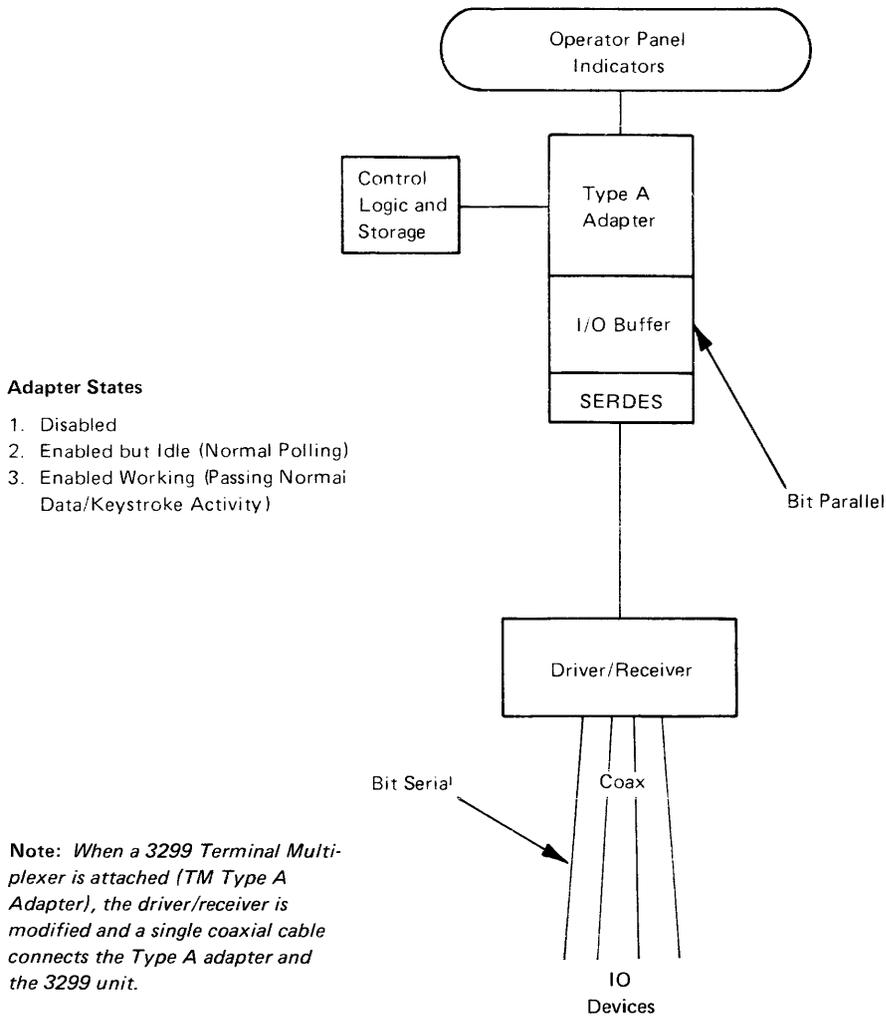
Figure 1-12. Coax to Type A Adapter Data Flow
