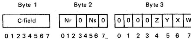
Byte 1 is the C-field that caused the CMDR response. Byte 2 contains the Ns and Nr sequence counts that existed immediately prior to establishing the CMDR response. Byte 3 indicates the reason for the CMDR.
