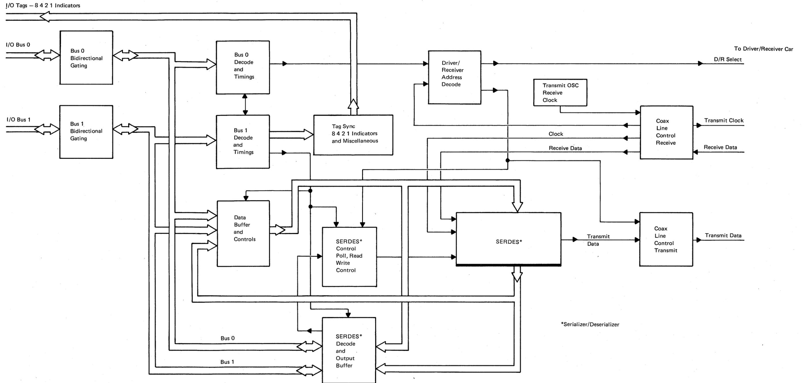
Figure 1-8. Keystroke Handling, Type A Adapter (without 3299)
