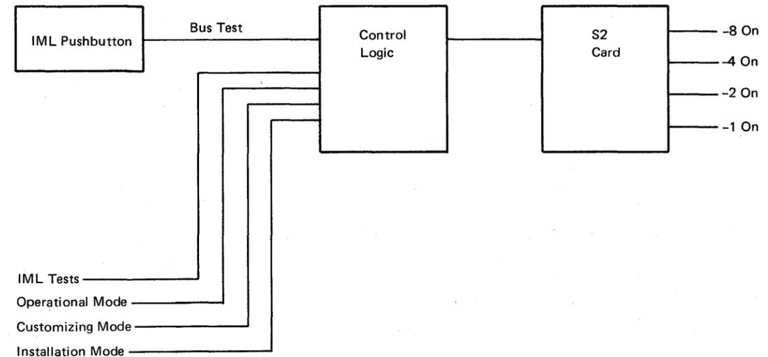
Figure 2-1. 8 4 2 1 Indicator Control Logic
