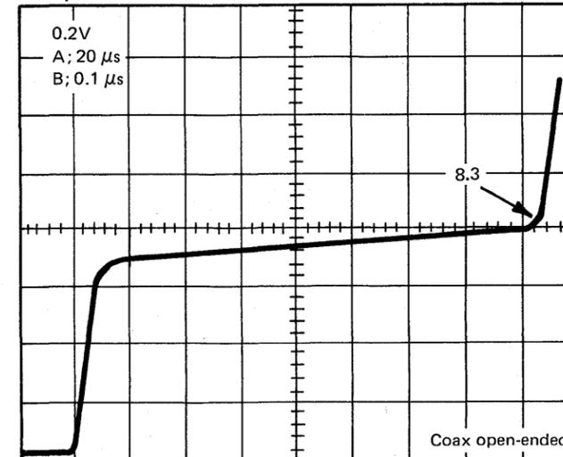
101 m (332 ft) of good coax cable, 8.3 divisions long. (This is an effective method to measure the length of the cable.)
