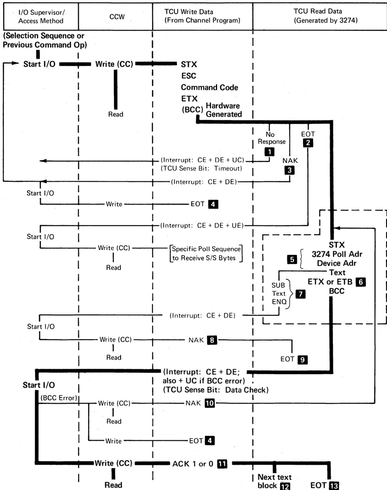
Figure 5-33. Read-Type Command, Sequence/Response Diagram
