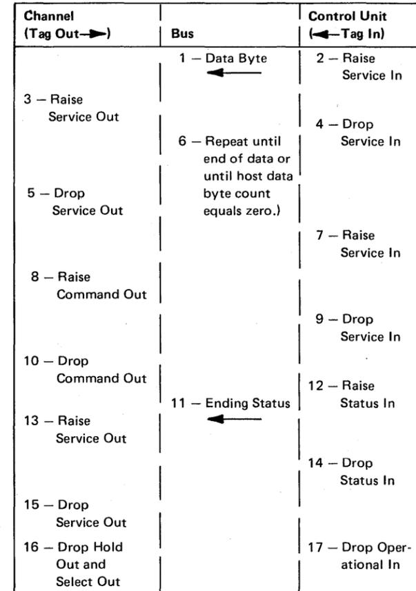
Figure 5-22. Read—After Selection with Read Command
