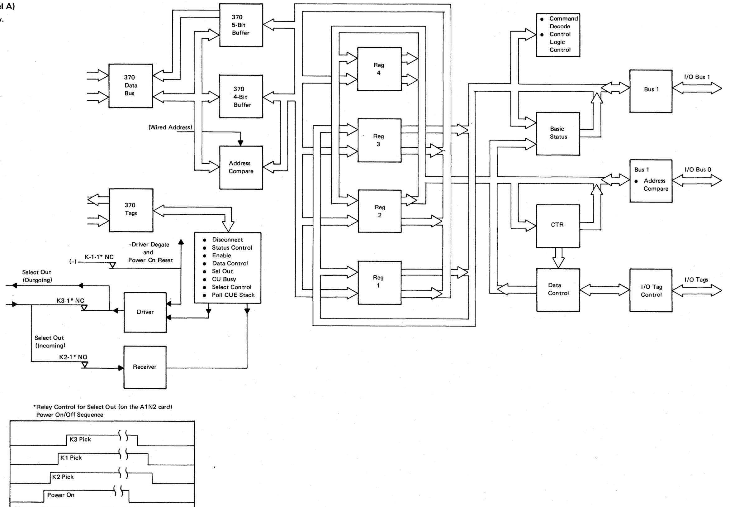
Figure 1-12. Local Channel Attachment Data Flow
