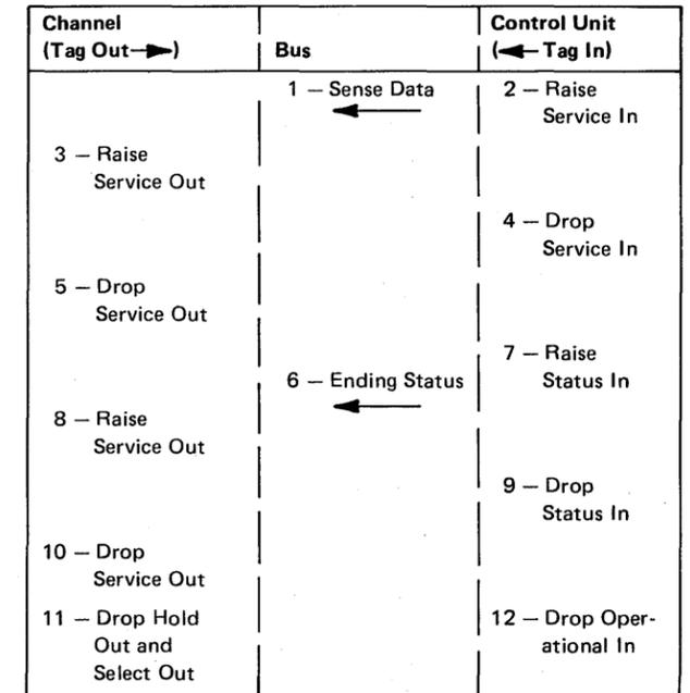
Figure 5-23. Sense—After Selection with Sense Command (Issued in Response to Unit Check Status)
