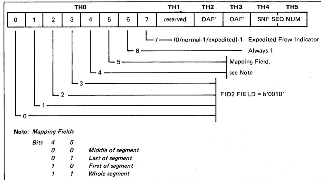
Figure 5-49. Transmission Header Format
