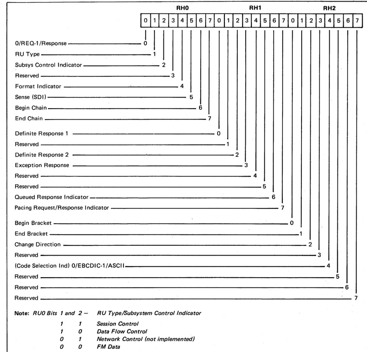
Figure 5-50. Request/Response Header Format
