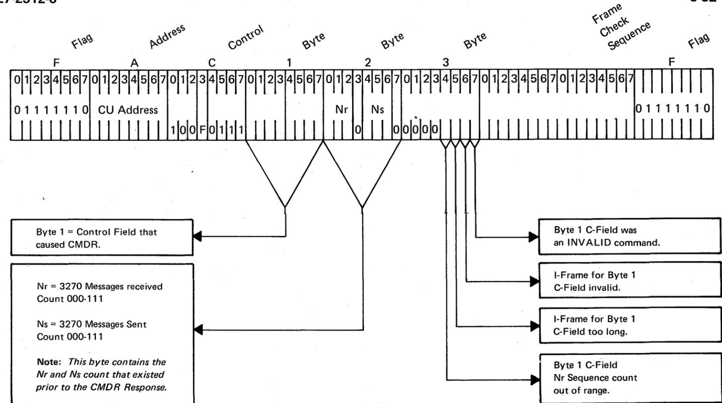
Figure 5-54. Command Reject (CMDR) Message Format
