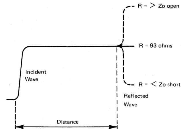
Figure 4-19. Incident and Reflected Waves
