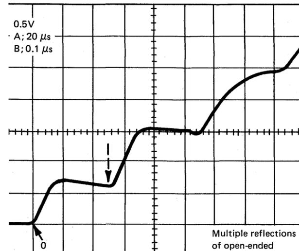
Improper setup of scope.
