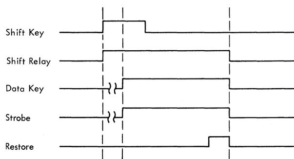
Figure 2-21. Keyboard Data Transfer Timing
