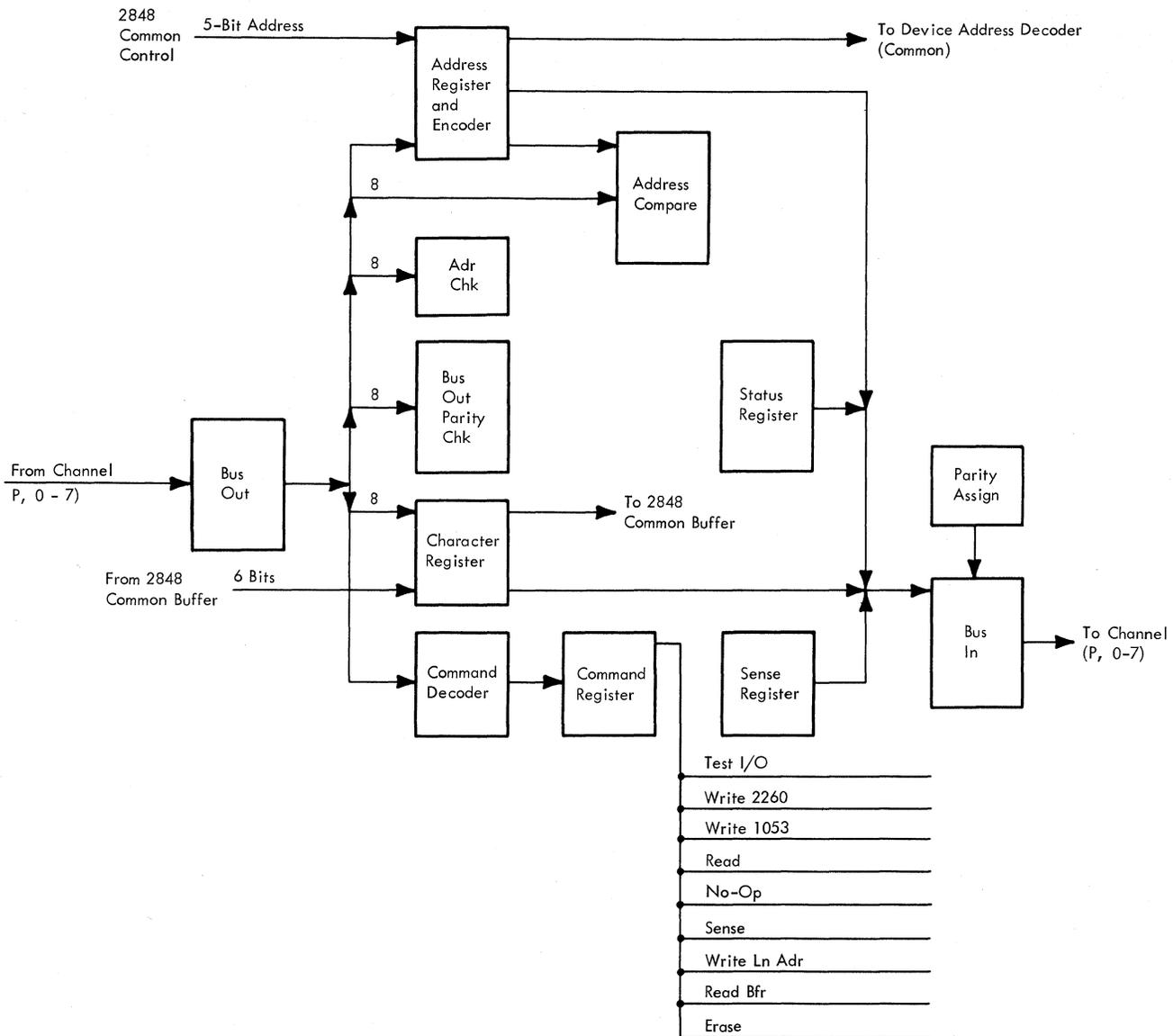
Figure 2-89. Channel Interface Controls
