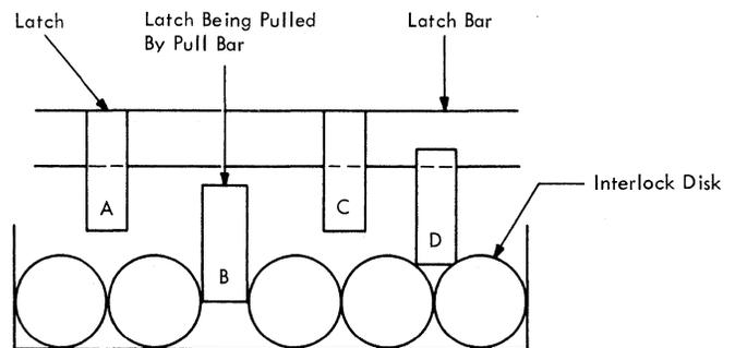
Figure 2-19. Interlock Disks (Partial)
