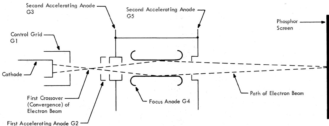
Figure 2-4. CRT Electron Gun
