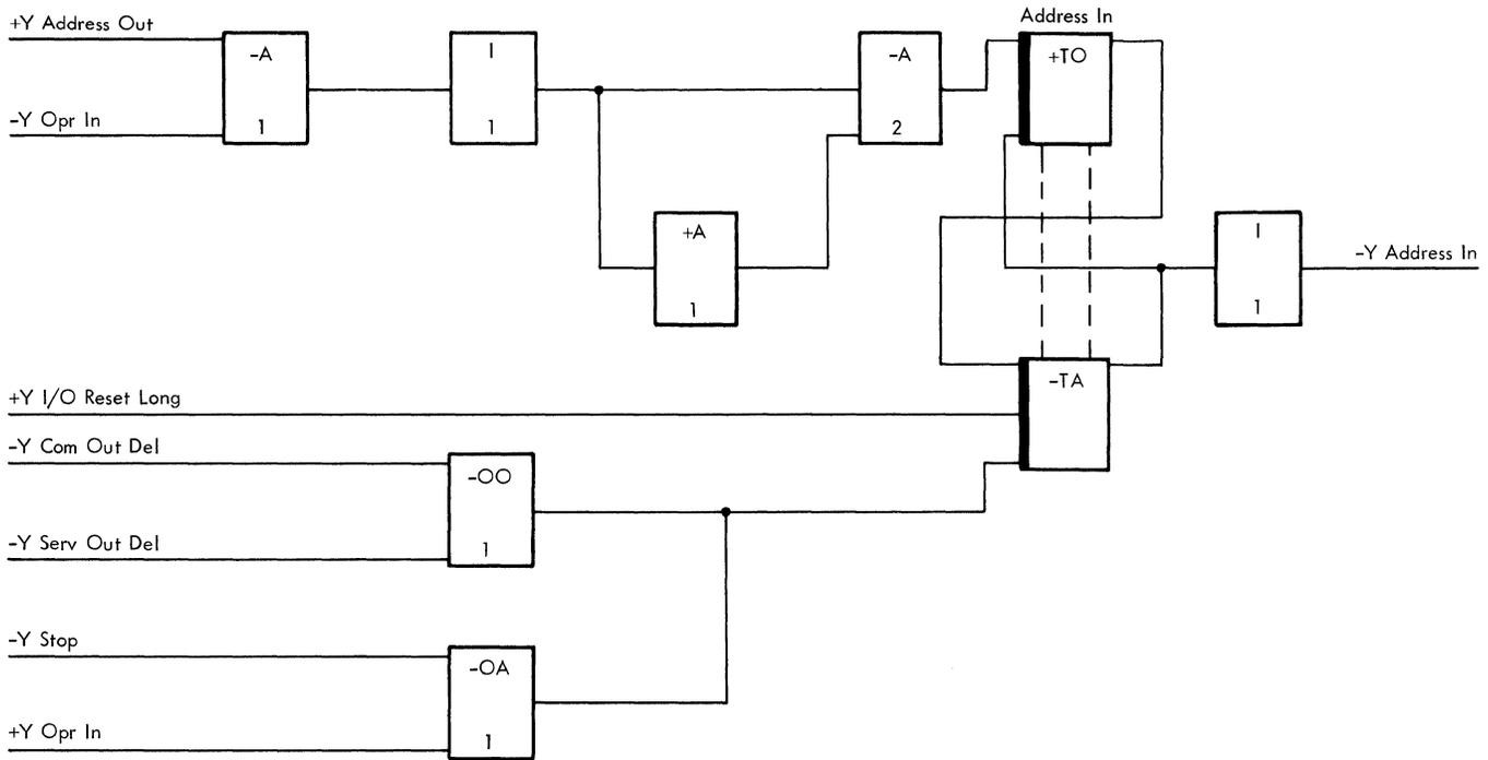
Figure 2-91. Address In Latch
