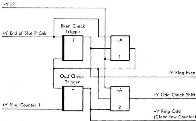
Figure 2-37. Buffer Parity Control Circuit
