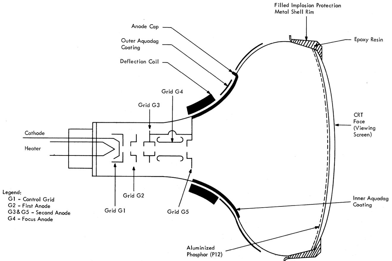
Figure 2-3. Cathode-Ray Tube
