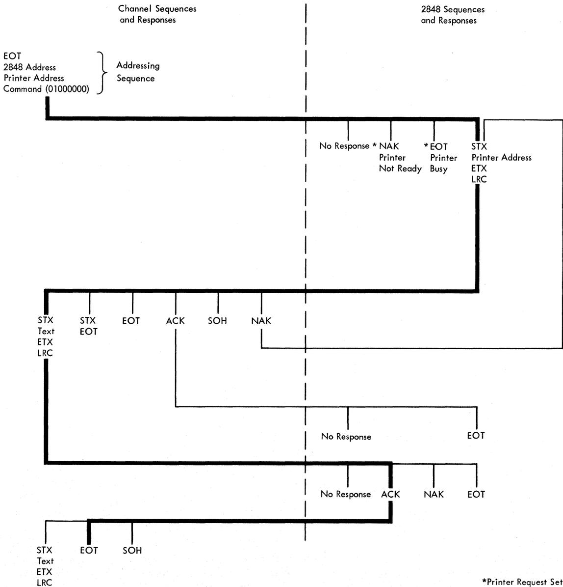
Figure 4-7. Sequence/Response Diagram - Specific Poll to Printer
