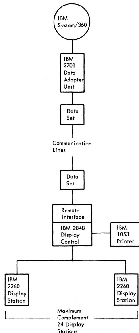
Figure 4-1. Remote Display Complex Configuration
