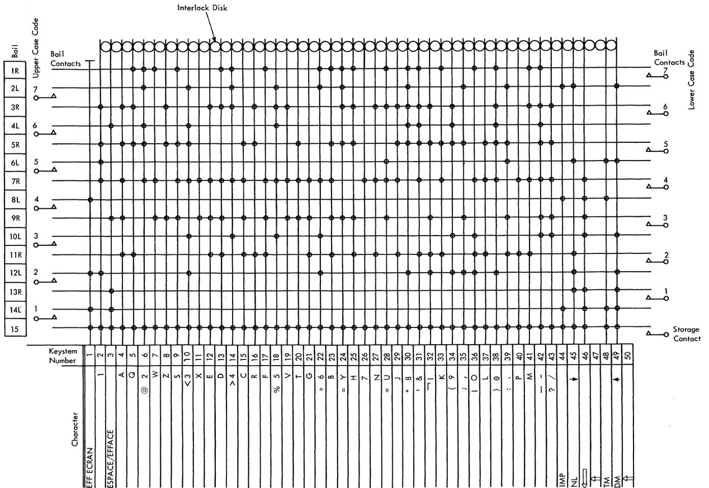
Figure C-7. Keystem Number and Bail Selection, French Alphanumeric Keyboard
