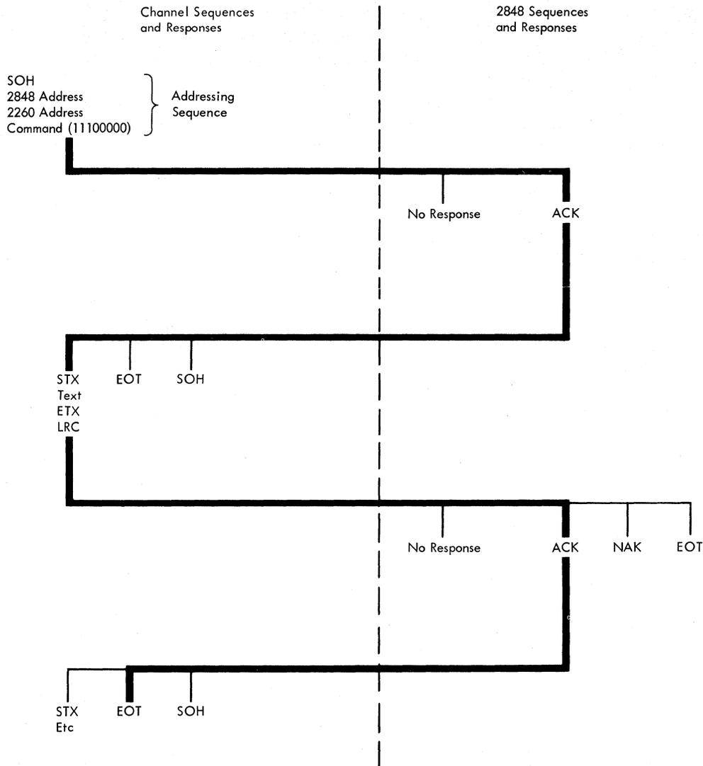
Figure 4-11. Sequence/Response Diagram - Erase/Write
