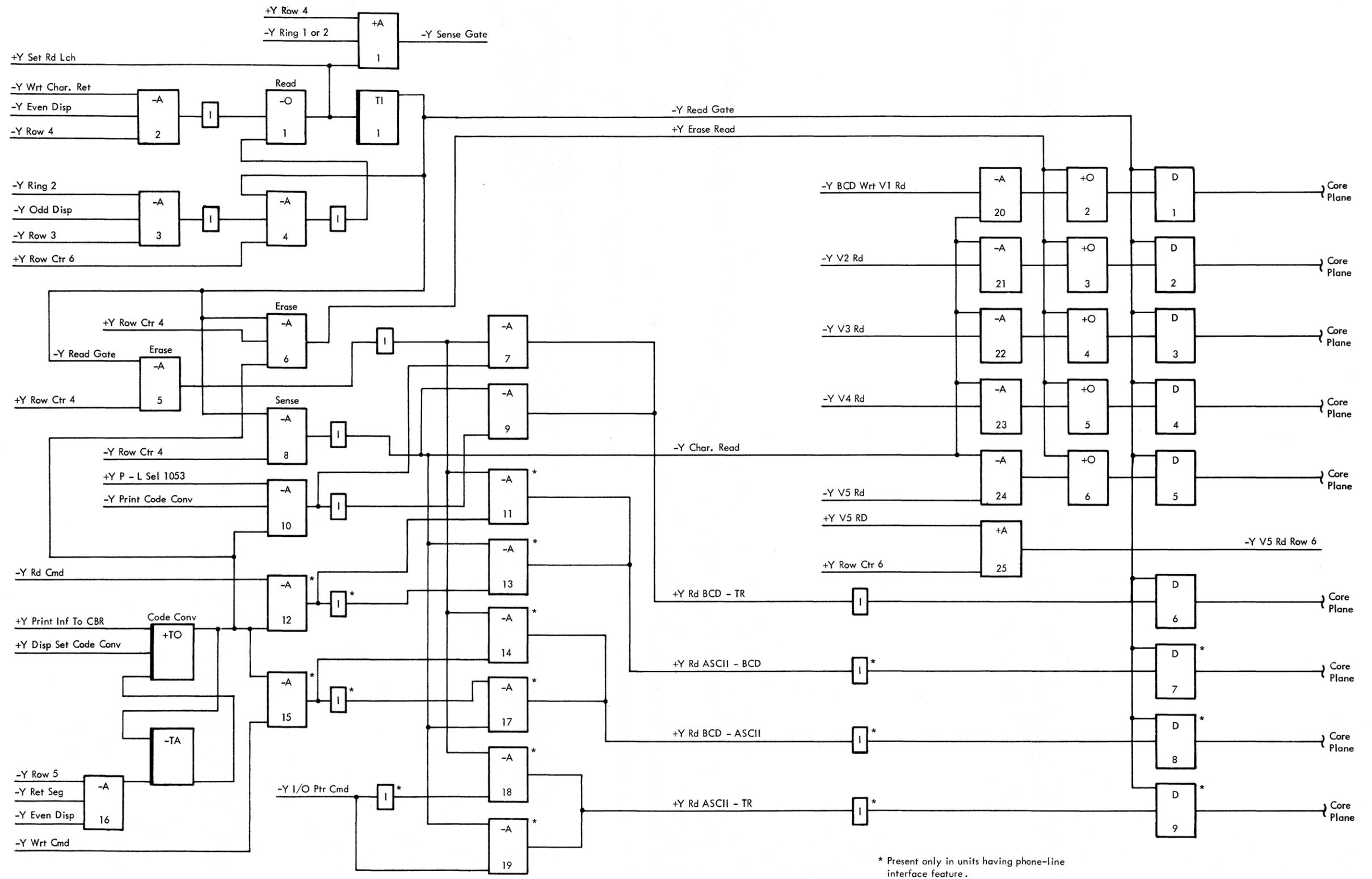
Figure 2-71. Character Generator Read Control Circuits
