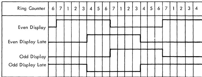
Figure 2-36. Even-Odd Display Trigger Circuit
