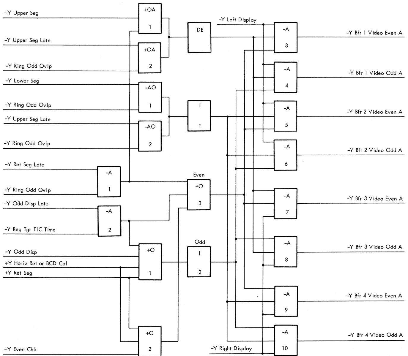
Figure 2-79. Video Buffer Selection, A Delay
