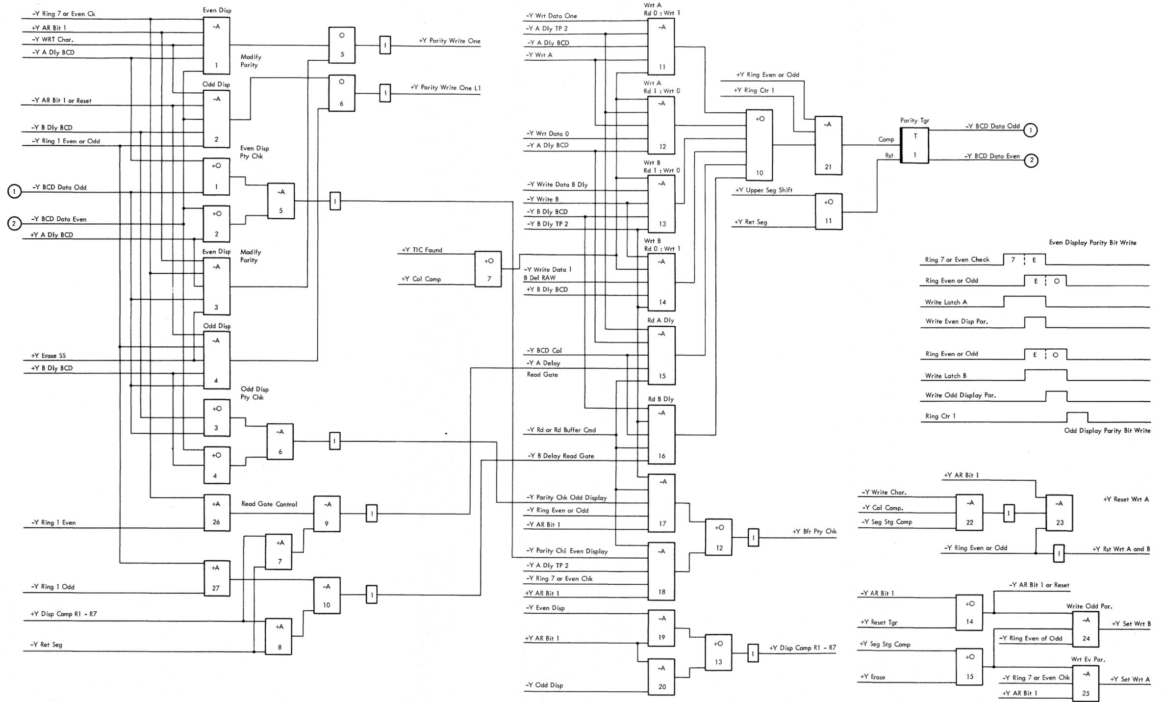
Figure 2-86. Parity Circuits
