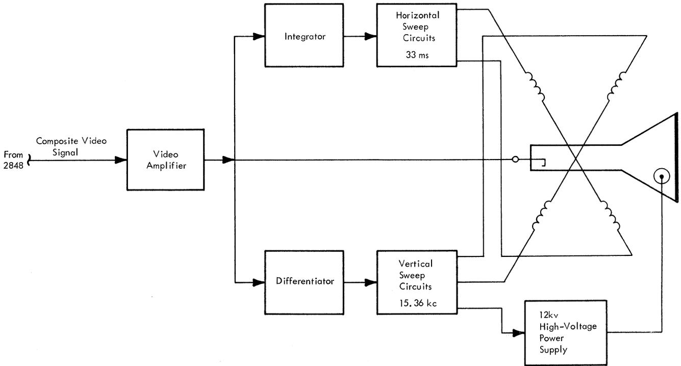
Figure 1-9. 2260 Display Station, Block Diagram
