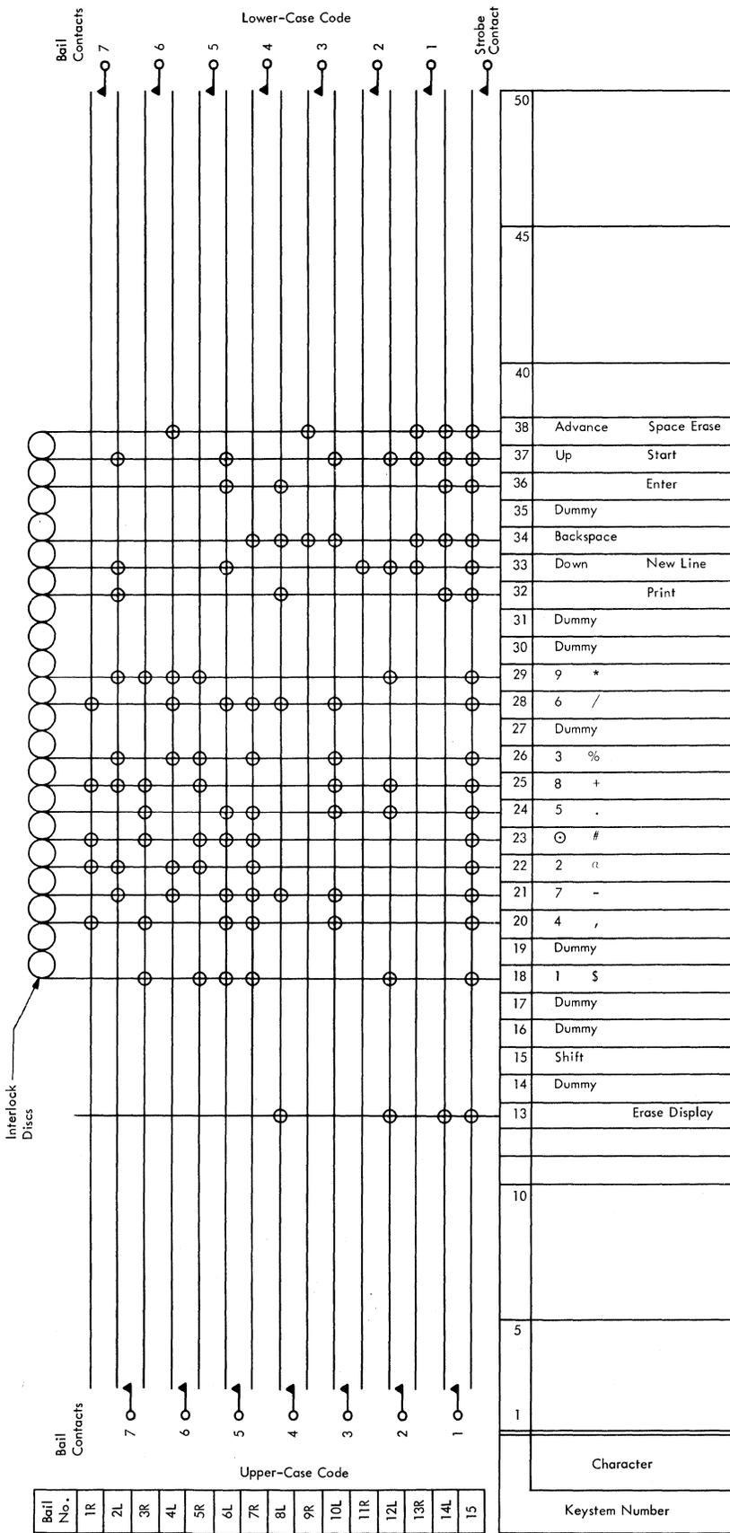
Figure 2-16. Keystem Number and Bail Selection For Numeric Keyboard
