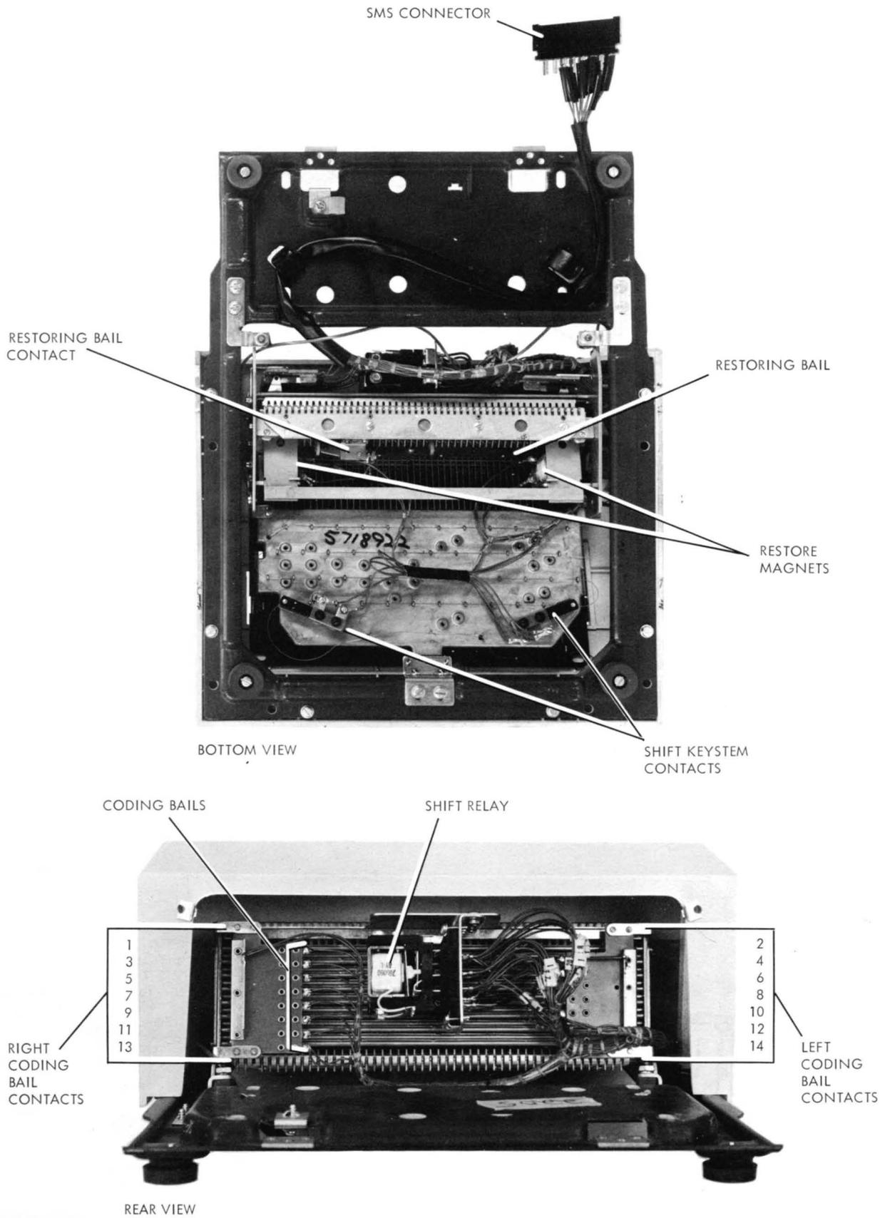
Figure 2-10. Alphanumeric Keyboard, Bottom and Rear Views
