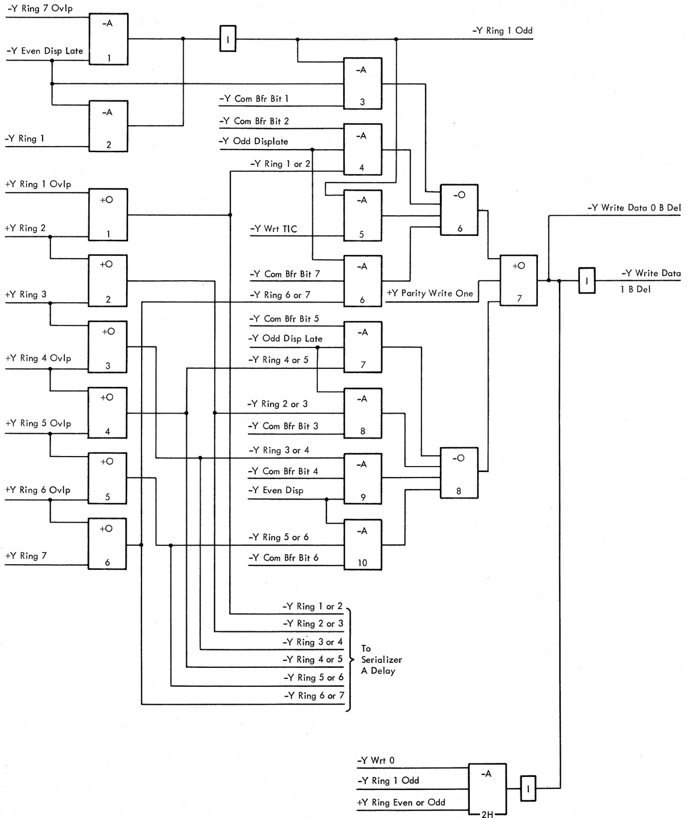
Figure 2-56. Serializer, B Delay
