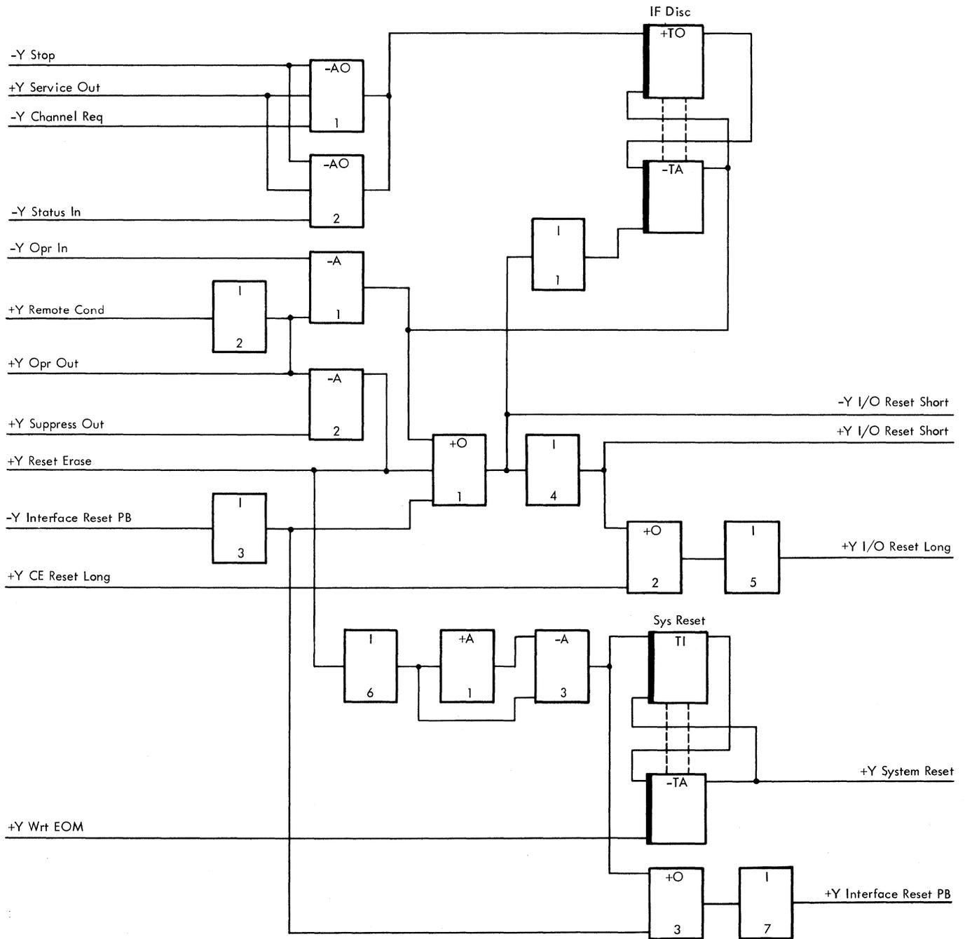
Figure 2-95. Disconnect and Reset
