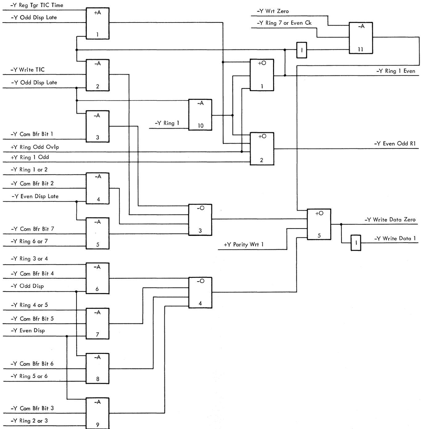
Figure 2-55. Serializer, A Delay
