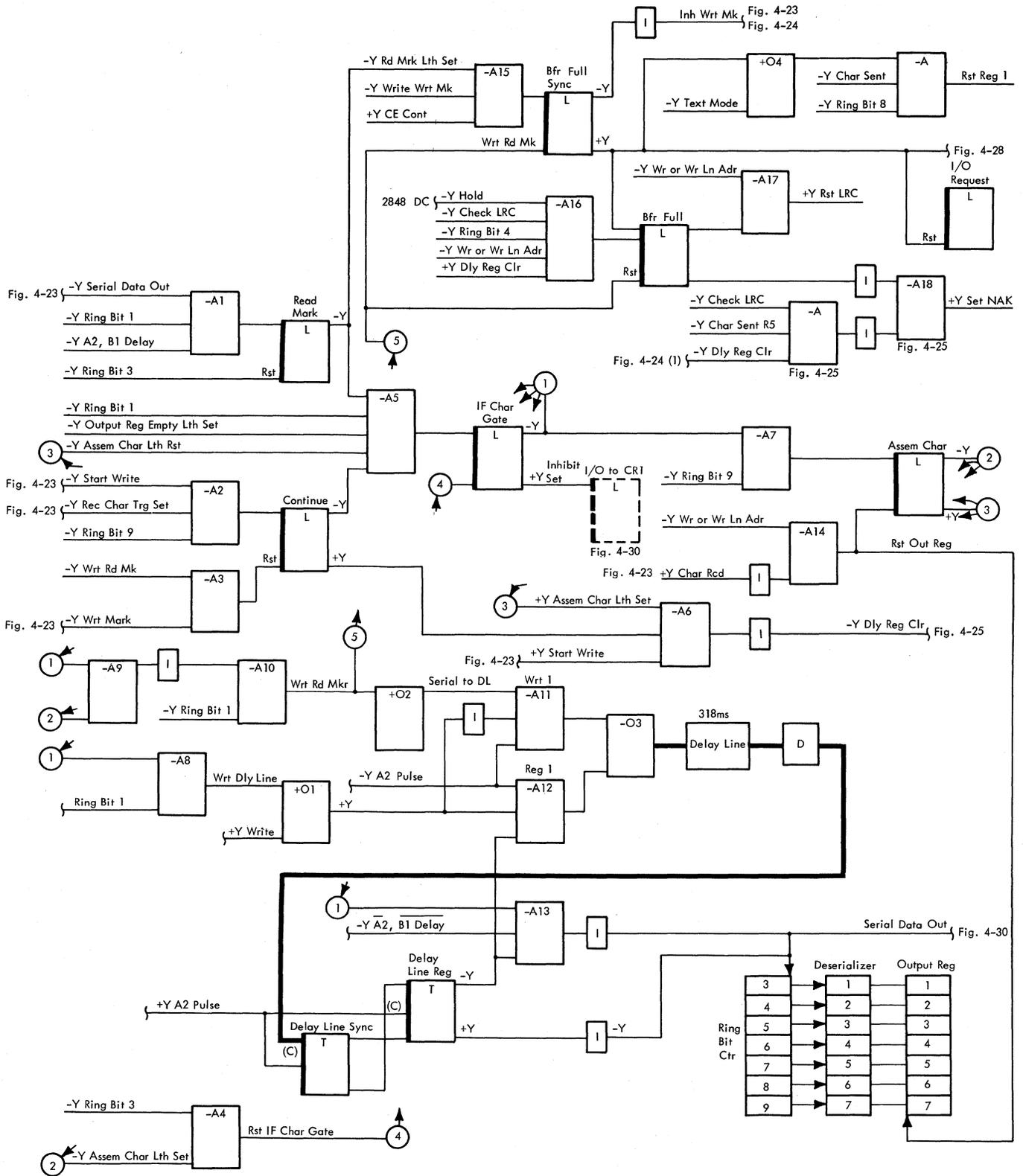
Figure 4-24. Delay Line Readout Control
