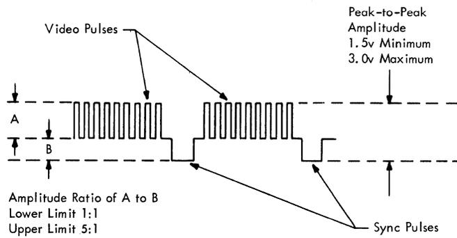
●Figure 2-2. Composite Video Signal (One Vertical Scan)
