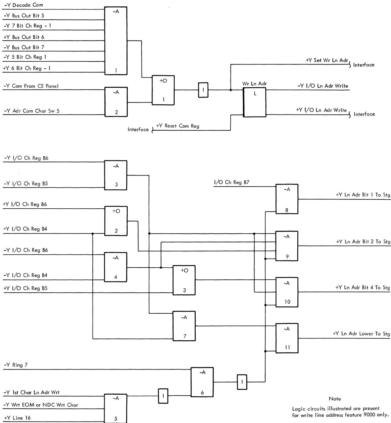
Figure 2-83. Write DS Line Address Decode and Gating
