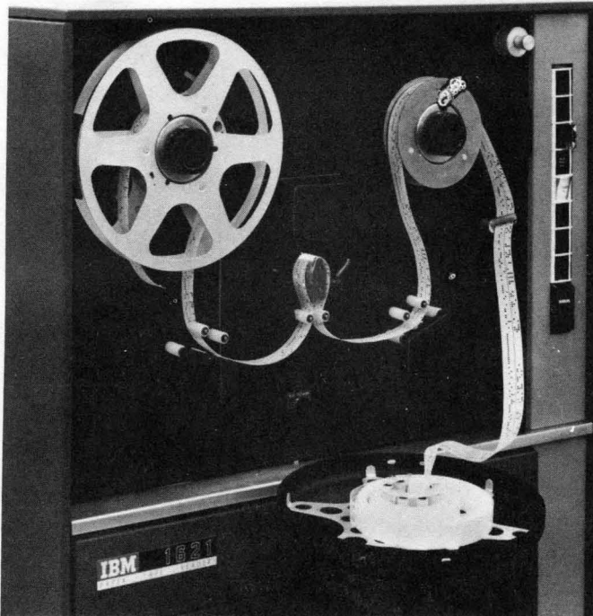
Fig. AV.2. Threading Tape from Center Roll Feed.
