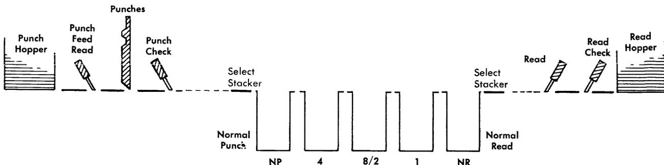
Figure 31. Punch-Feed-Read Schematic
