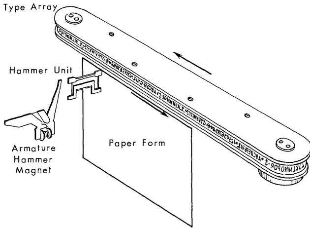
Figure 17. Schematic of Printing Mechanism
