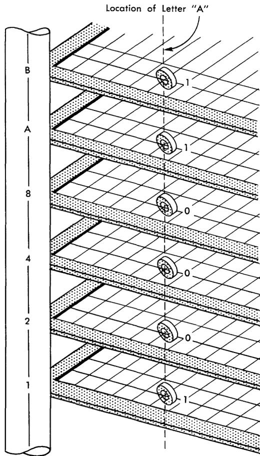
Figure 4. The Letter A Represented in Magnetic-Core Storage
