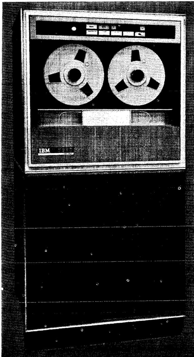
Figure 24. IBM 7330 Magnetic Tape Unit
