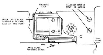
Figure 3-2. Chute Blade and Select Magnet Adjustments
