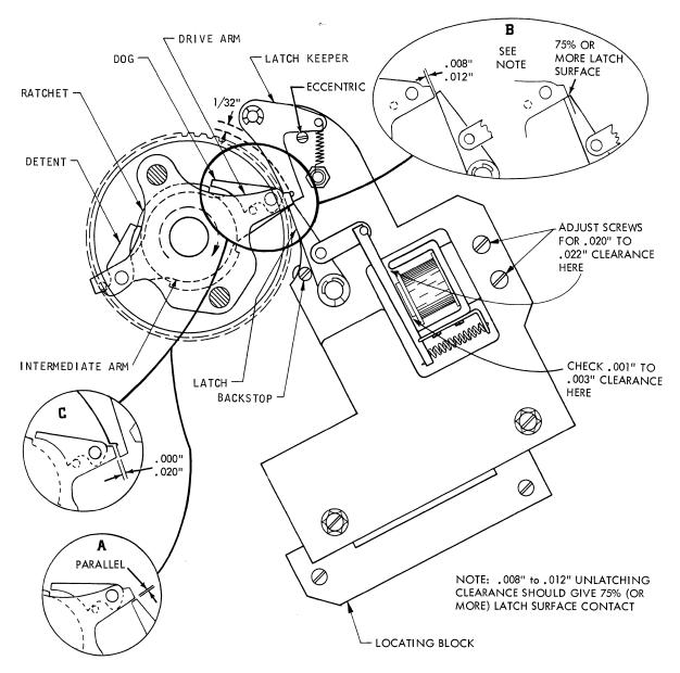
Figure 2-4. Magnet Assembly Adjustments
