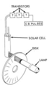
Figure 6-2. Solar Cell Schematic
