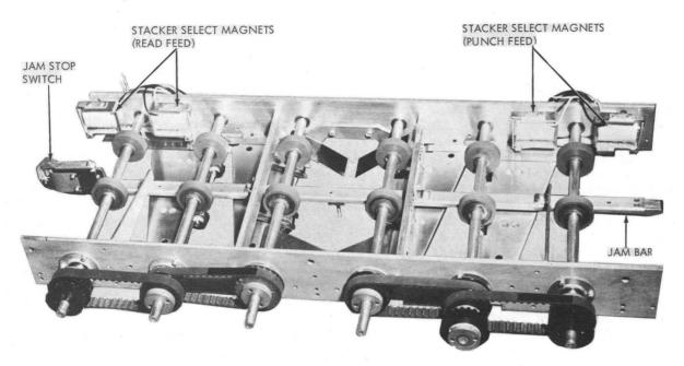
Figure 1-2. Transport Mechanism
