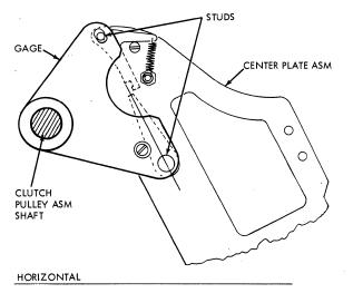
Figure 2-5. Latch Assembly Plate Alignment
