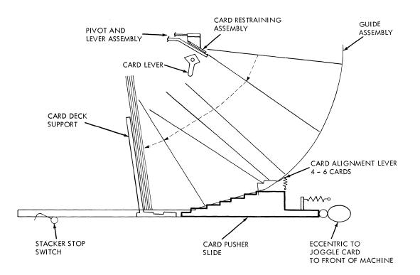
Figure 3-5. Stacker Schematic
