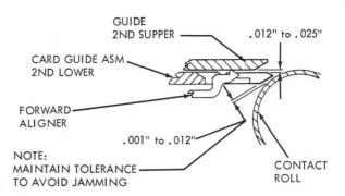
Figure 8-5. Punch Feed Read Card Guide Adjustments and shift the card guide to obtain clearance.
