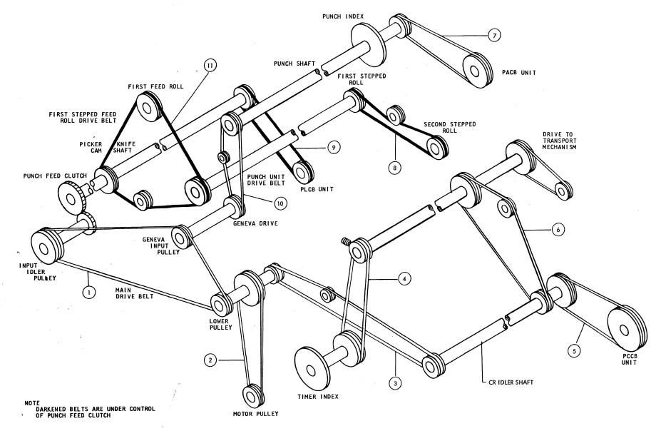
Figure 5-2. Punch Feed Timing Belts
