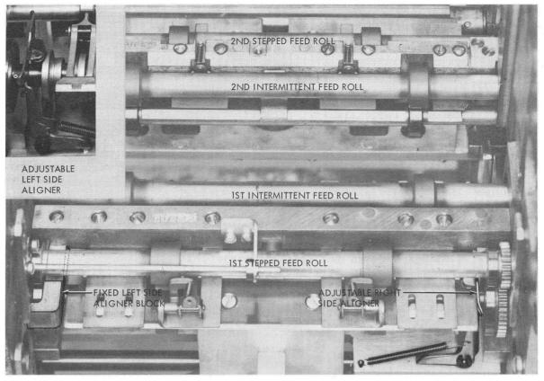
Figure 4-5. Feed Rolls and Aligner Stations
