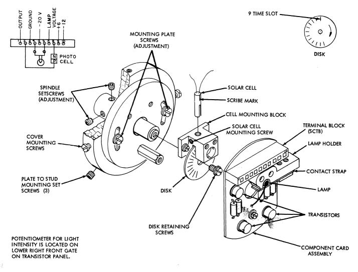
Figure 6-3. Solar Cell Lamp
