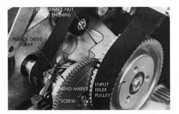
Figure 5-4. First Stepped Feed Roll Timing Belt Installation
