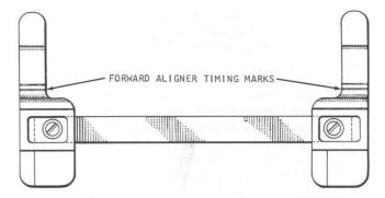
Figure 4-7. Gage 608183 Timing Mark
