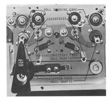
Figure 4-8. Roll Opening Device
