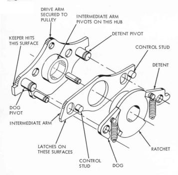
Figure 2-3. Clutch Assembly
