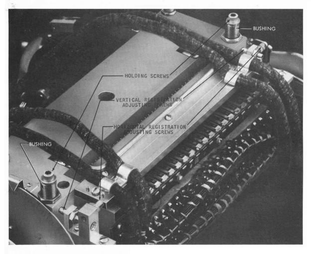
Figure 4-17. Punch Unit Adjusting Screws
