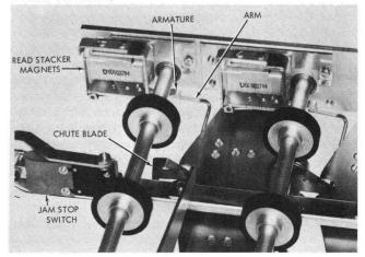
Figure 8-1. 51-80 Column Transport Selectors
