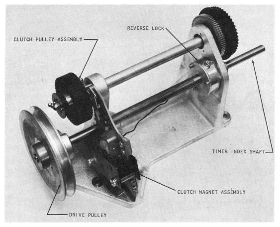
Figure 2-6. Clutch Drive Assembly
