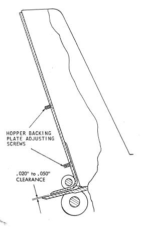
Figure 2-12. Hopper Back Plate Clearance
