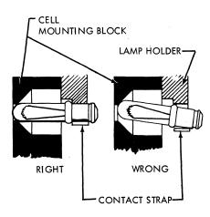
Figure 6-4. Solar Cell Adjustments
