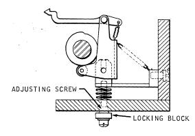
Figure 4-9. Forward Aligner Adjustments
