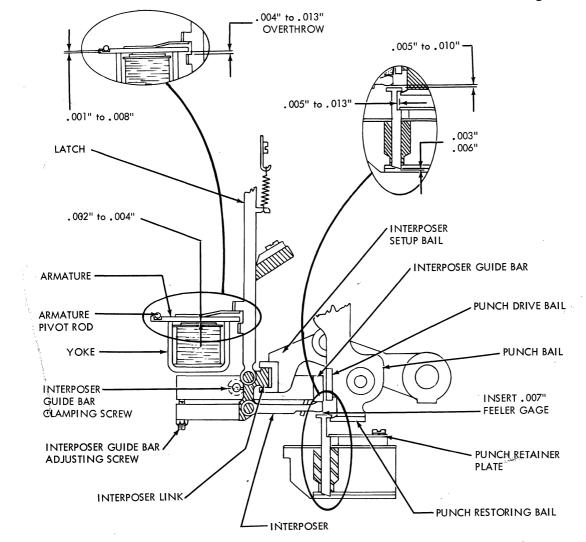
Figure 4-15. Punch Unit Adjustments
