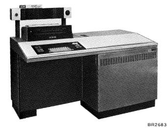
Figure 1. IBM 1131 Central Processing Unit (Models 1A, 1B, 2A, 2B, 4A, and 4B)
