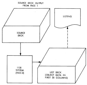
Figure 3. Card Assembler, Pass 2
