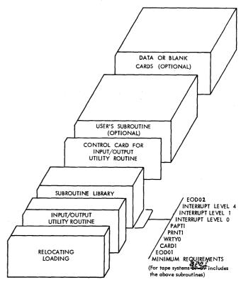
Stacked Input Arrangement for Utility Input/Output Operations
