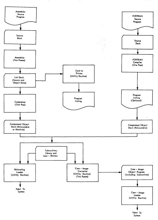
Figure 1. Typical Card Processing System
