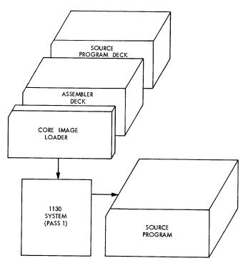
Figure 2. Card Assembler, Pass 1
