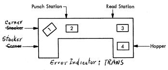
Operator procedure: When program halts, empty hopper, clear 1442 card path, place cards 2 and 3 in hopper before card 4, and ready the 1442.
