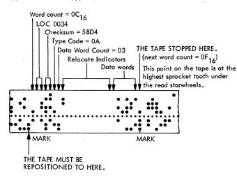
Step 15 of the procedure displays the word count in the SBR. In this case it is 670°C. Convert the two right characters to decimal:  $0^{\circ}_{16} = 12^{\circ}_{10}$ , multiply this number by 2 and add 2, as indicated in step 16.
