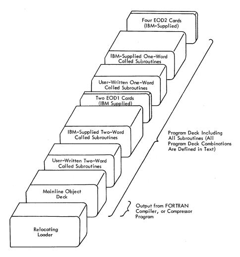
Figure 10. Stacked Input to Load a Relocatable Program
